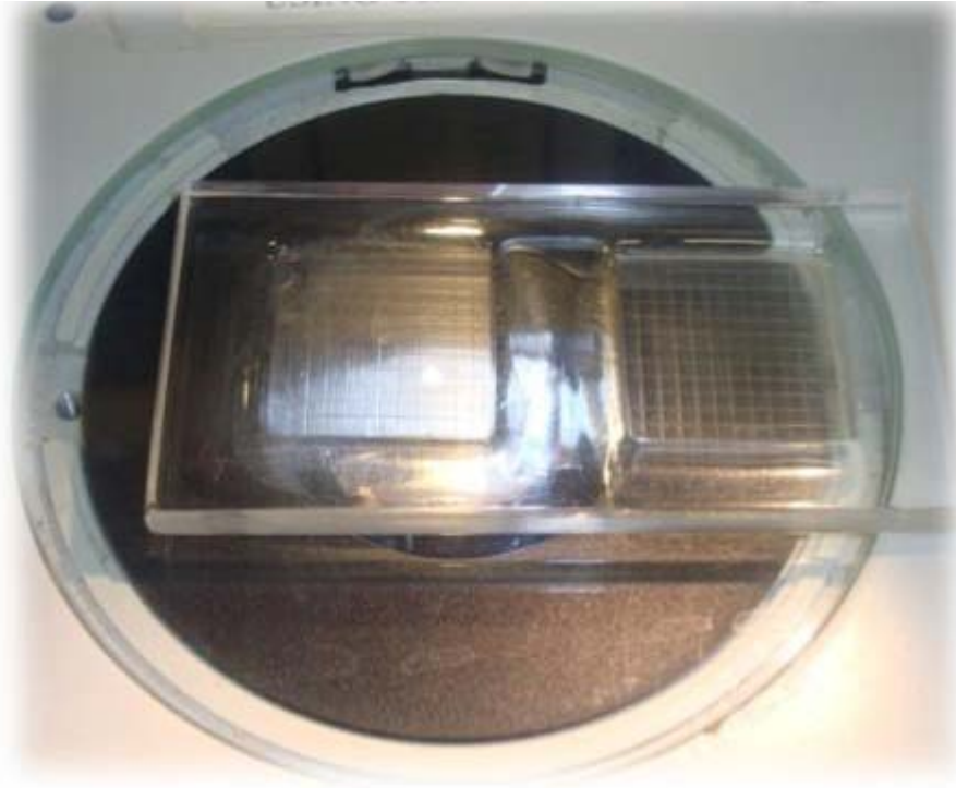
Figure 7. Nematode counting chamber used to determine IJ concentration. Each cell holds 1 ml of IJ suspension.
