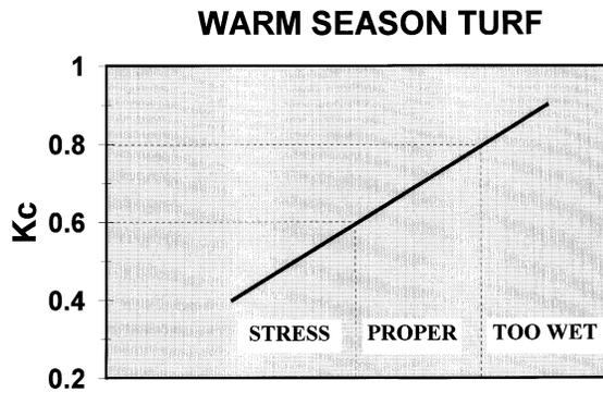
Figure 2. The appropriate  $K_c$  range for warm season grass is 0.6-0.8. Use of a  $K_c$  below 0.6 will likely produce water stress; use of  $K_c$ s above 0.8 will likely produce wet and/or muddy conditions.
