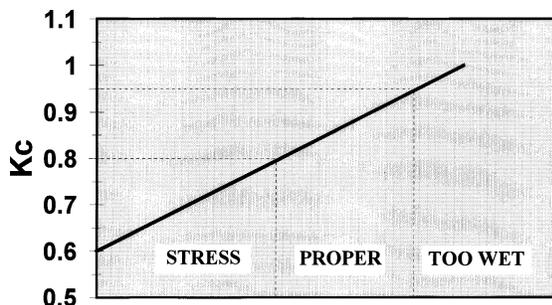
Figure 3. The  $K_c$  range for cool season grasses (e.g. fescue) during summer is 0.80-0.95. Use higher  $K_c$ s for high quality turf and turfs with less heat tolerance. Lower  $K_c$ s suffice for lower quality turf or for more heat tolerant varieties.
