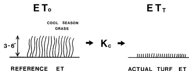
Figure 1. Reference Evapotranspiration ( $ET_0$ ) must be adjusted with a crop coefficient ( $K_c$ ) to estimate turf ET ( $ET_T$ ).
