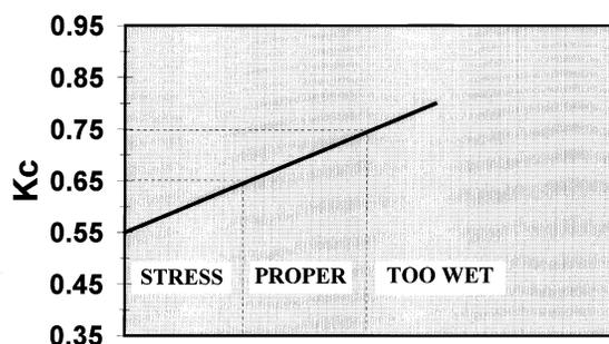
Figure 4. The  $K_c$  range for overseeded perennial rye is 0.65-0.75. Higher  $K_c$ s are required for high quality turf and warm weather. Lower  $K_c$ s suffice for cooler weather and lower quality turf.
