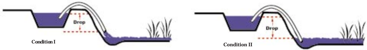
Figure 5. Diagrams where to measure the drop distance for siphon tubes. (Diagram by J.S. Jones, 2003).
