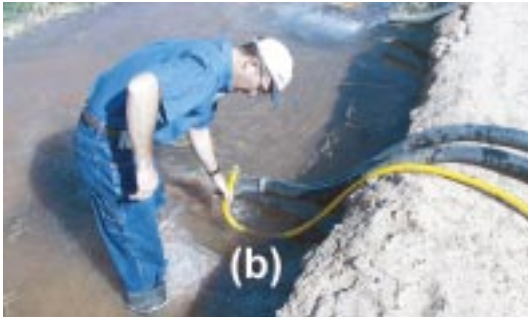
Figure 6. Three photos demonstrating how to measure the “drop” in a surface system. The drop is the distance from the level of the water in the ditch to the water level in the field. (a) Use the hose to siphon water out of the ditch; (b) Raise the hose up until water stops flowing out of the hose end; (c) Measure the distance between the end of the hose and the water level in the field.
