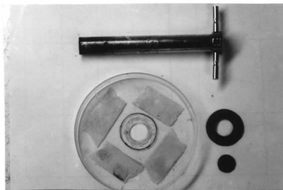
Figure 5. Summary of Bioassay Procedure (Ignoffo et al. 1976) Showing Cork Borer, PLastic Template, and Large Leaf Disk with Inner (Treated) Portion Removed.
