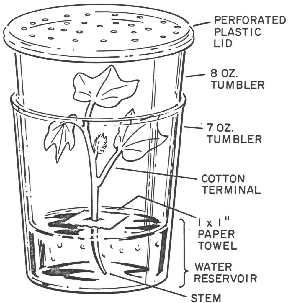
Figure 4. Microcages Used for Bioassay of Treated Terminals.
