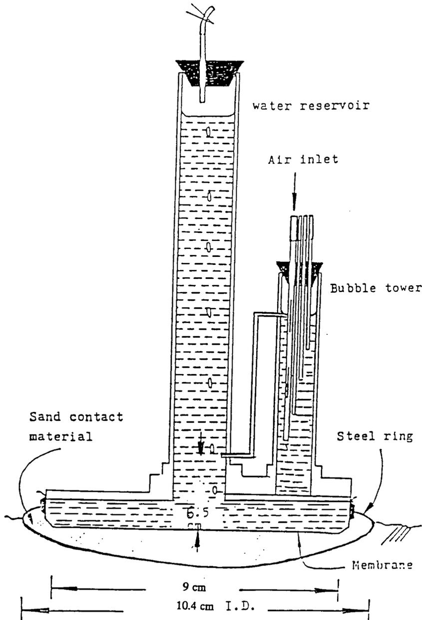
Figure 2.6. The small disc permeameter used for unsaturated water flow.
