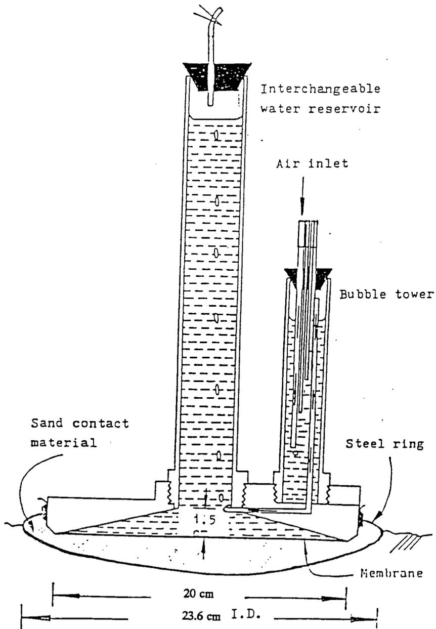
Figure 2.7. The large disc permeameter used for unsaturated water flow.
