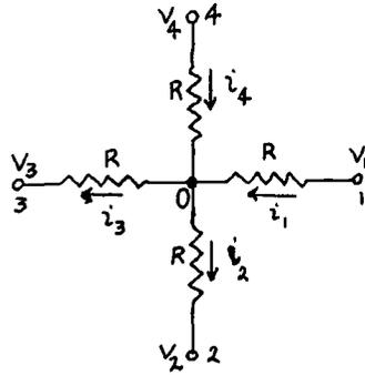
the current flowing through the resistors, and the sum of the currents are given in terms of voltages as:
