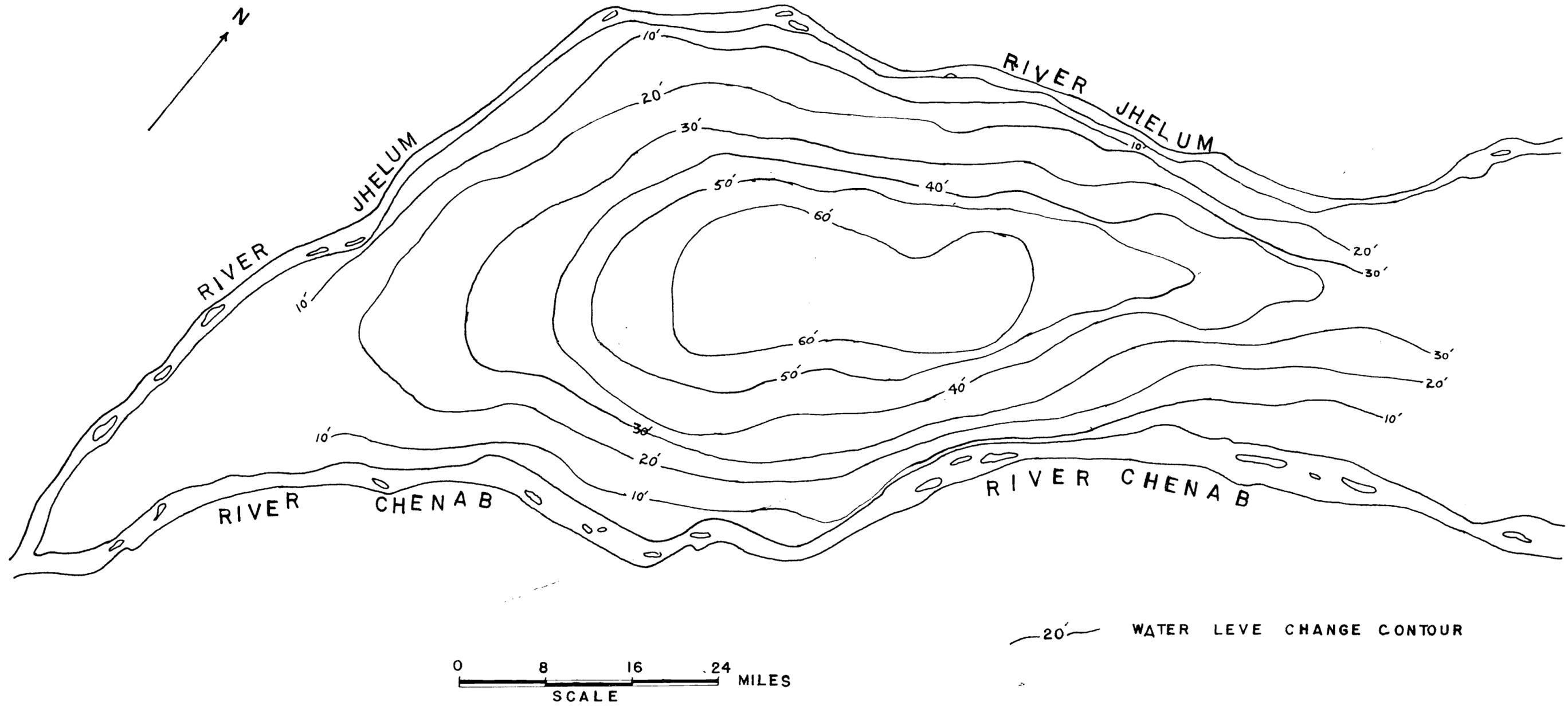
FIG. 13 CHANGE MAP SHOWING RISE IN GROUND WATER LEVELS (PRE-IRRIGATION TO 1960)
