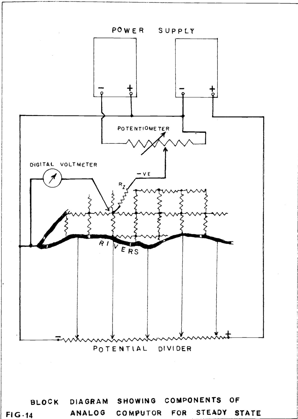
**FIG. 14** BLOCK DIAGRAM SHOWING COMPONENTS OF
