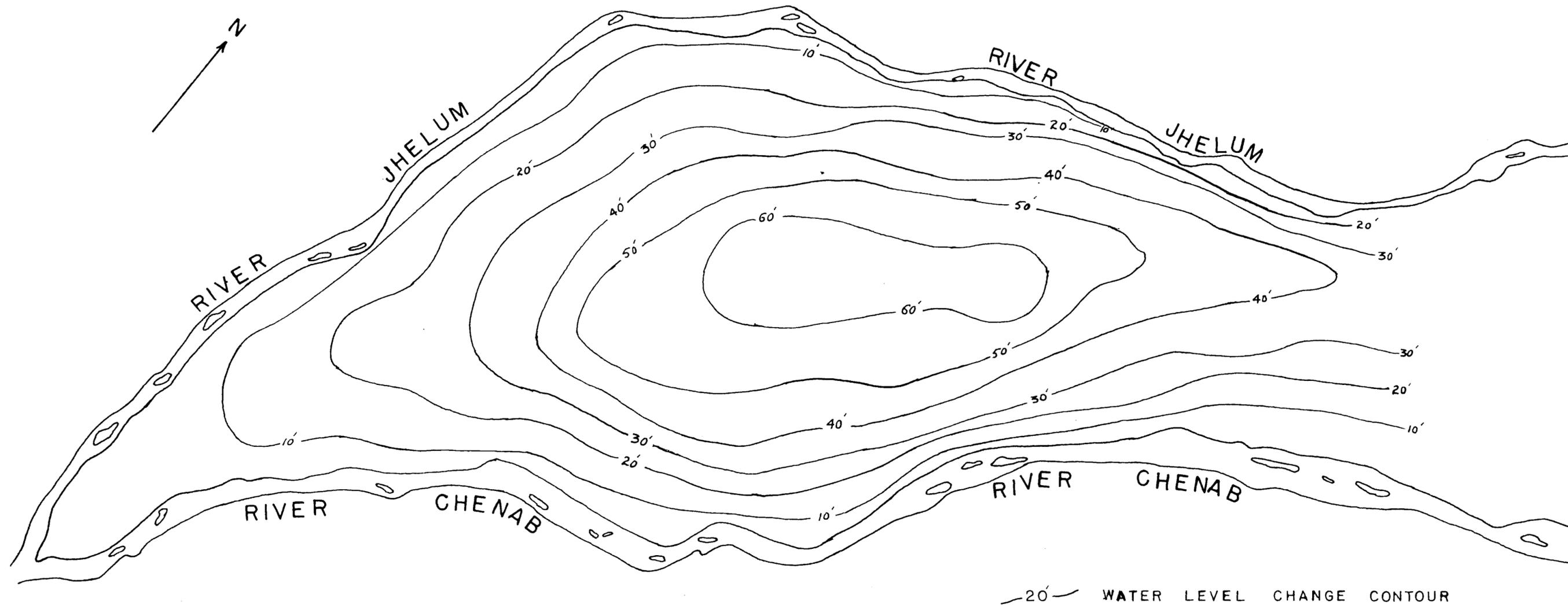
FIG. 21 CHANGE MAP SHOWING RISE IN GROUND WATER LEVELS (WITHOUT E.T.), (PRE-IRRIGATION TO 1960)
