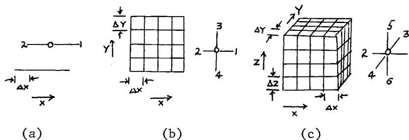
Consider first the one-dimensional field as shown in figure a. If the hydraulic heads  $h_1$ ,  $h_0$ , and  $h_2$  are assumed to exist at net points, respectively, the average hydraulic gradient between nodes 1 and 0 may be expressed as their head difference divided by the distance between them:
