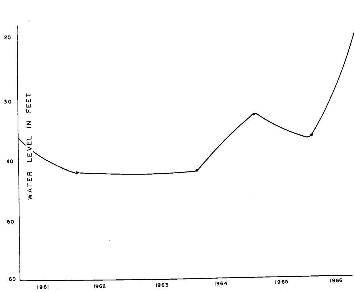
FIGURE. II Water level fluctuations for six years in well (22-16-5 cccd) in Sonoita Creek basin
