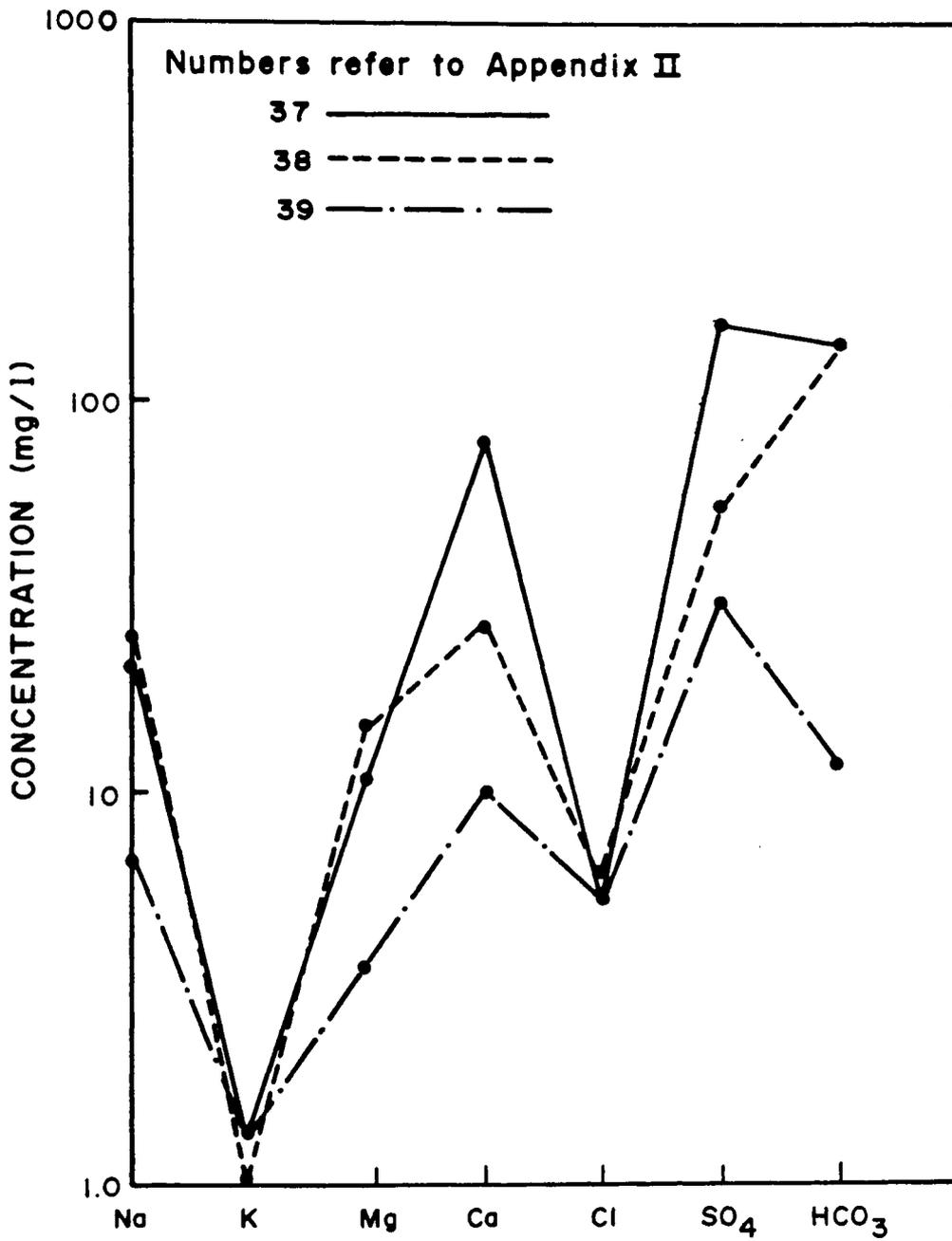
Figure 4.24. Finger-print diagrams of analyses of water samples from Chino Canyon.
