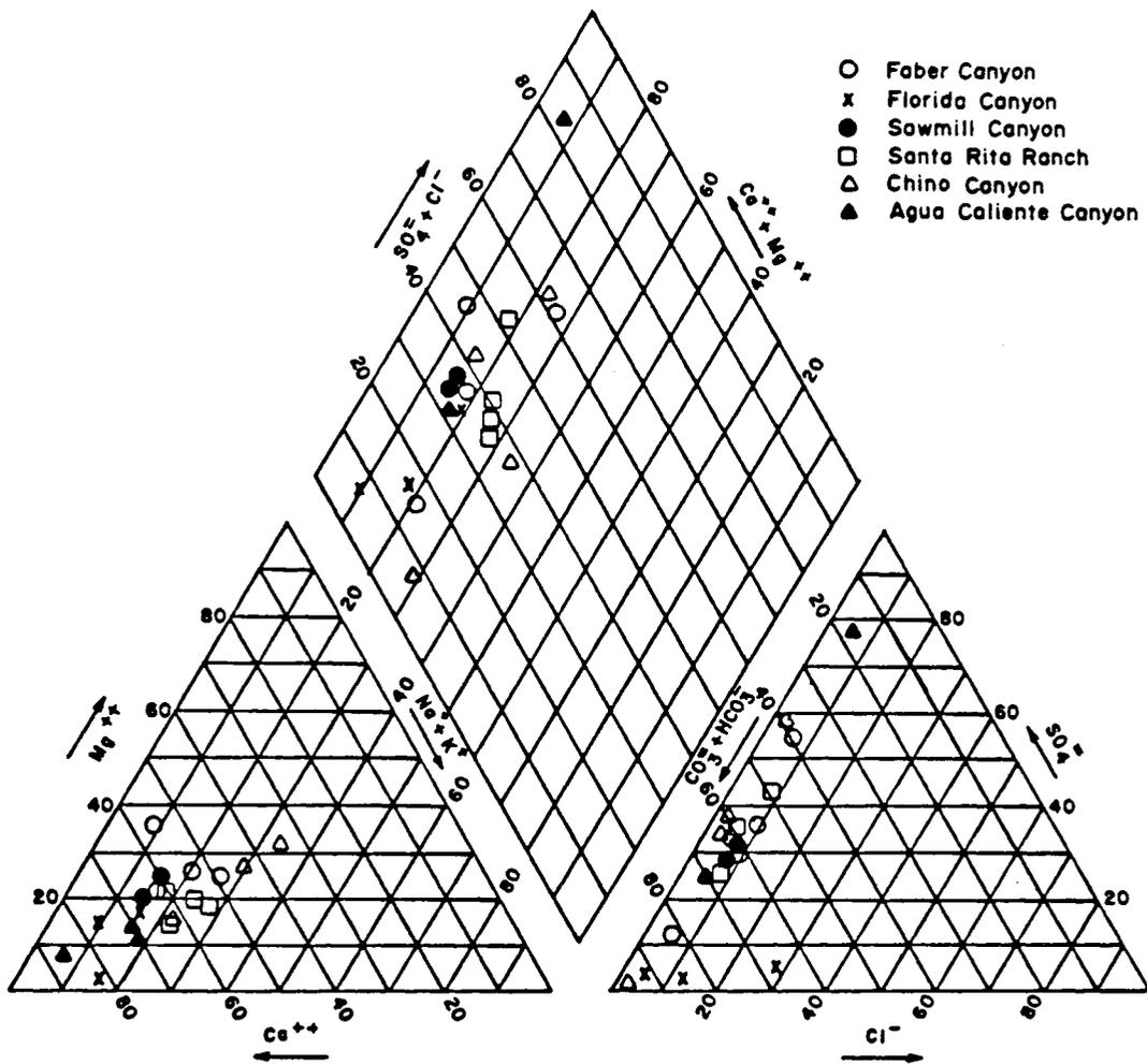
Figure 4.18. Trilinear diagram of analyses of water samples from from minor canyons.
