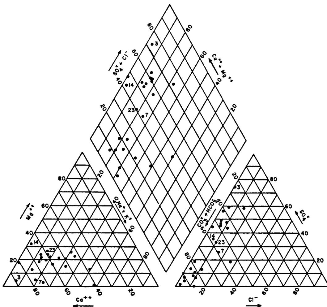
Figure 4.1. Trilinear diagram of analyses of water samples from Madera Canyon.
