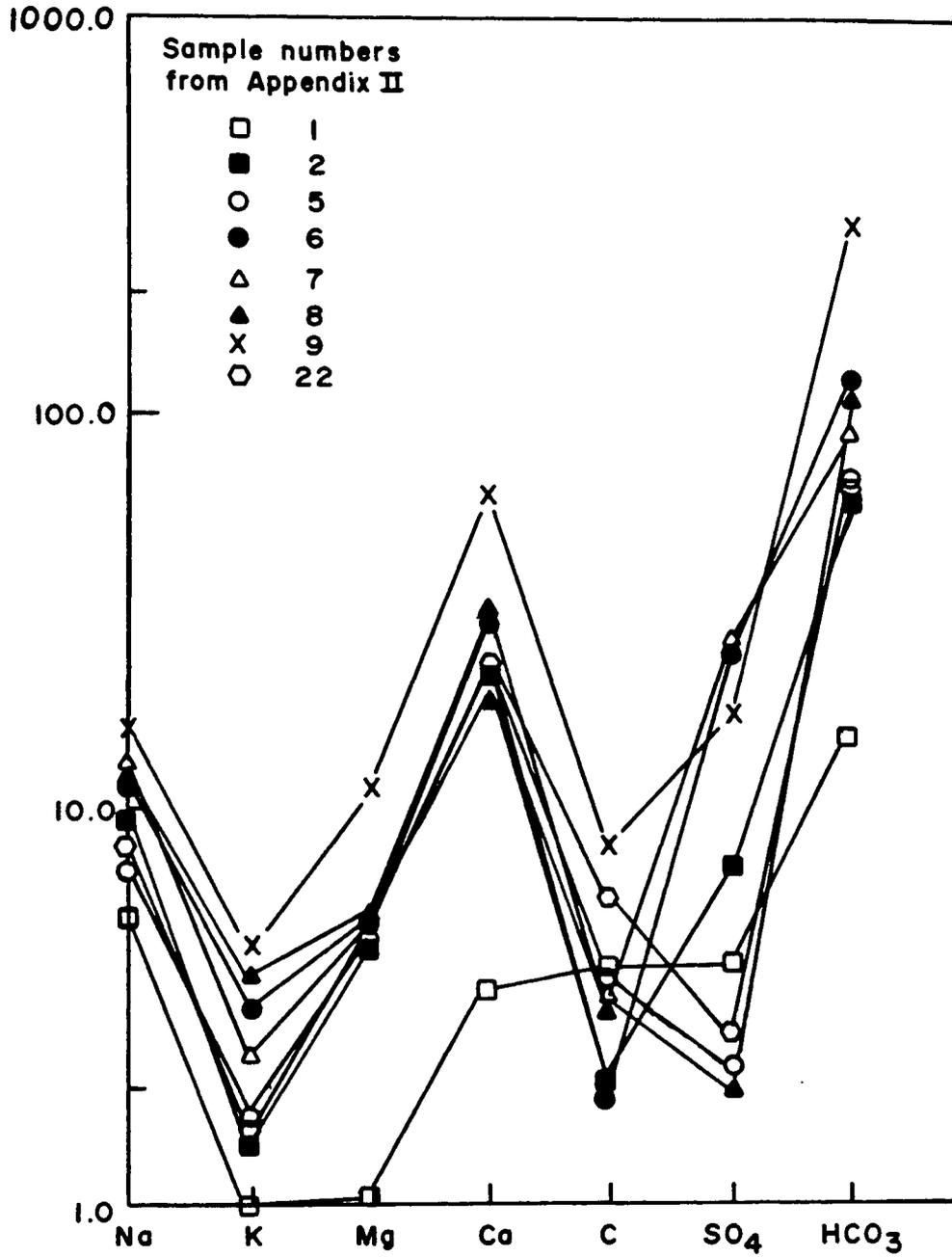
Figure 4.2. Finger-print diagrams of analyses of water samples from the east flank of Madera Canyon.
