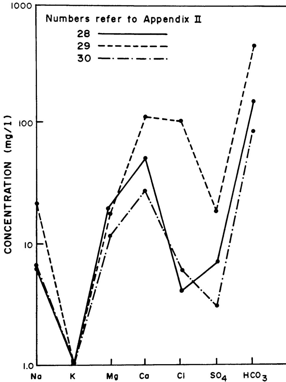
Figure 4.21. Finger-print diagrams of analyses of water samples from Florida Canyon.
