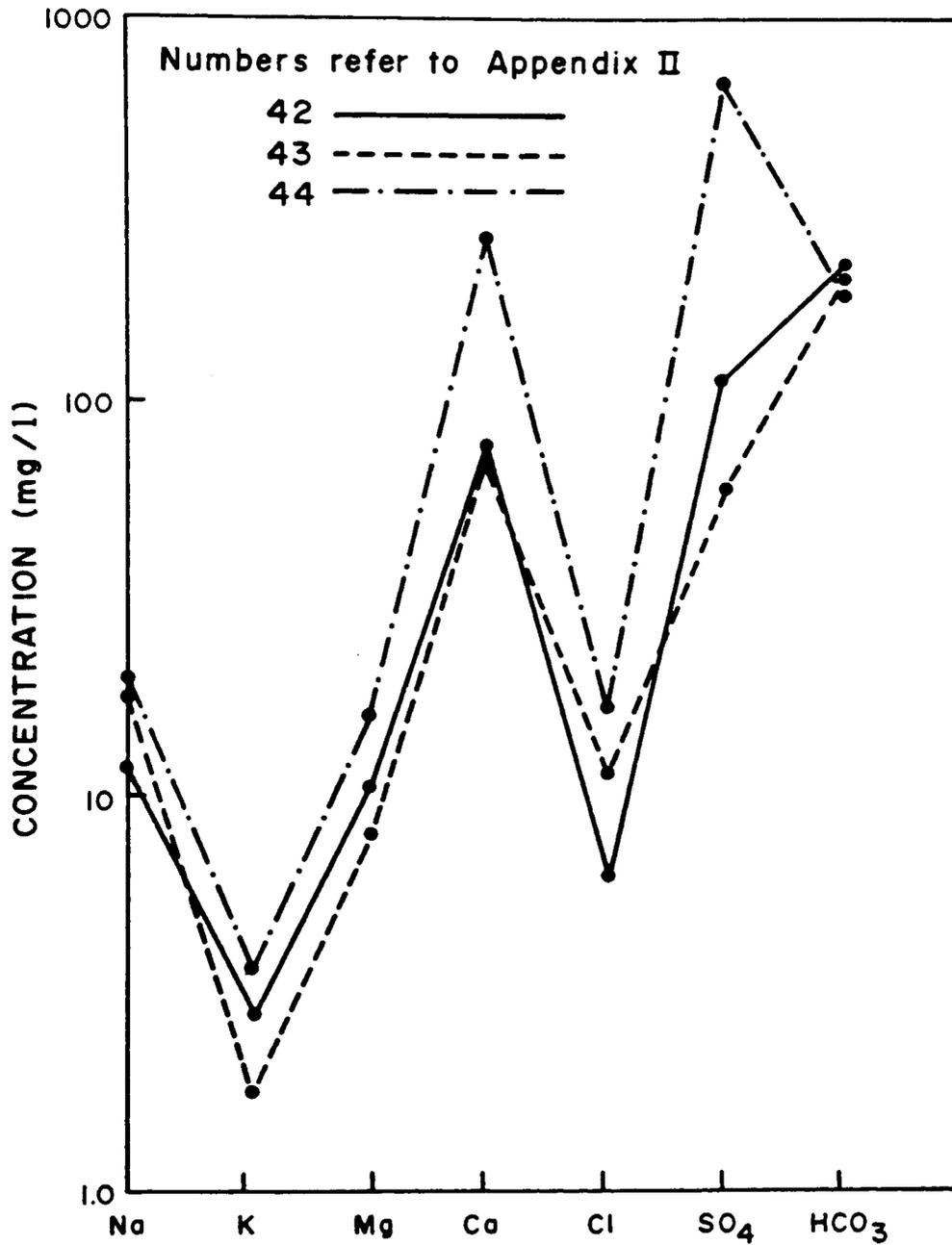
Figure 4.23. Finger-print diagrams of analyses of water samples from Agua Caliente Canyon.
