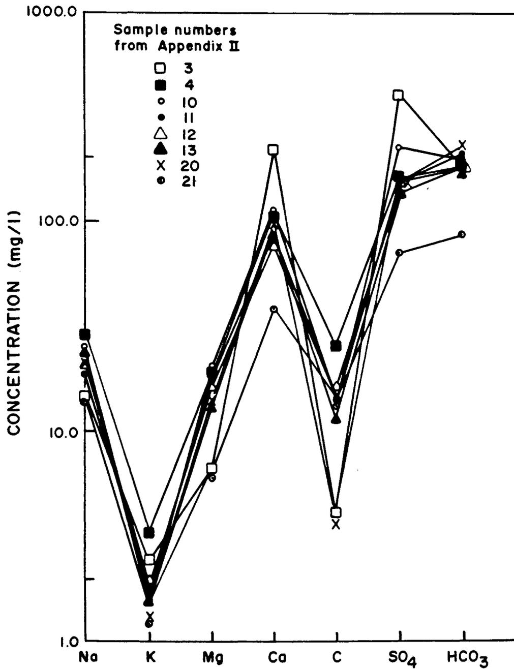
Figure 4.3. Finger-print diagrams of analyses of water samples from No Name Mine and near Madera Canyon stream.
