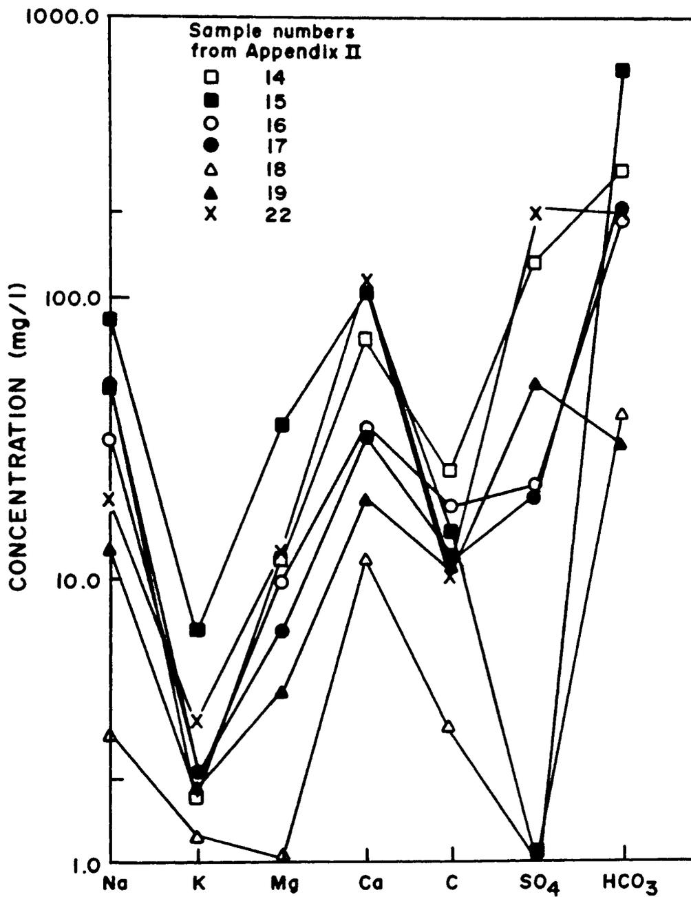
Figure 4.4. Finger-print diagrams of analyses of water samples from Madera Canyon fan.
