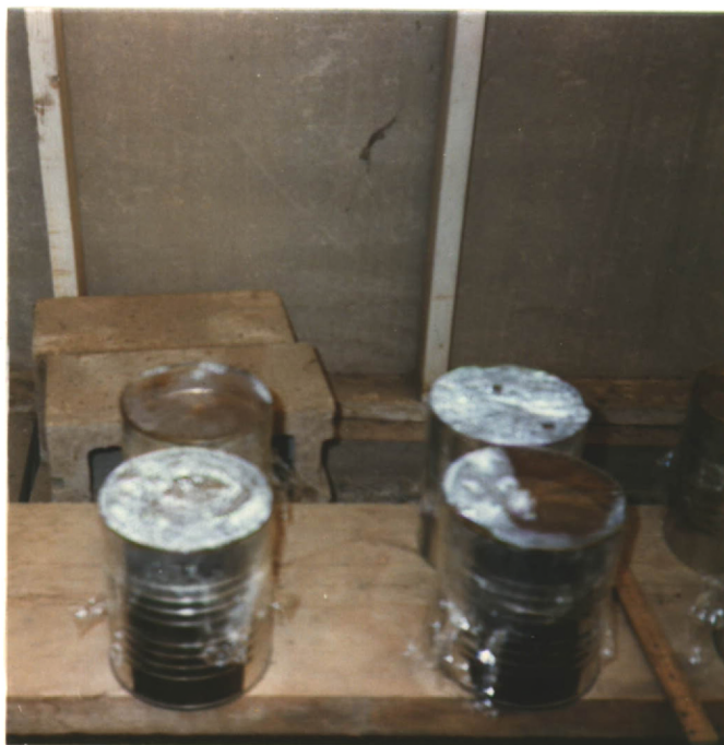
Figure 2. Evaporation reduced by packing cans with plastic.
