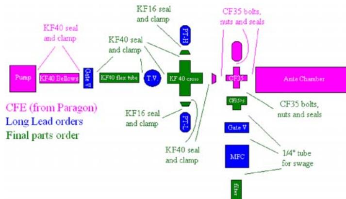
**Figure 1.1: Detailed Final Layout**
