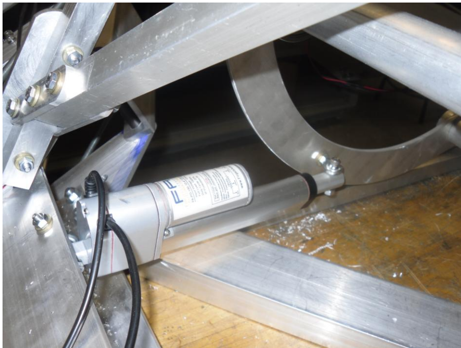
Figure 8. Linear actuator attached to laminate cage.
