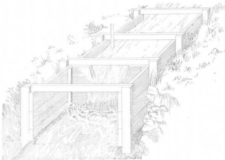
Fig. 4. Trapezoidal or Cippoletti weir box with 12 inch notch, showing construction and depth measurement. The scale is placed with the zero end at the level of the crest.
