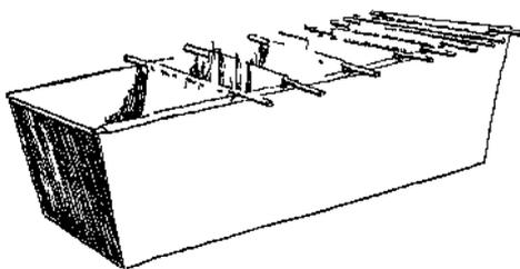
Fig. 1. Pan germinator, for testing several kinds of seeds at once.
