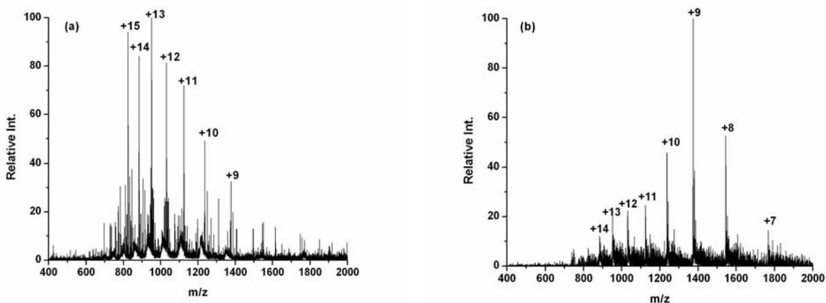
**FIGURE 4.6.** a) DESI mass spectrum of cytochrome c; b) NanoESI mass spectrum of cytochrome c. All mass spectrometry parameters remain the same for those two measurements.
