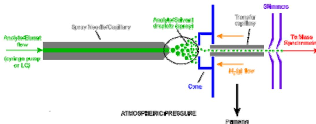
**FIGURE 1.1.** A schematic diagram of an electrospray ionization source (ESI) interface (figure from [www.bris.ac.uk/nerclmsmf/techniques/hplcms.html](http://www.bris.ac.uk/nerclmsmf/techniques/hplcms.html)) [6].
