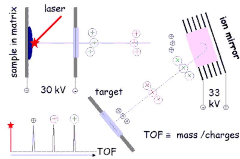
**FIGURE 1.6.** A schematic diagram of a MALDI-TOF instrument (figure from <http://edoc.hu-berlin.de/dissertationen/xie-jing-2003-12-15/HTML/chapter2.html>)[35]
