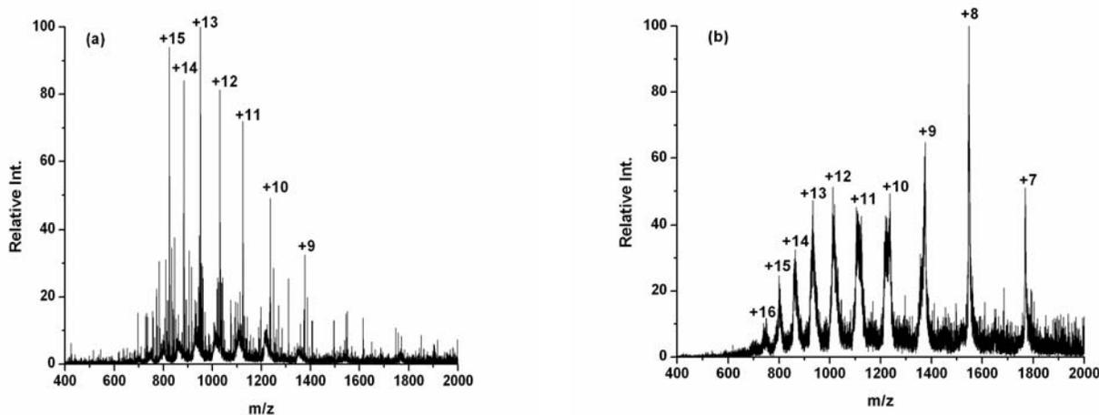
**FIGURE 4.5.** DESI mass spectra of cytochrome c: a) The spectrum was collected under optimum condition; b) the spectrum was collected when the sprayer and sample surface are much closer to the mass spectrometer inlet.
