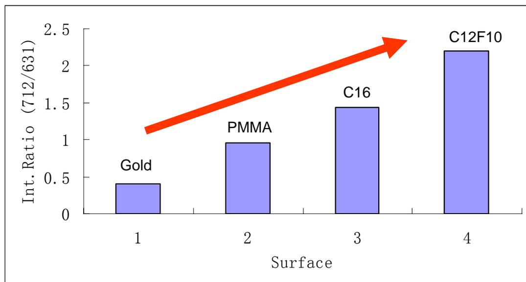
**FIGURE 4.8.** The peak intensity ratios between  $m/z = 712$  (YGGFLR) and  $m/z = 631$  for different surfaces used in DESI-MS.
