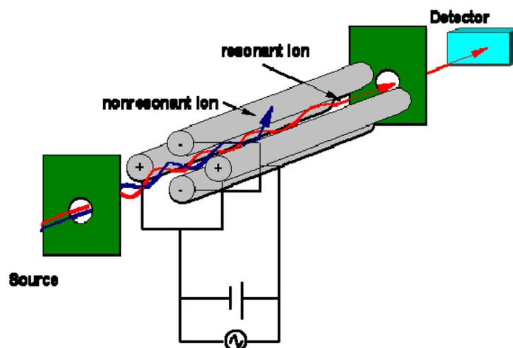
**FIGURE 1.3.** A schematic diagram of a quadrupole mass analyzer (figure from <http://www.ivv.fraunhofer.de/ms/ms-analyzers.html>) [27].
