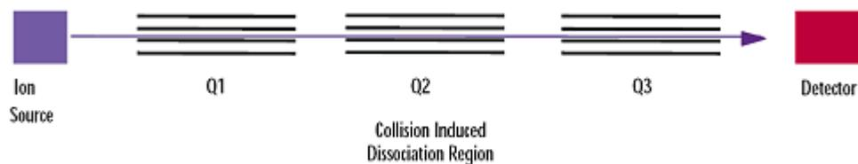
**FIGURE 1.4.** A schematic diagram of a triple quadrupole mass spectrometer (figure from <http://www.waters.com>) [29].
