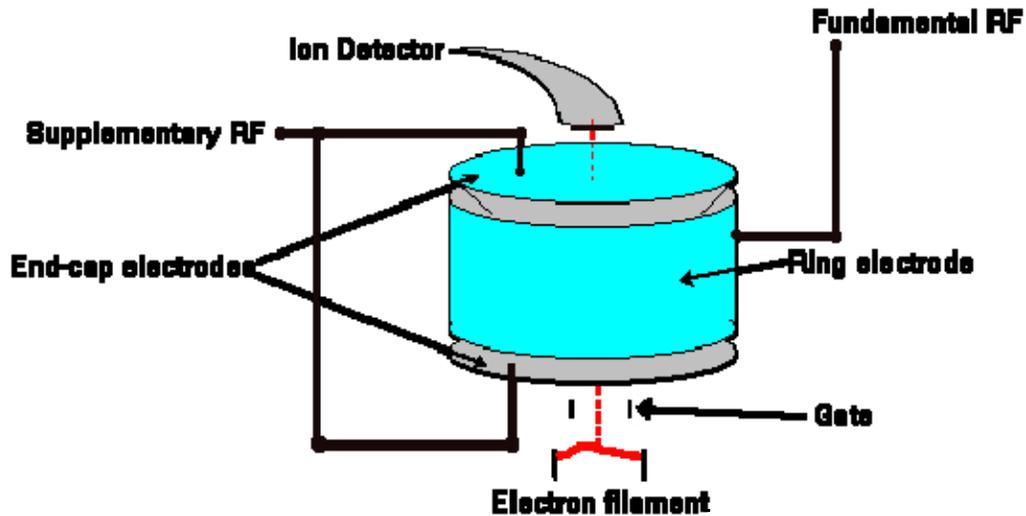
**FIGURE 1.5.** A schematic diagram of quadrupole ion trap mass analyzer (QIT) (figure from <http://www.ivv.fraunhofer.de/ms/ms-analyzers.html>) [33].
