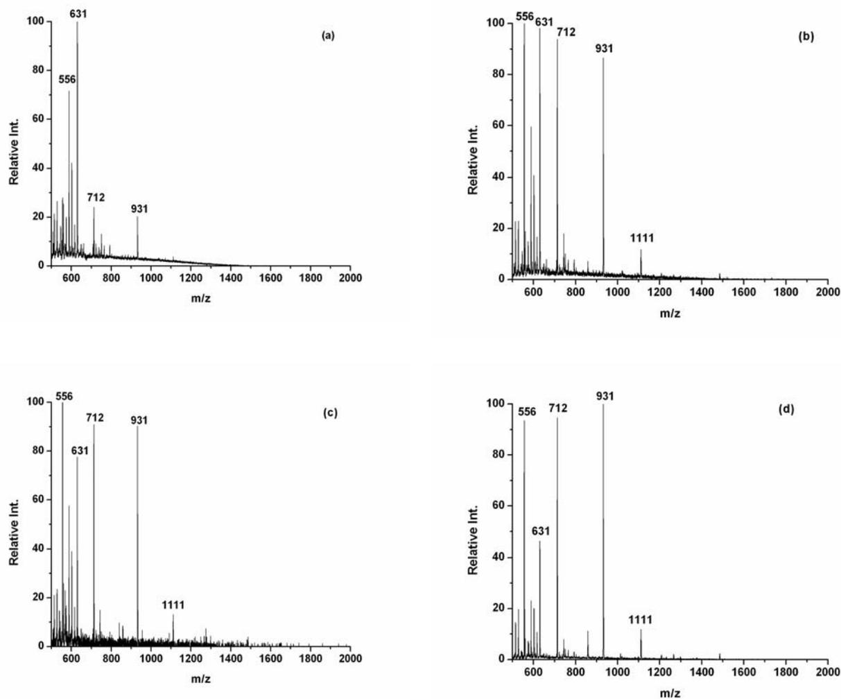
**FIGURE 4.7.** DESI-MS spectra of YGGFL, YGGFLR and angiotensin3 (RVYIHPF) mixture: a) bare gold; b) PMMA; c) C16 self assembled monolayer on gold; and d) C12F10 self assembled monolayer on gold.
