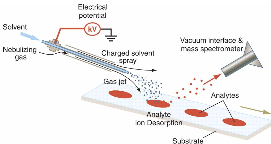
**FIGURE 4.1.** A diagram of desorption electrospray ionization source (Figure from reference [4] with permission).
