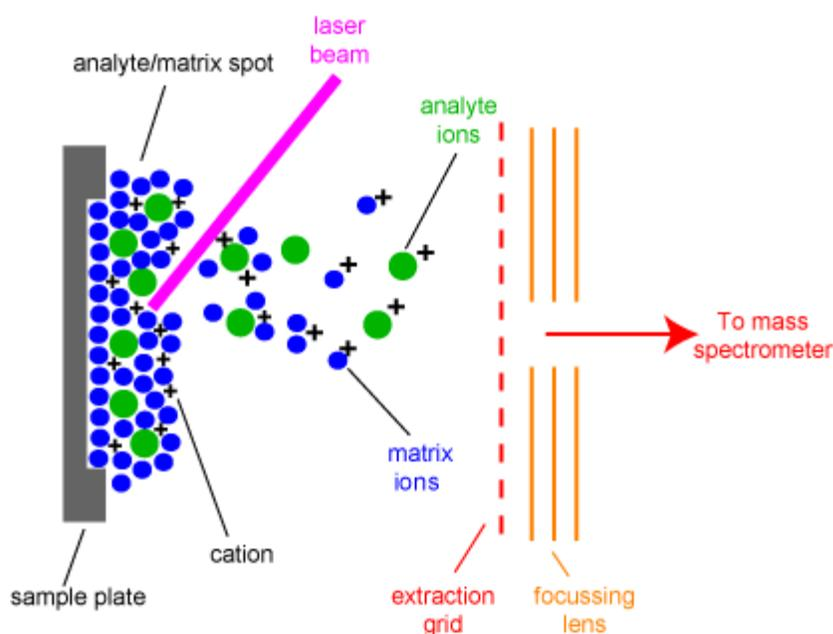
**FIGURE 1.2.** A schematic diagram of matrix assisted laser desorption ionization (figure from <http://www.chm.bris.ac.uk/ms/theory/maldi-ionisation.html>) [21].
