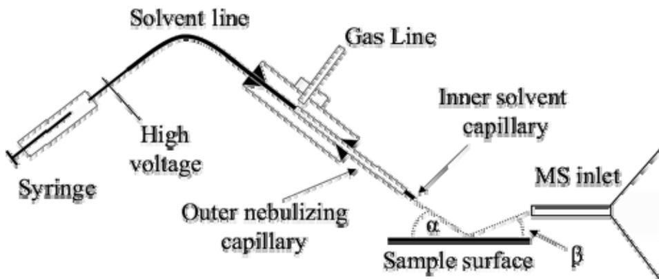
**FIGURE 4.3.** A diagram of DESI sprayer. (Figure from Reference [16] with permission)
