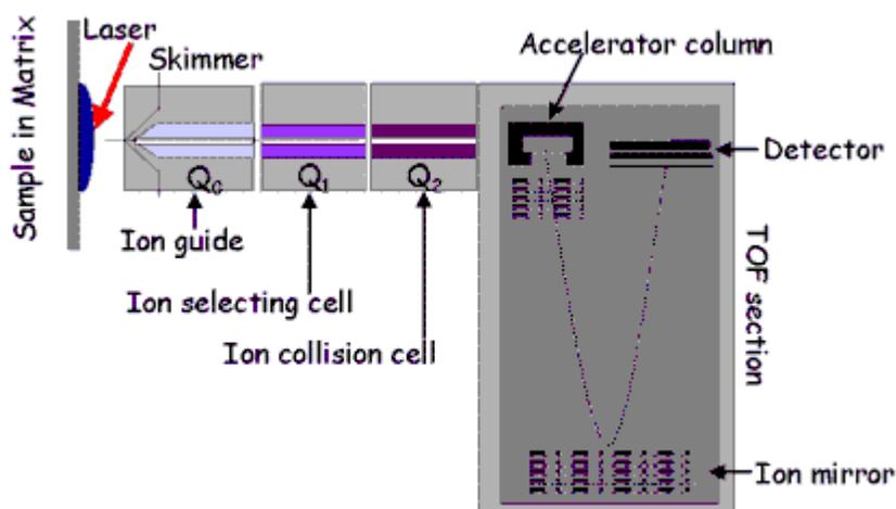
**FIGURE 1.7.** A schematic diagram of a MALDI-QTOF mass spectrometer (figure from <http://edoc.hu-berlin.de/dissertationen/xie-jing-2003-12-15/HTML/chapter2.html>) [39].
