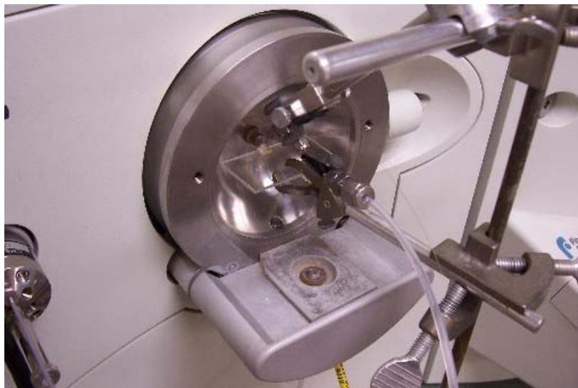
**FIGURE 4.2.** The set-up of DESI source used in the present study.
