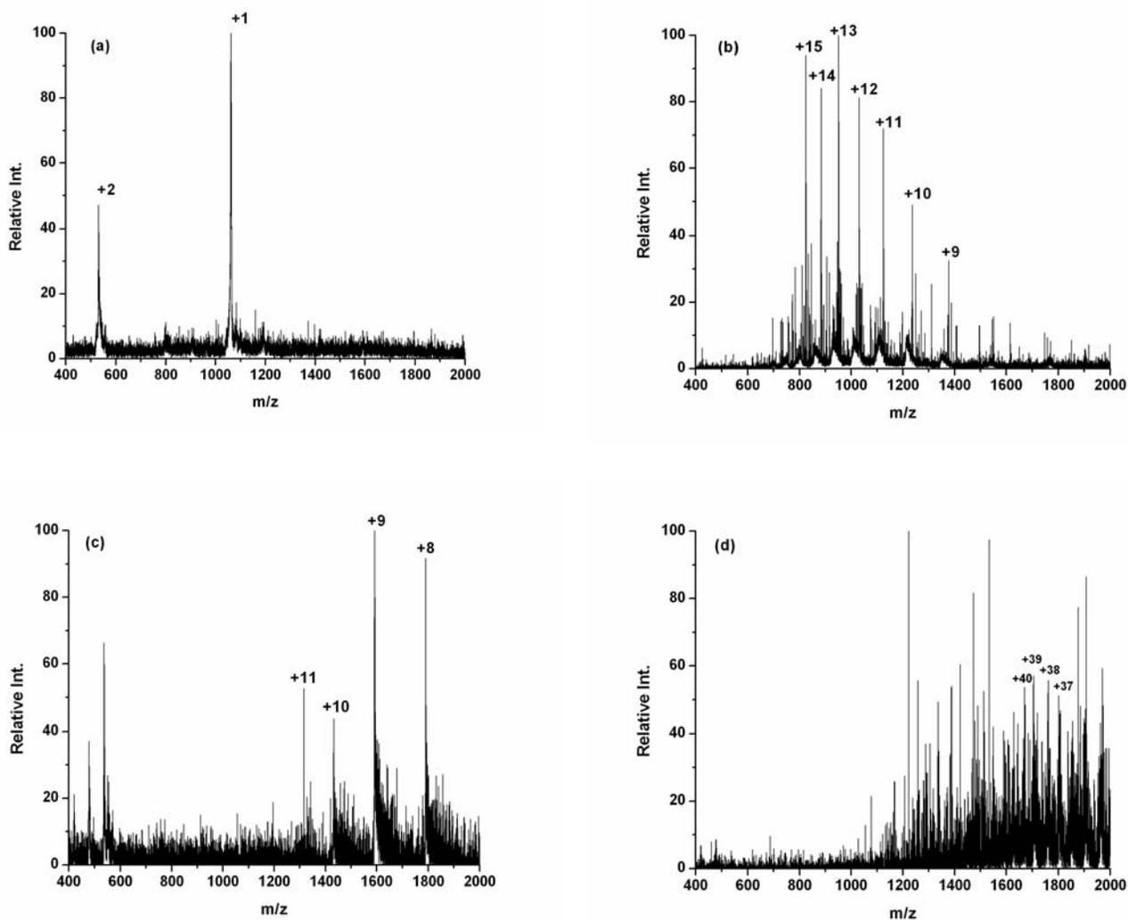
**FIGURE 4.4.** DESI mass spectra of intact peptide and protein standards under optimum conditions: a) bradykinin (1.06 kDa); b) cytochrome c (12.3 kDa); c) lysozyme (14.3 kDa) and BSA (66.4 kDa). The peptide and proteins ( $\sim 1 \mu\text{M}$ ) were deposited on a PMMA surface.
