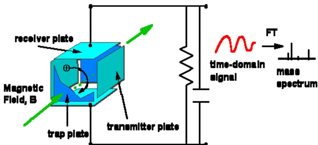
**FIGURE 1.8.** A schematic diagram of a FT-ICR mass analyzer (figure from <http://www.ivv.fraunhofer.de/ms/ms-analyzers.html>) [41].
