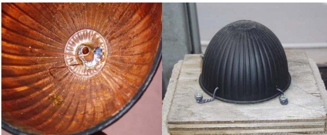
Figure 4.2.3.1. Construction of globe thermometer. Internal view of copper coil for insertion of thermistor (left) (prior to addition of thermistor and insulation foam) and view of completed globe thermometer (right).
