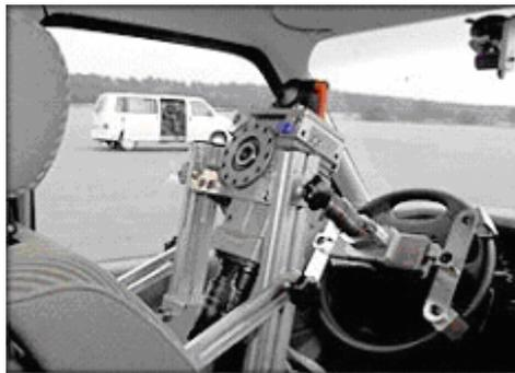
Figure 1.1 "Klaus," the driving robot developed by German carmaker Volkswagen, drives a VW Multi-van on a test track (from <http://www.vw-personal.de/>)
