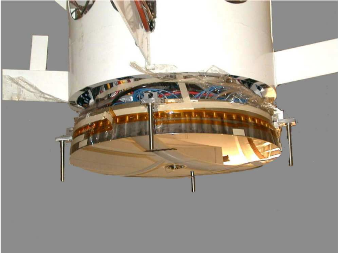
Figure 1.2 The MMT's adaptive optics secondary mirror. (Photo courtesy Center for Astronomical Adaptive Optics)
