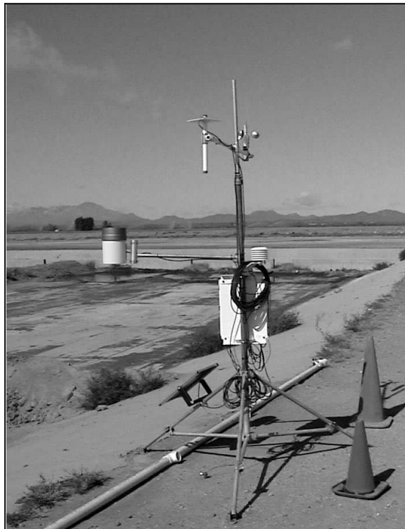
Figure -2. Remote weather station and data acquisition system
