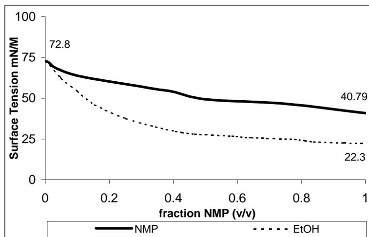
**Figure 20: Surface Tension of cosolvent-water mixtures**
