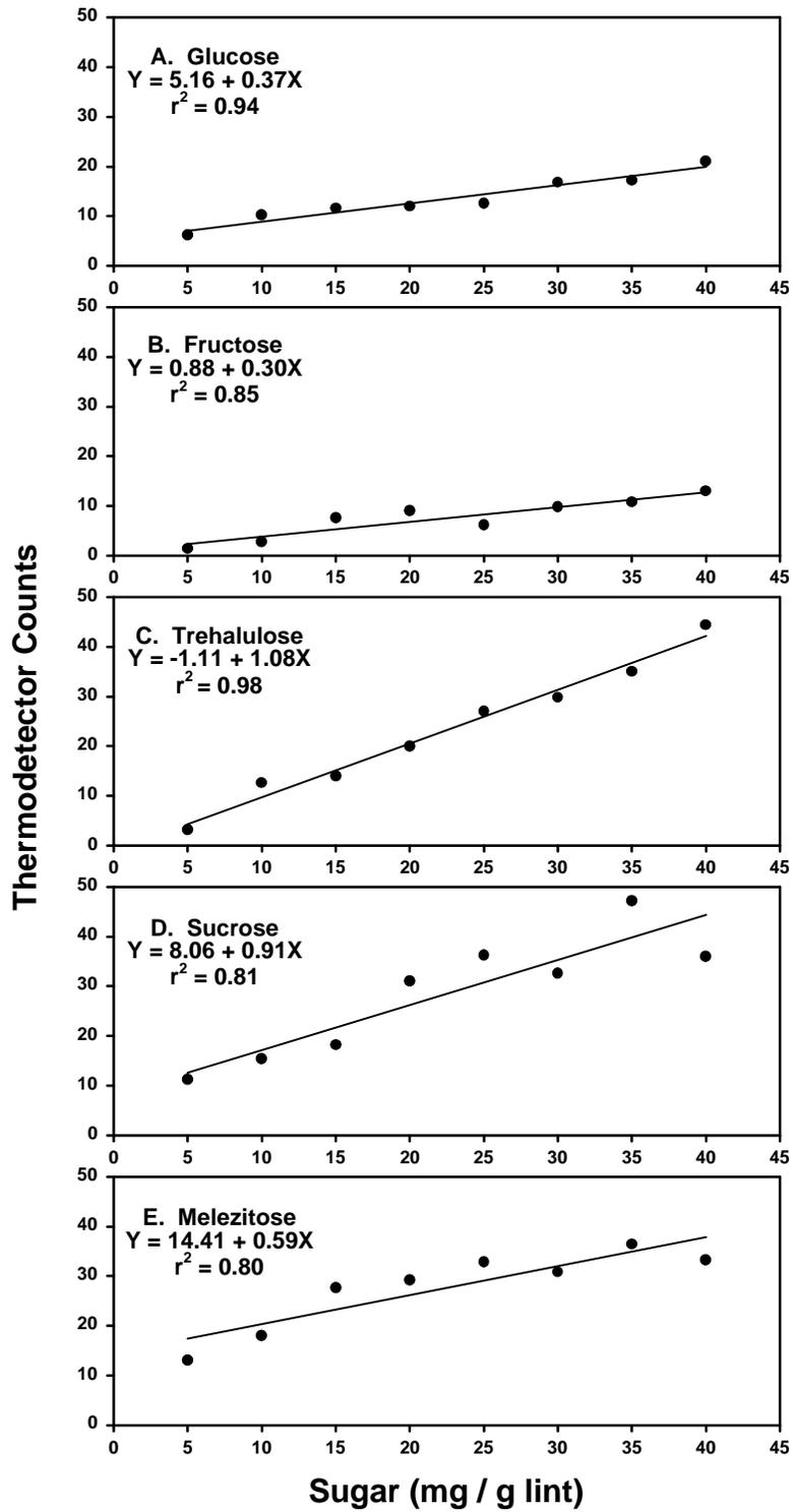
Figure 1. Mean numbers of thermodetector counts for cotton lint sprayed with individual honeydew sugars at different concentrations.
