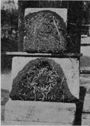
Plate V.—Results of preliminary washing test on adobes, upper adobe from Lot 7 and lower adobe from University of Arizona Farm stack. The melting away of the adobe at the lower edge of the latter is clearly shown.
