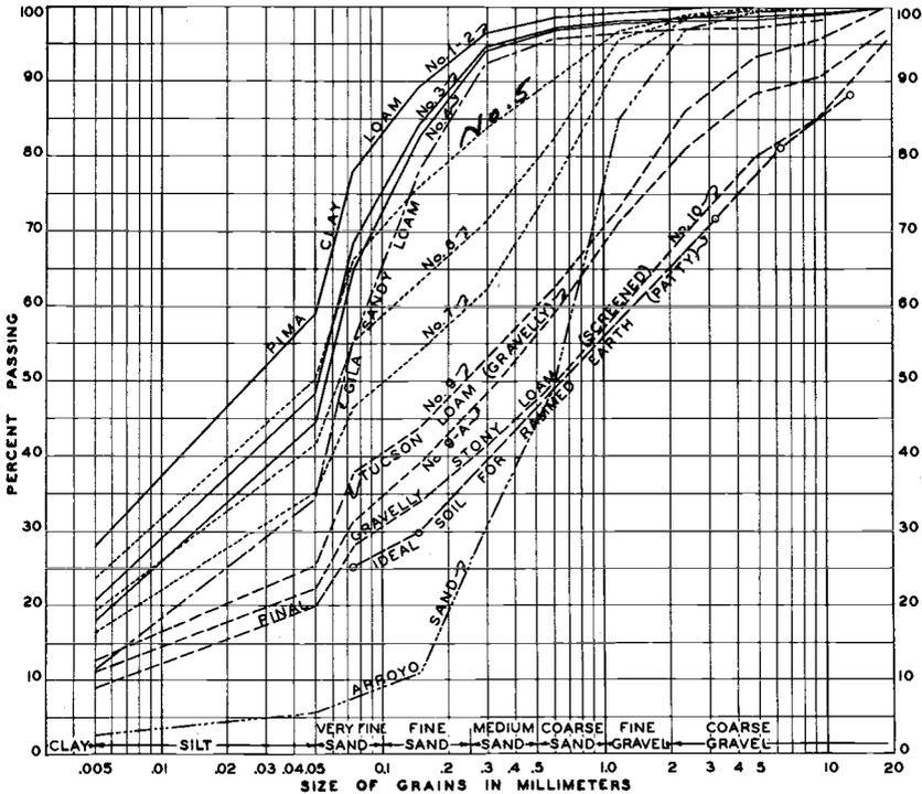
Figure 1.—Curves showing the results of mechanical analyses of soils and soil mixtures used in making test adobes. Curves No. 1-2 and No. 10 mark the approximate upper and lower limits of soils from which adobes can be made. The curve marked "Patty" was found ideal for rammed earth walls.
