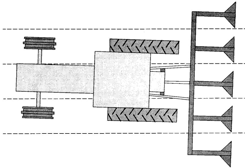
Figure 1. Implement "tailout" caused by the geometry of the tractor and implement combination. When the front of the tractor moves in one direction, the implement immediately moves in the opposite direction.
