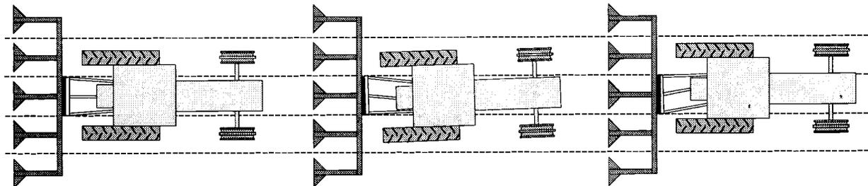
Figure 3. The action of an articulated or pivot guidance system; showing (left) both tractor and implement correctly aligned to the rows, (center) the tractor out of parallel to the rows and implement tailout completely compensated for by the pivoting action of the guidance system, and (right) tractor mis-aligned and parallel to the rows with the implement correctly aligned to the rows.
