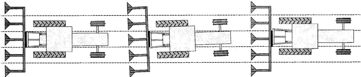
Figure 2. The action of a side-shift or push guidance system; showing (left) both tractor and implement correctly aligned to the rows, (center) the tractor out of parallel to the rows and the implement tailout partially compensated for by the side-shifting action of the guidance system, and (right) tractor mis-aligned and parallel to the rows with the implement correctly aligned to the rows.
