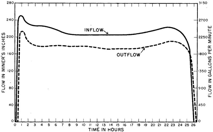
FIGURE 2.—Pattern of seepage loss on Test 3, unlined ditch, Mohave fine sand and sandy loam.
