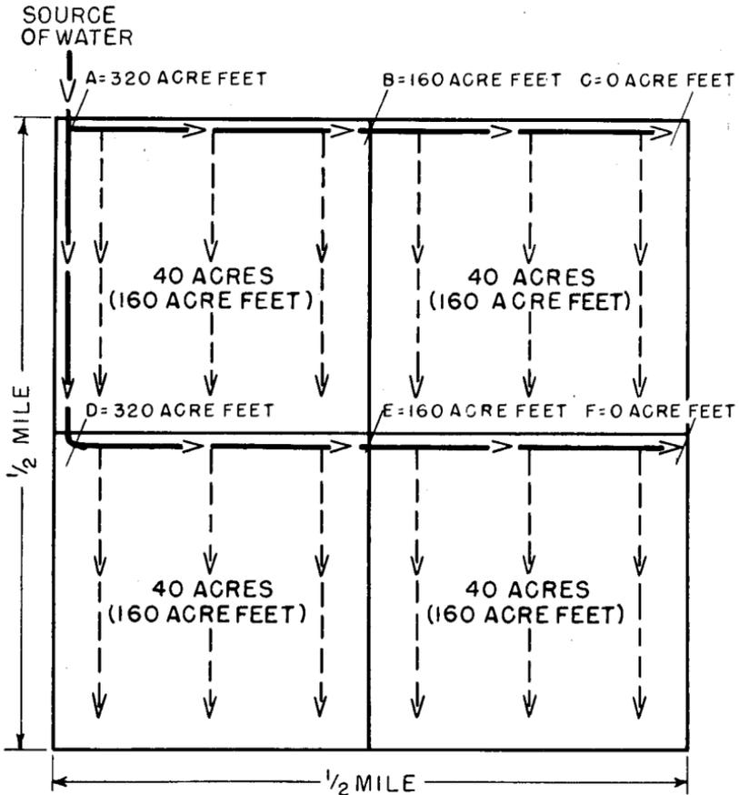
FIGURE 5.—Field layout and amount of water carried in each section of the ditch where the water is delivered to the high point of each  $\frac{1}{4}$  section of land.
