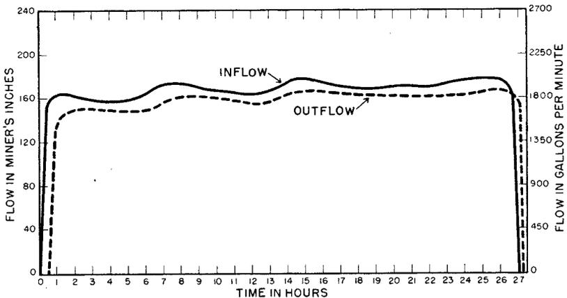
Figure 3.—Pattern of seepage loss on Test 4, unlined ditch, Cajon silty clay loam (shallow phase).
