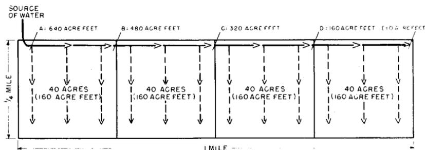
FIGURE 4.—Field layout and the amount of water carried in each section of the irrigation ditch where 160 acres are irrigated from 1 mile ditch.
