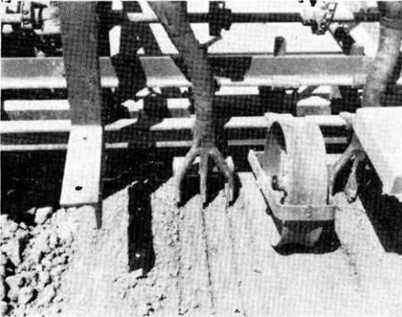
**Figure 4.—(top, left) 4-inch splatter-type shoe. Note triangle-shaped tongue in center of shoe to aid in spreading seed.**
