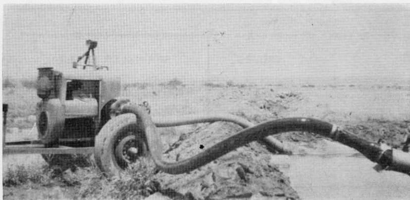
Plate XI.—A portable pumping unit with air-cooled gasoline engine direct-connected to a 4-inch centrifugal pump used for sprinkler irrigation of permanent pasture near Hereford, Arizona.
