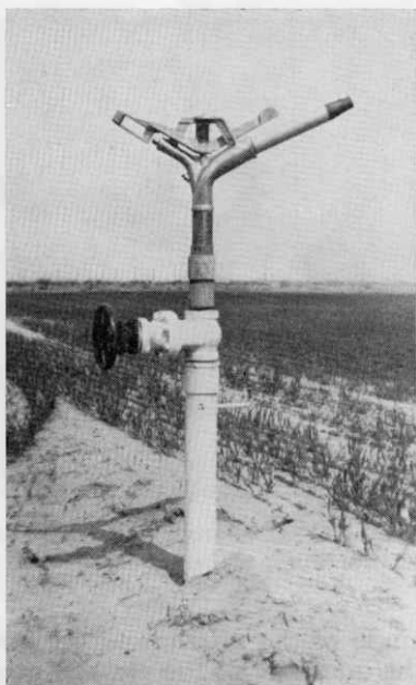
Plate X.—Large volume sprinkler capable of discharging up to 600 gpm.
