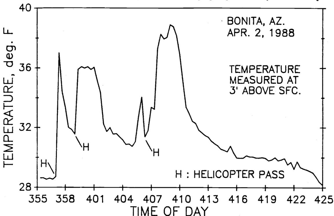
Figure 3. Response of orchard temperature to multiple passes of a helicopter. Air temperature was recorded at 3' above the orchard floor.
