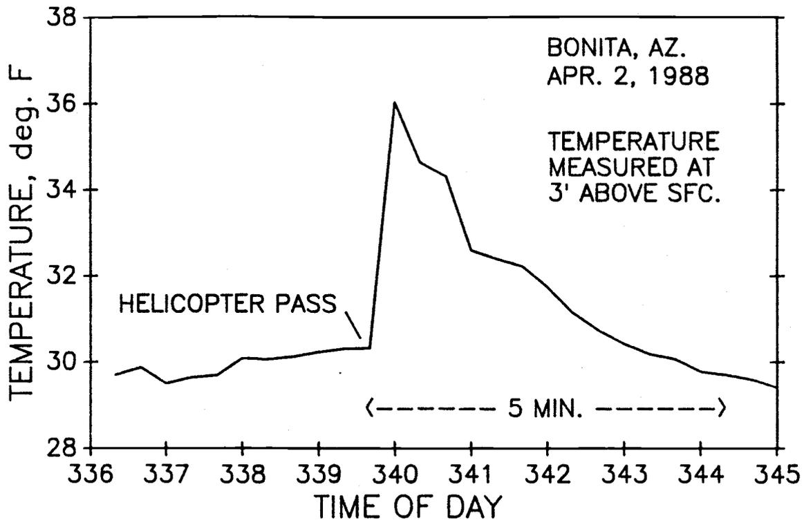
Figure 2. Air temperature at 3' above the orchard floor prior to, during and following a single pass of a helicopter.
