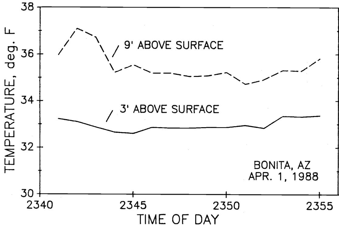
Figure 1. Air temperatures recorded at 3' and 9' above the orchard floor clearly show the presence of a temperature inversion.
