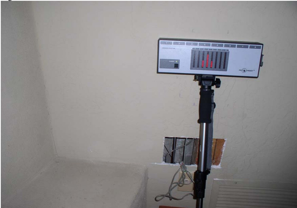
a) Motion detection of termites within a wall by Pestfinder.
