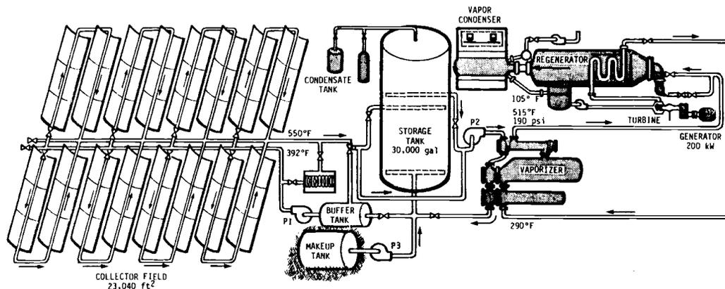
Figure 1. Schematic diagram of the solar thermoelectric power plant at Coolidge, Arizona
