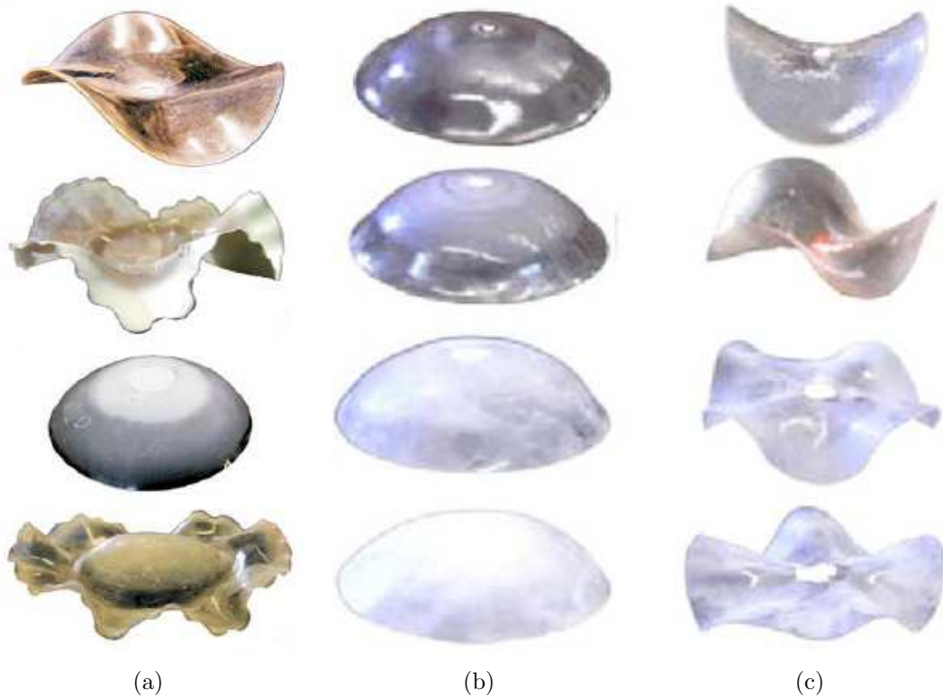
FIGURE 1.4. (a) By controlling the Gaussian curvature K_0 , non-Euclidean plates of different shapes can be constructed (Klein et al., 2007). In the top two images K_0 < 0 leading to rippled shapes. In the third image from the top K_0 > 0 leading to a spherical dome like shape. The hydrogel in the bottom image is a combination of an interior region with K_0 > 0 and an outer region with K_0 < 0 . (b) The equilibrium shapes of hydrogel disks of constant radius of R = 14mm and varying thickness ( t = .75mm , .6mm , .25mm , and .19mm from top to bottom) with a constant Gaussian curvature K = .0011mm^{-2} (Klein et al., 2011). (c) The equilibrium shapes of hydrogel disks of constant radius of R = 14mm and varying thickness ( t = .75mm , .6mm , .25mm , and .19mm from top to bottom) with a constant Gaussian curvature K = -.0011mm^{-2} (Klein et al., 2011).
