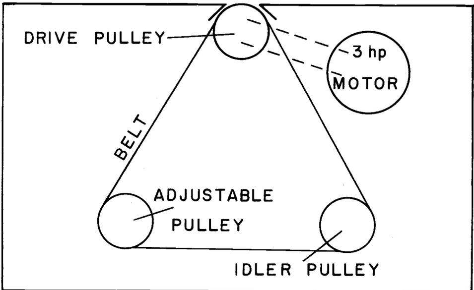
FIG. 2. Schematic sketch of details of sanding machine.
