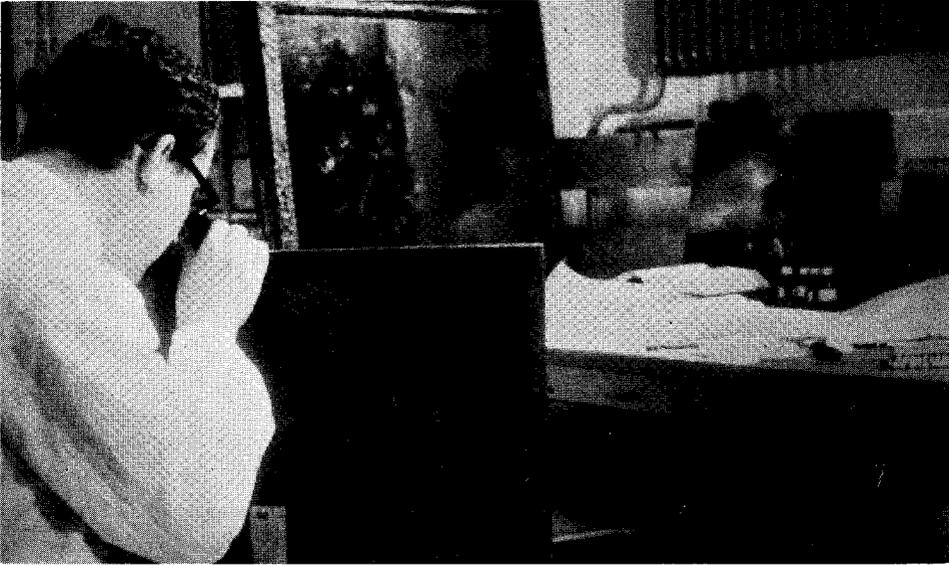
Figure 5. A panel of a Wouwerman painting is investigated for its tree-ring characteristics.
