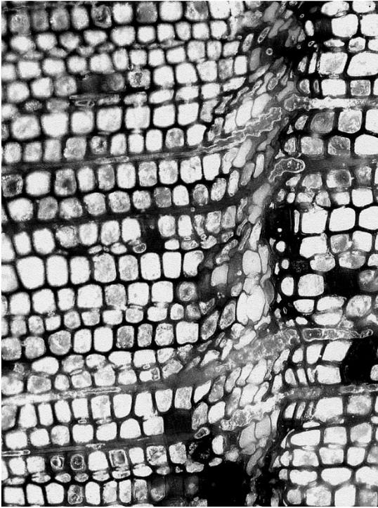
Figure 3. Frost damage in the 1979-138 specimen.
