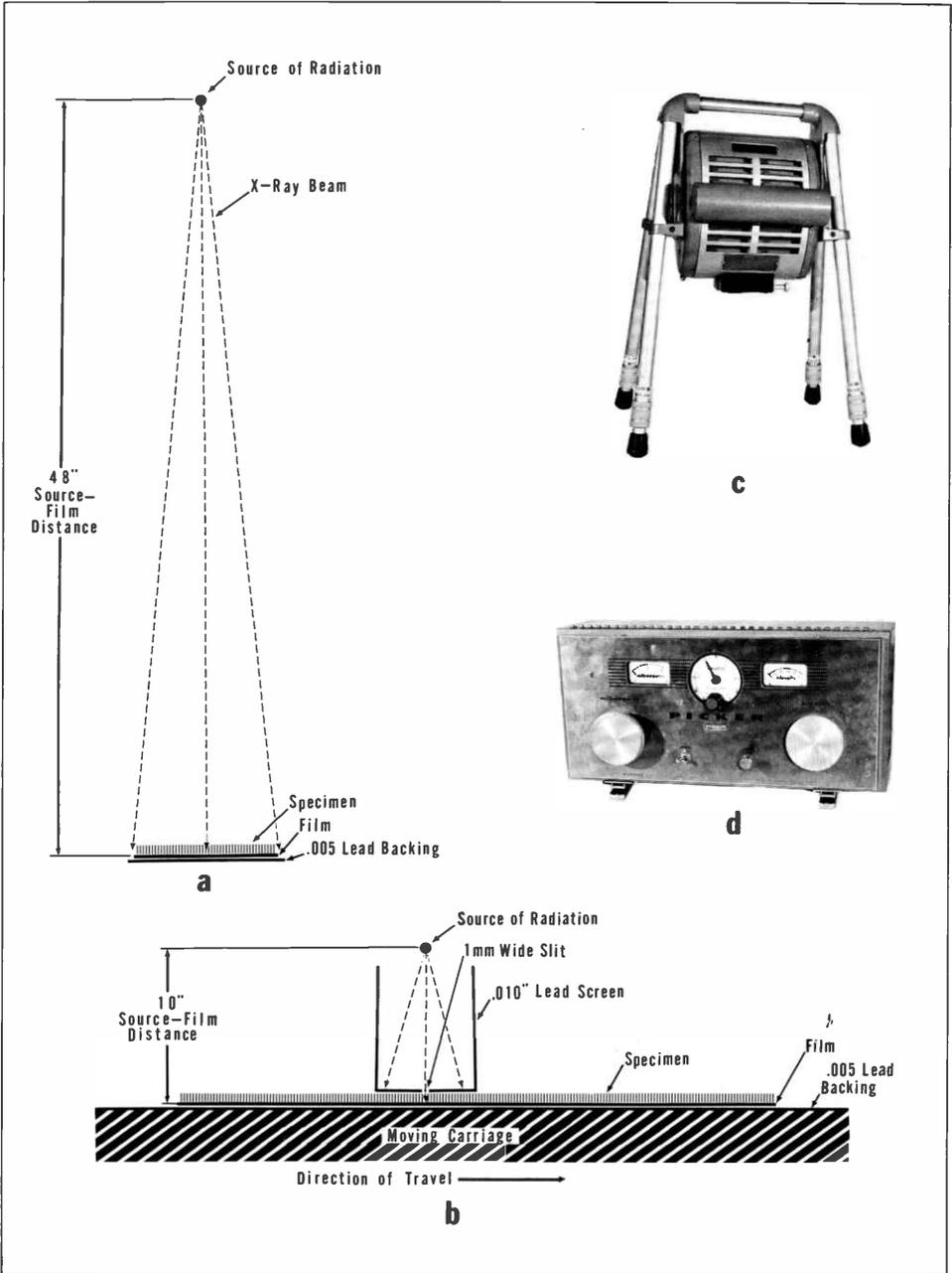
Fig. 5. X-ray techniques *a*, stationary technique; *b*, in-motion technique; *c* X-ray tube; *d*, electronic controls.
