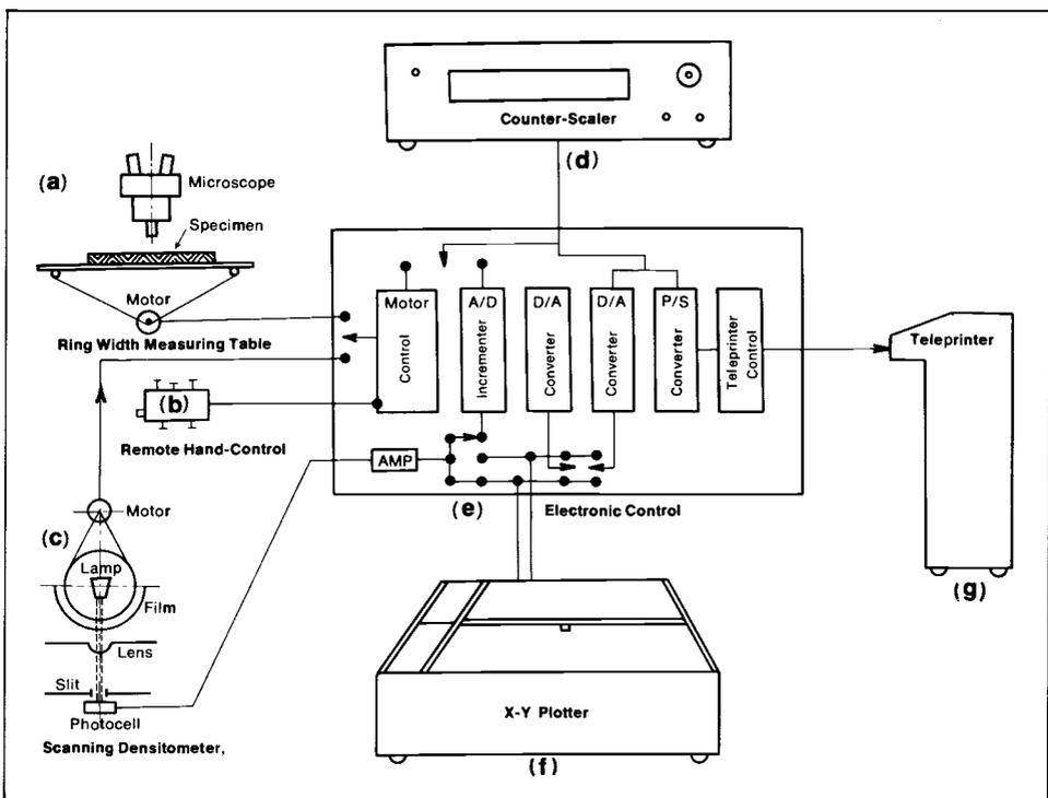
Fig. 5. Schematic Diagram of the System
