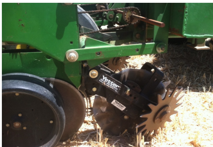
Figure 2. Yetter™ equipment attached to the front of planter disk to push away grain straw and loosen up the soil.
