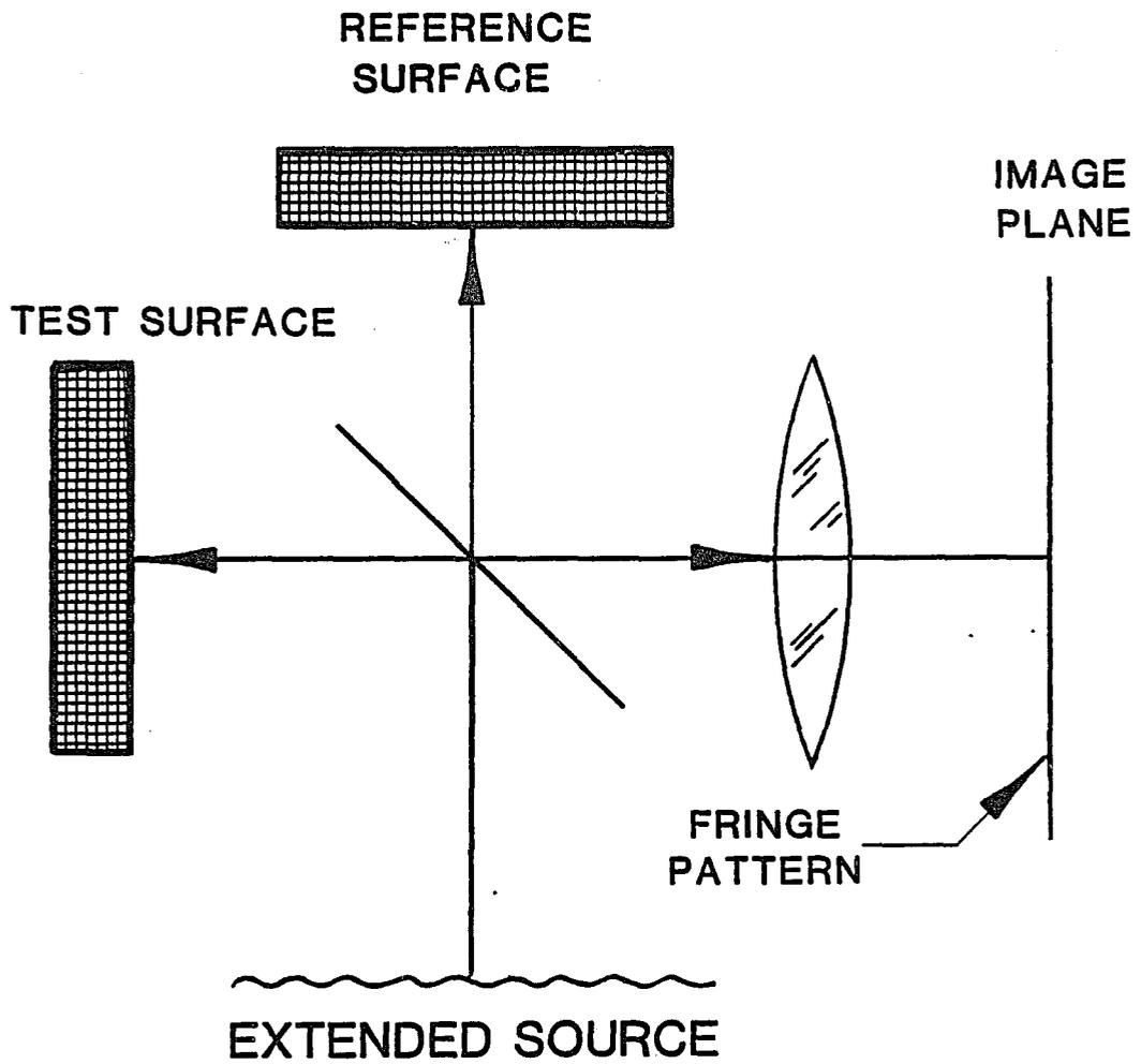
Fig. 7. Michelson Interferometer.
