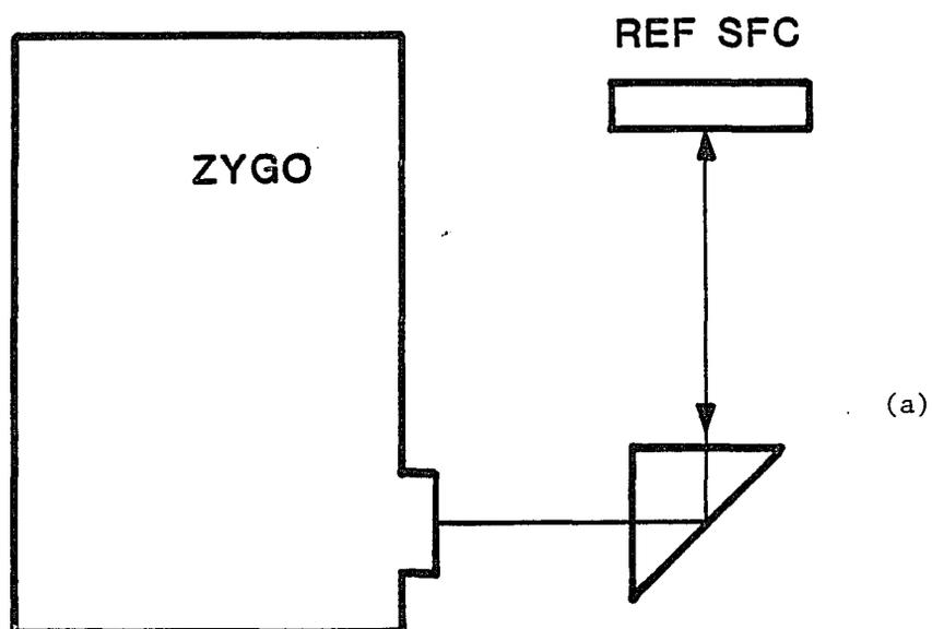
Fig. 25. Zygo interferometer test of cube half.
