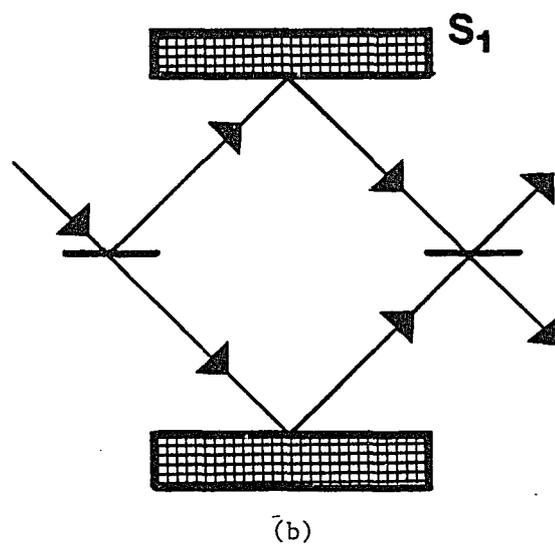
Fig. 8. Mach-Zehnder and Mirau interferometers.
