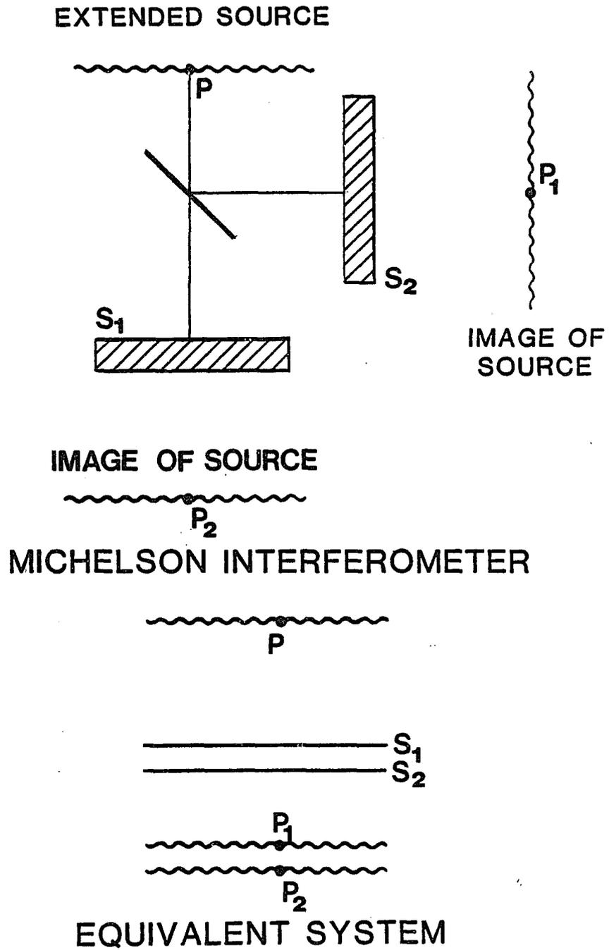
Fig. 4. Simplified Interferometer.
