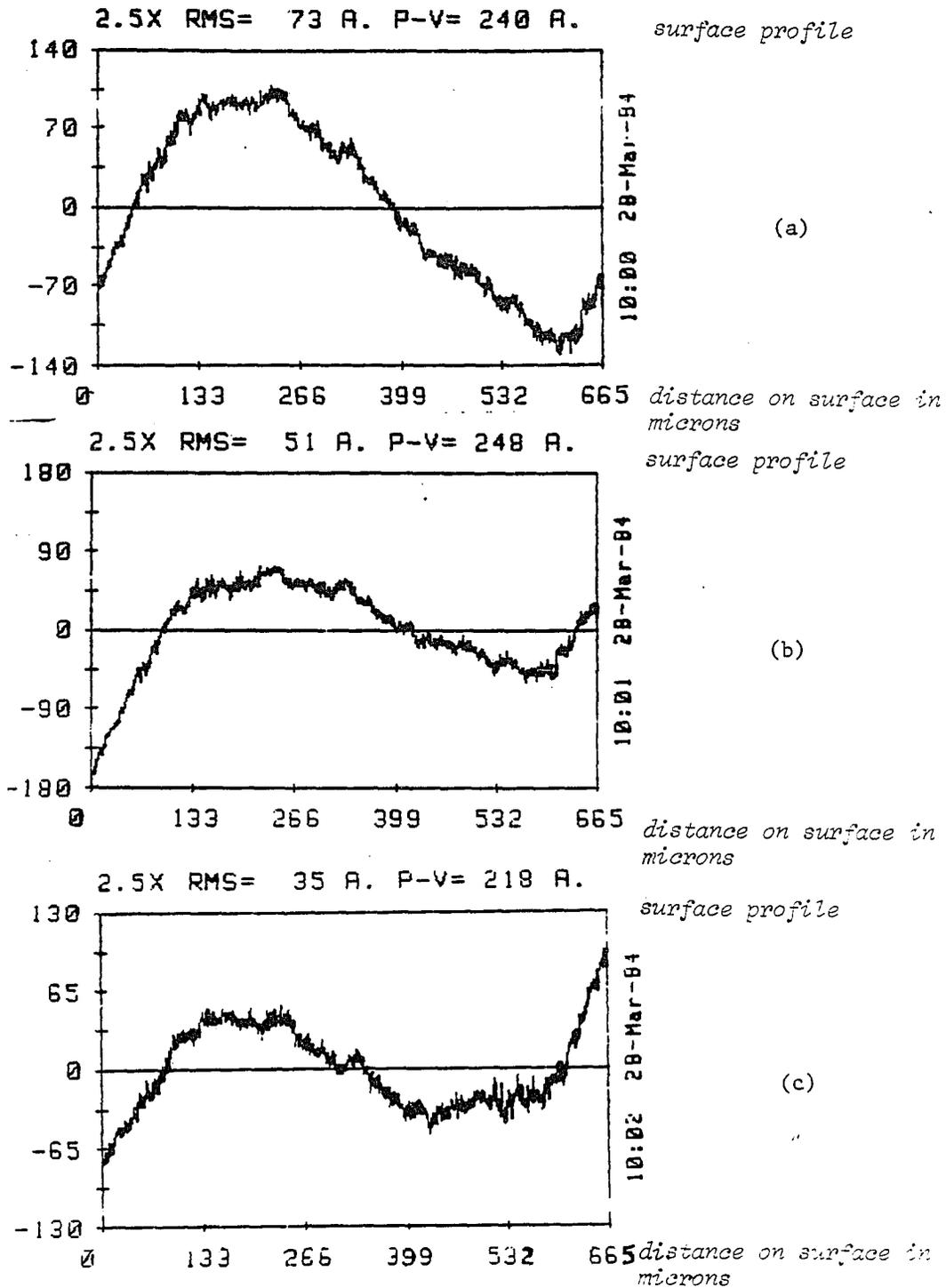
Fig. 21. Profile data showing beamsplitter induced profile error.
