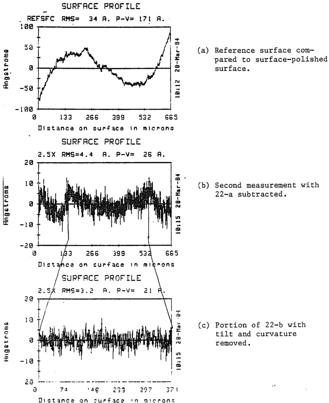
Fig. 22. Profile data showing reference subtraction technique.
