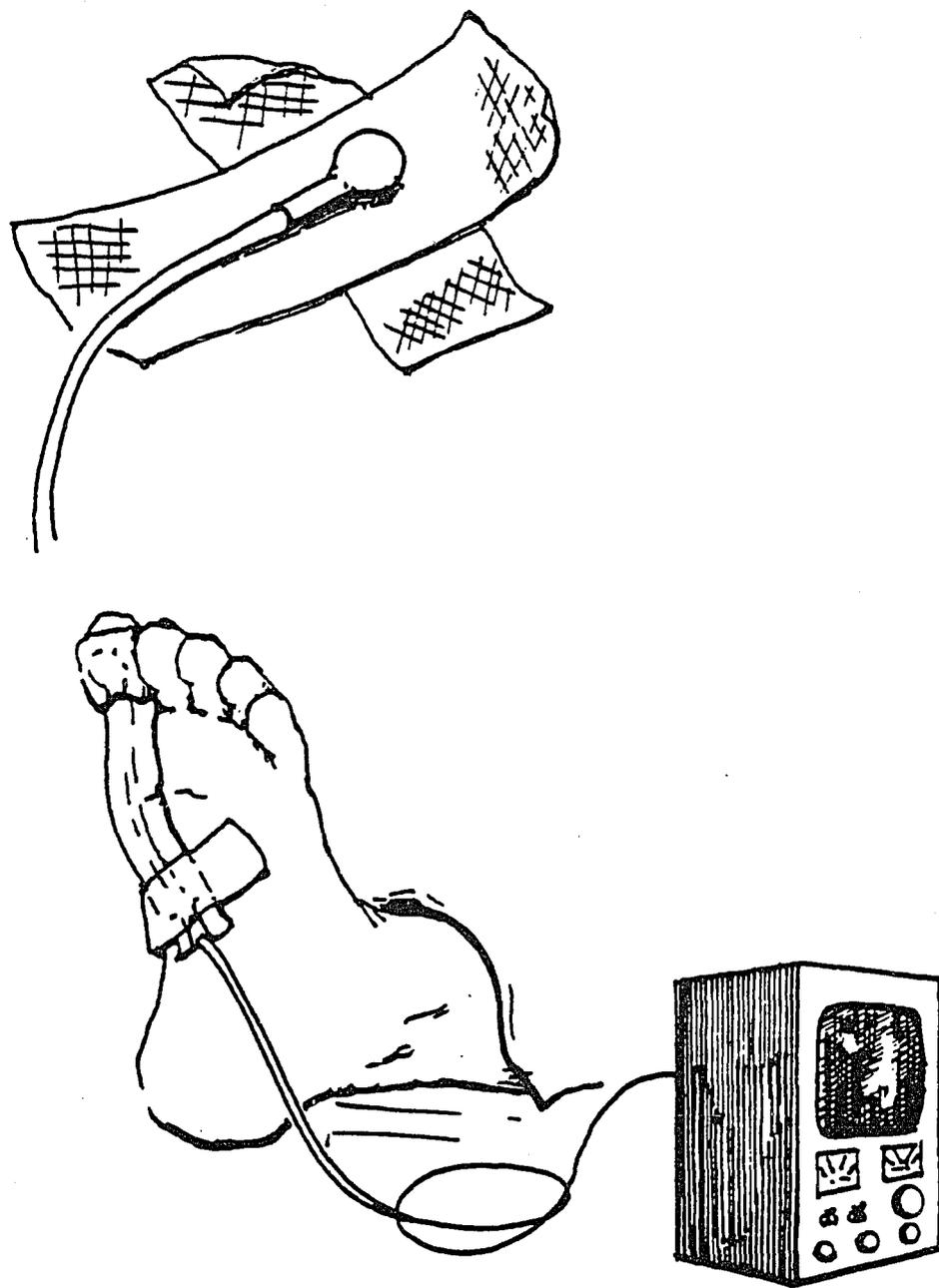
Figure 2. Temperature Probe Application Procedure
