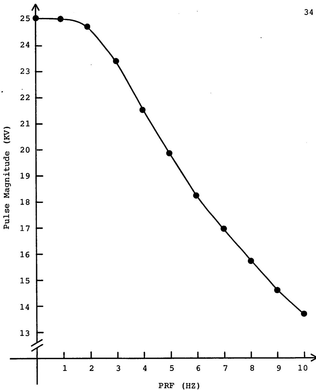
Figure 4.2. Pulse magnitude as a function of the pulse repetition frequency for the matched termination.
