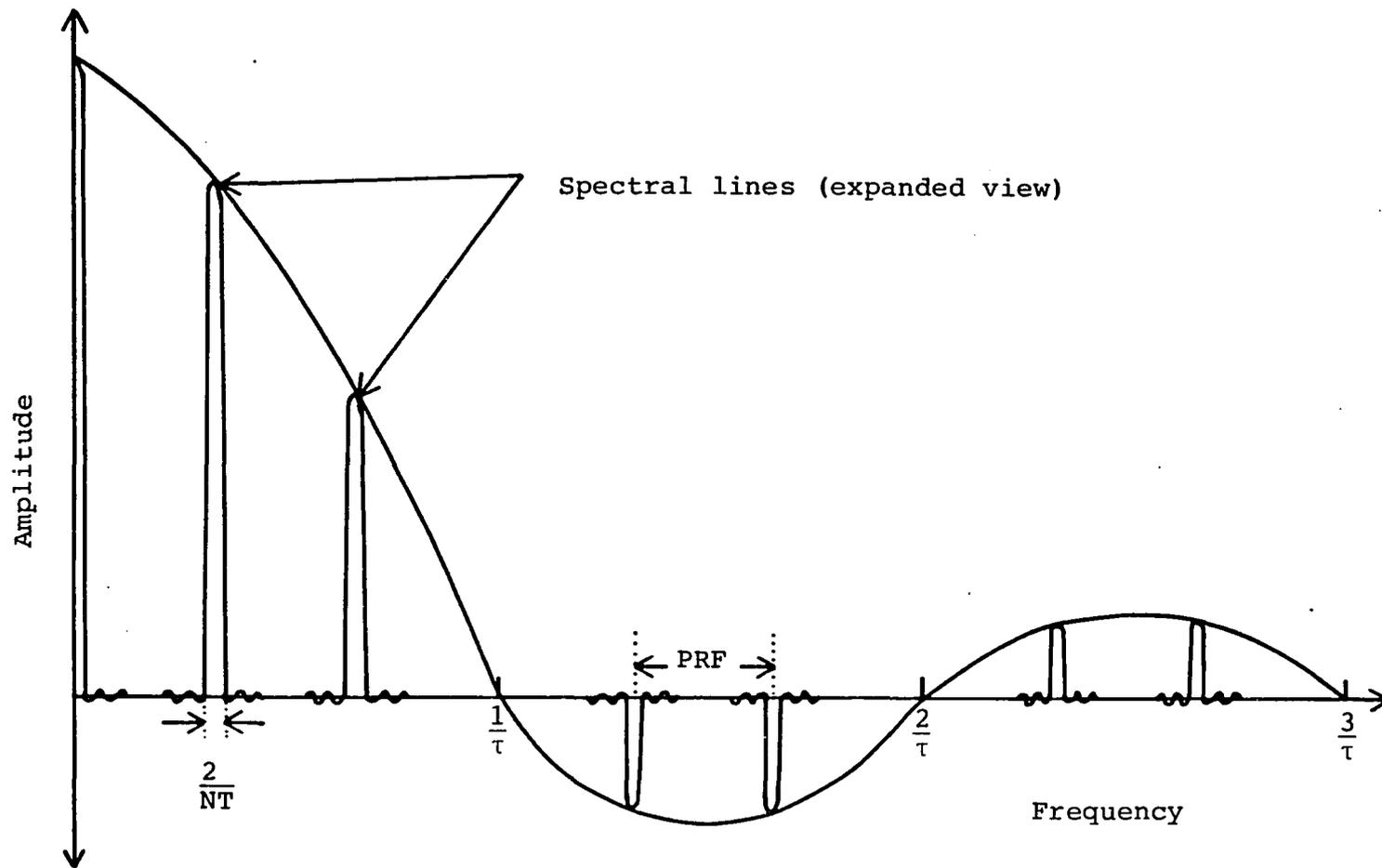
Figure 4.9. Fourier transform for a rectangular train of  $N$  DC pulses.
