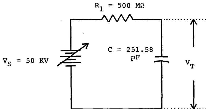
Figure 4.1. Pulse system charging circuit.
