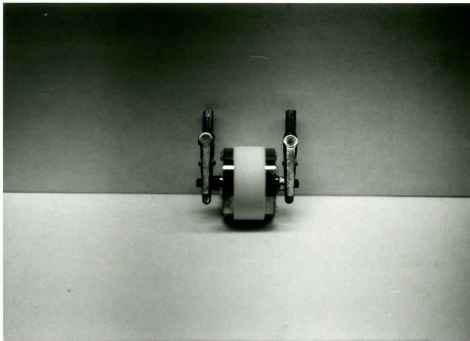
Figure 3.1. Cell holder with attached measurement clips.
