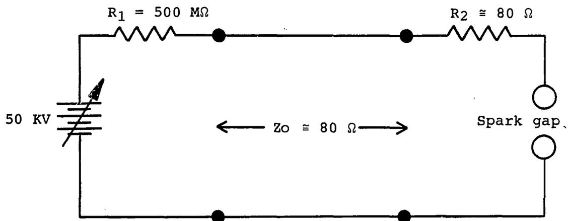
Figure 2.5. Abbreviated pulse system circuit.
