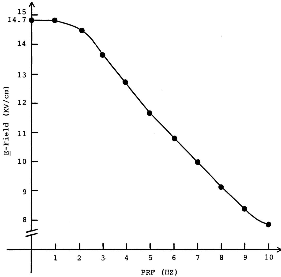
Figure 5.1. Electric field within the cell holder versus obtained PRF.
