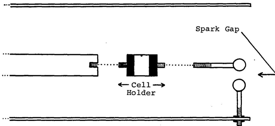
Figure 3.4. Transmission line with cell holder and spark gap.
