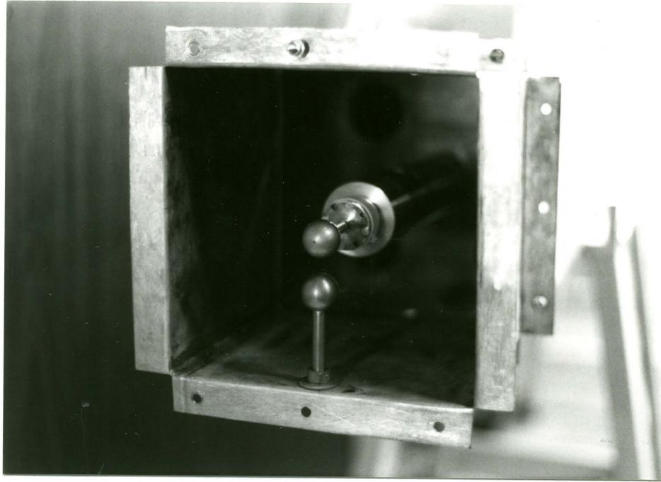
Figure 1.2. Pulse system front end, including the parallel-plate cell holder.
