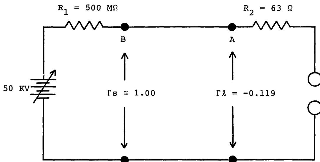
Figure 4.4. Mismatched pulse system circuit with discontinuities at points A and B.
