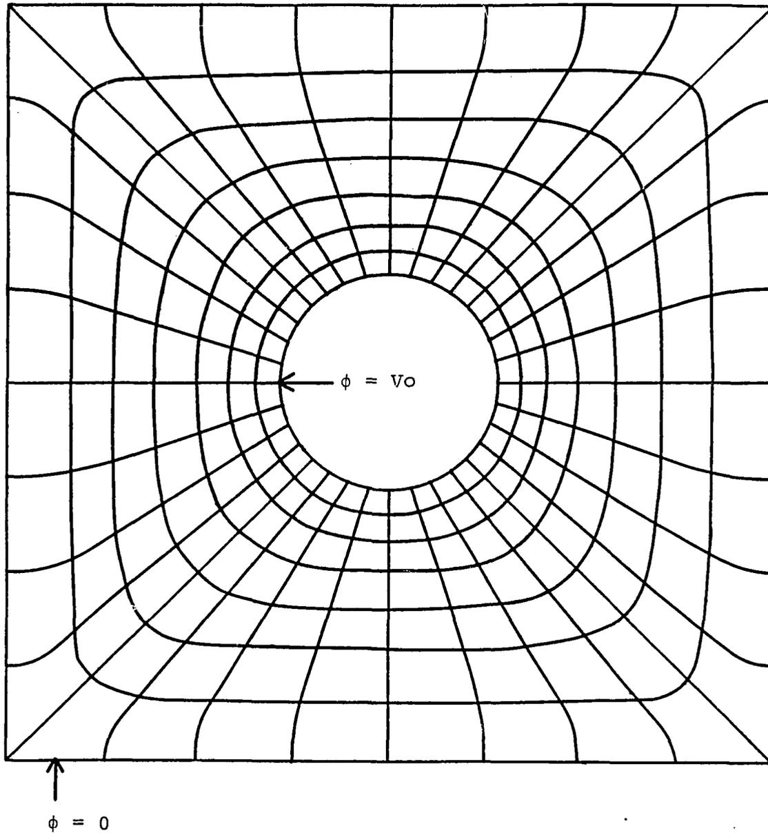
Figure 2.2. Transmission line cross-section, including E-field and equipotential lines.
