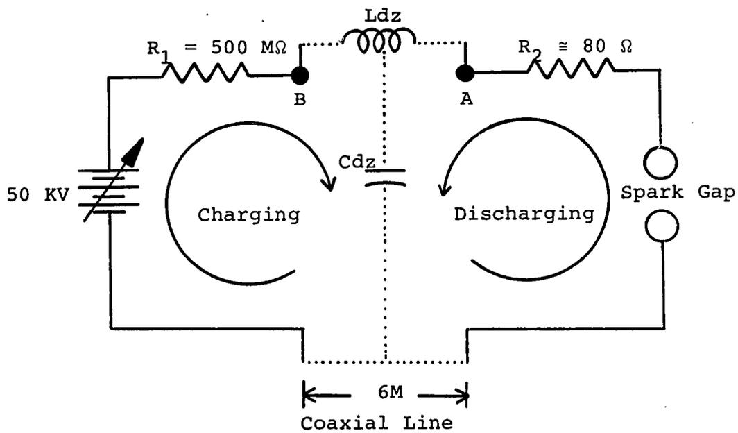
Figure 2.1. Equivalent pulse system circuit.
