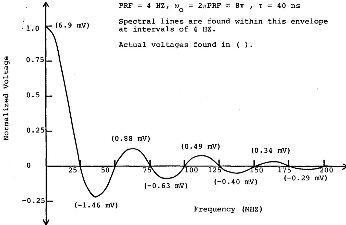
Figure 4.8. Spectral envelope for the matched termination (ideal case).
