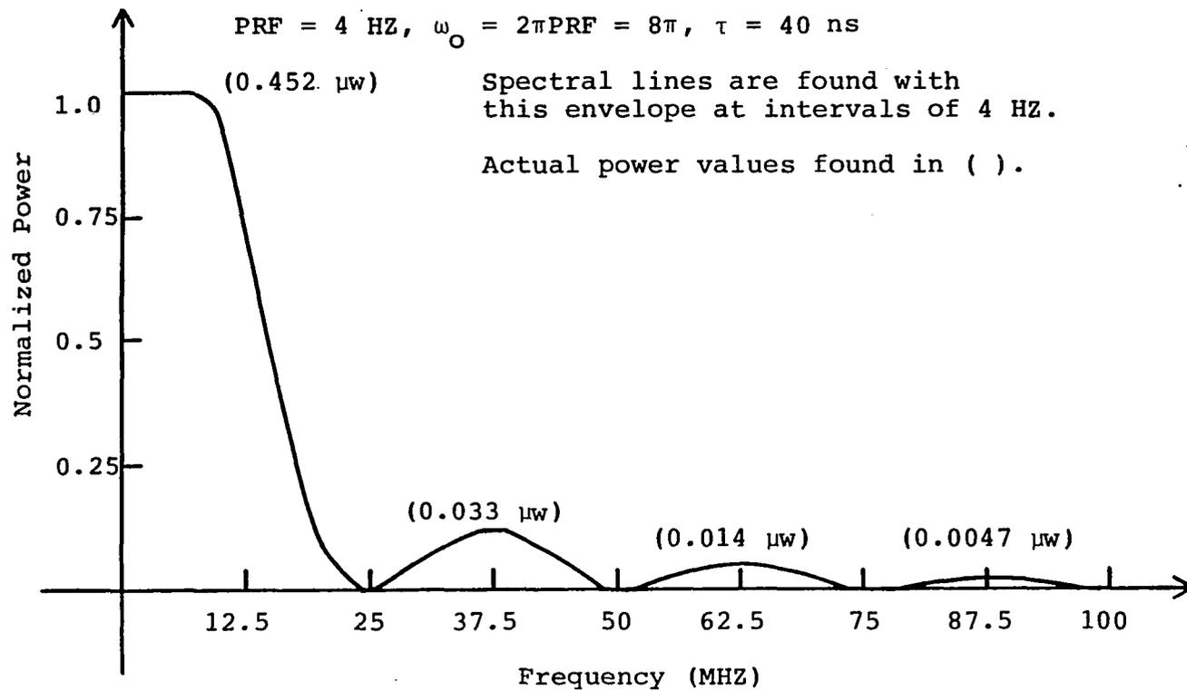
Figure 4.10. Power spectrum envelope for the mismatched termination (actual case).
