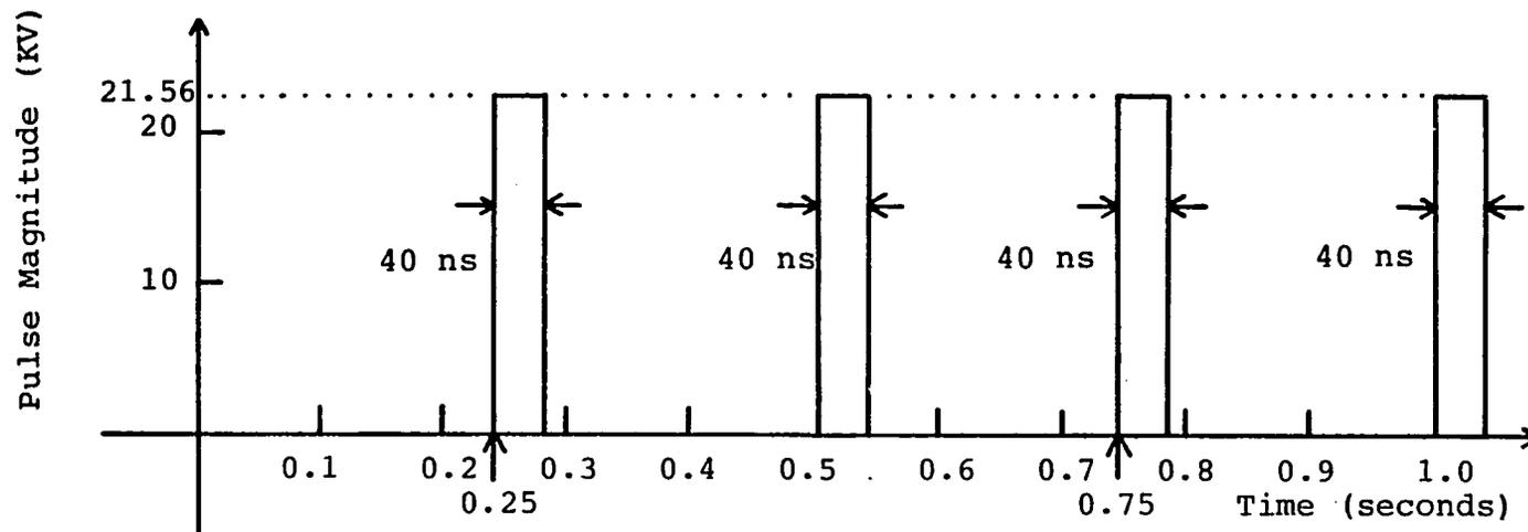
Figure 4.3. Transmission line voltage,  $V_T$ , and pulse magnitude as a function of time.
