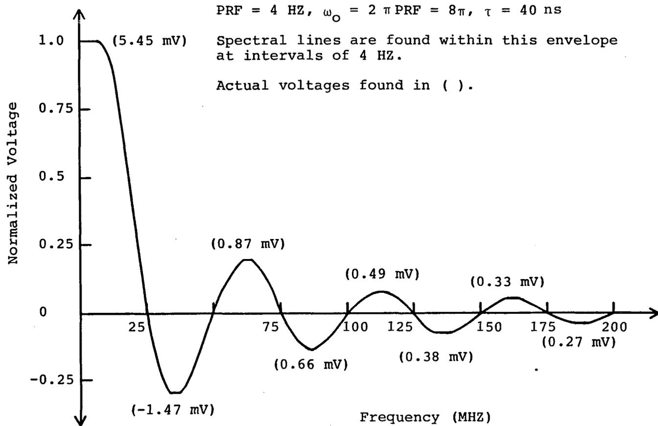
Figure 4.6. Spectral envelope for the mismatched termination (actual case).
