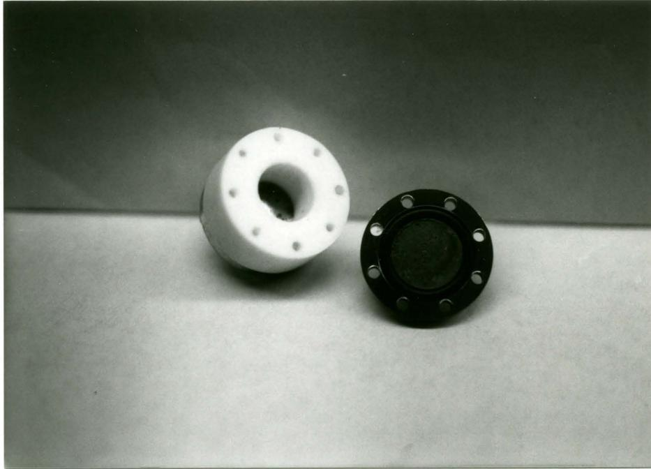
Figure 3.3. Cell holder with one plate removed, exposing the teflon disk.
