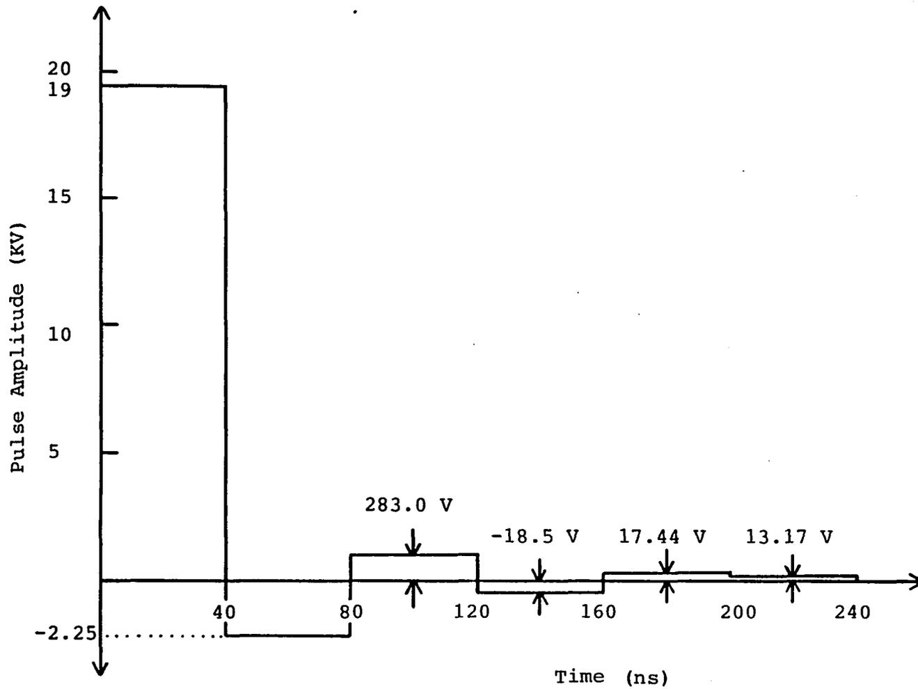
Figure 4.5. Pulse amplitude versus time for the mismatched termination.
