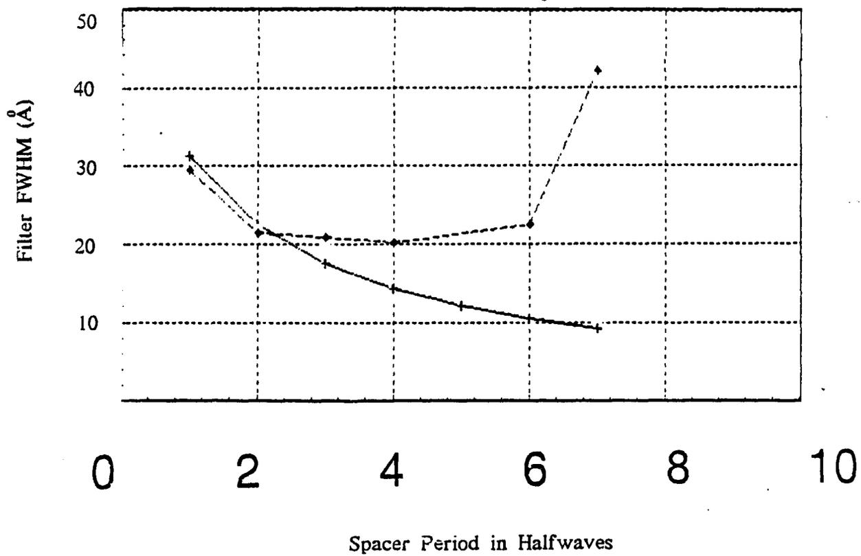
Figure 5.5 A comparison of the theoretical filter FWHM (solid line) with the experimentally observed halfwidth
