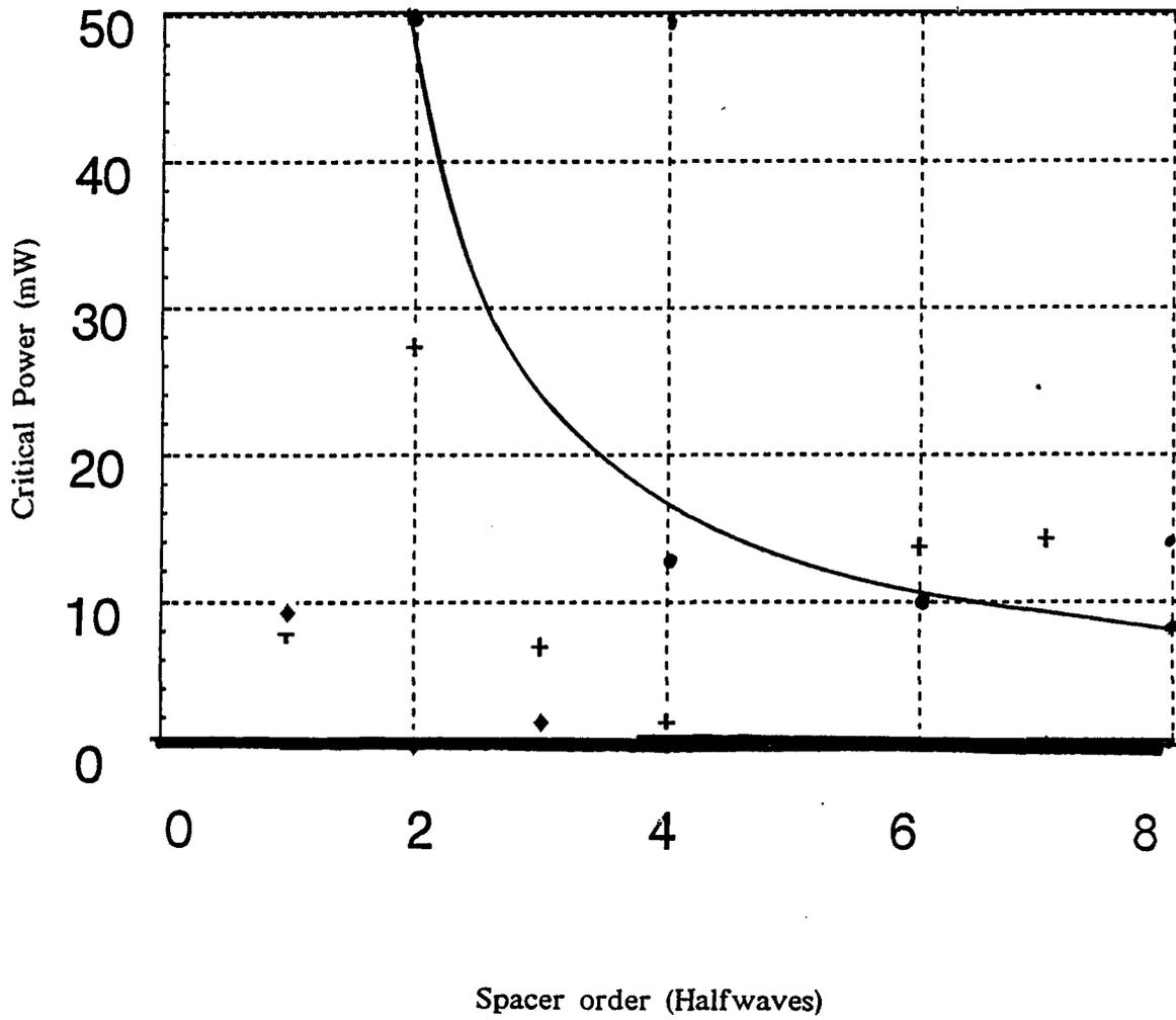
Figure 5.8 *The observed minimum critical power as a function of spacer order.*
