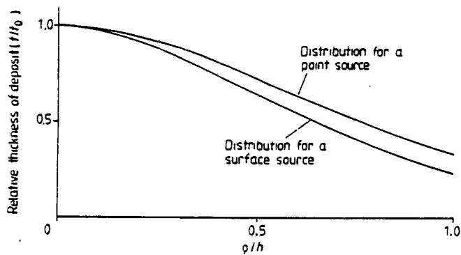
**Figure 4.2** *The thickness distribution calculated for a point source and a directed surface source* (Macleod, 1986)
