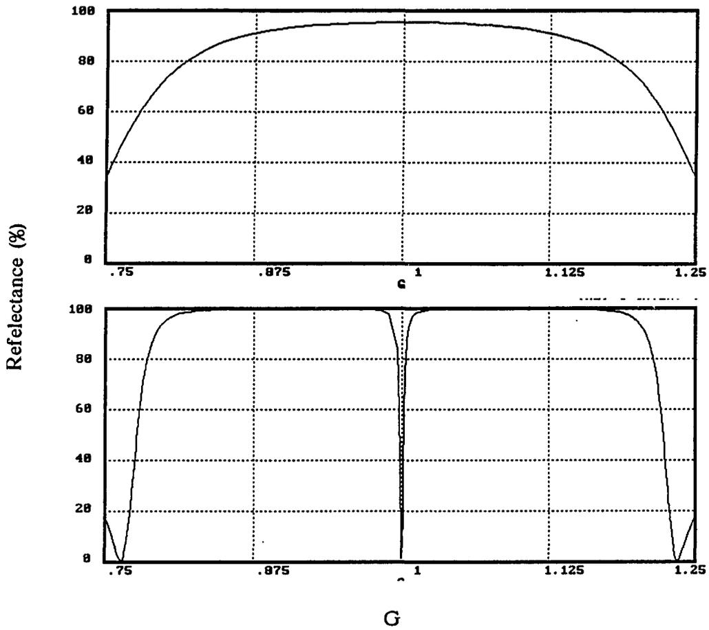
Figure 3.6 *The Reflectance of a NBF compared to that of its mirrors*
