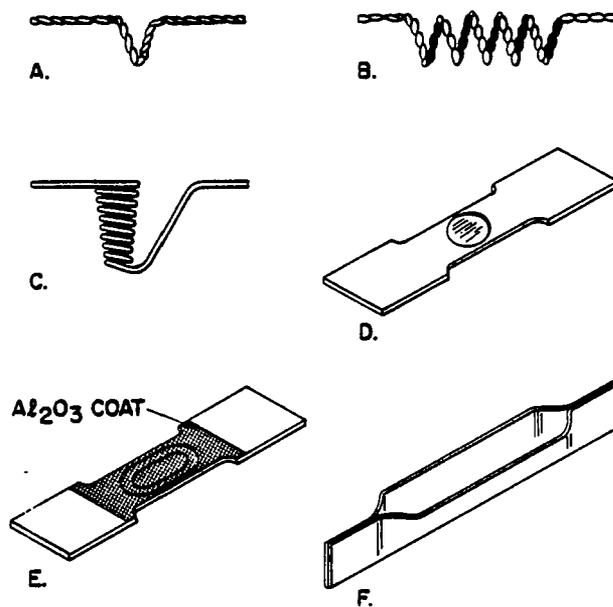
**Figure 4.5** Several common types of resistive sources used in thin film deposition: (a) Hairpin; (b) coiled filament; (c) coiled basket; (d) dimple; (e)  $\text{Al}_2\text{O}_3$  coated dimple; (f) canoe.
