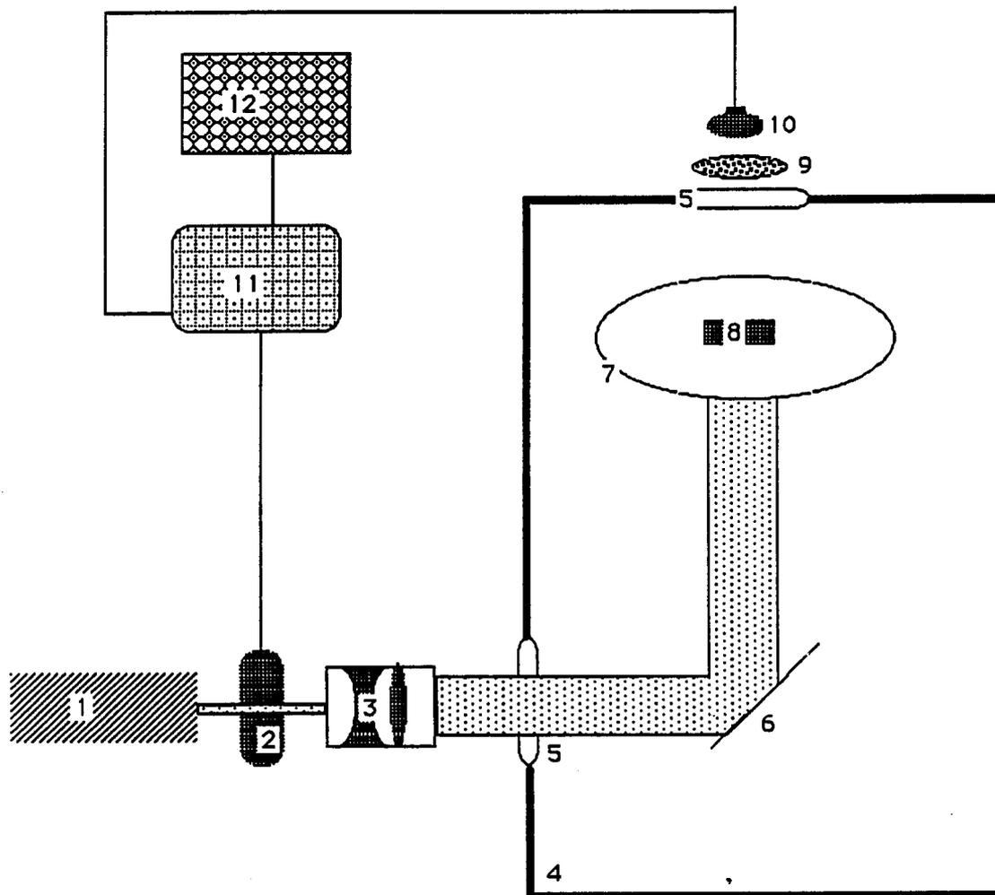
(1) air cooled Ar<sup>+</sup>ion laser ( $\lambda=5145\text{\AA}$ ); (2) Beam Chopper; (3) beam expander; (4) vacuum chamber wall; (5) system window; (6) folding mirror (7) substrate holder; (8) substrate; (9) 5145Å Filter; (10) Si Pin detector; (11) Lock-in Amplifier; (12) Strip chart recorder.
