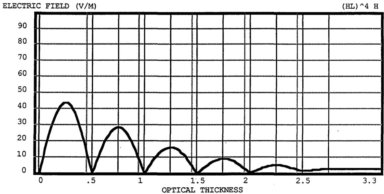
Figure 2.5 *Electric field in a mirror*, an all dielectric multilayer design as figure 2.4, normalized to  $1 \frac{\text{watt}}{\text{M}^2}$  incident for  $G=1$ .
