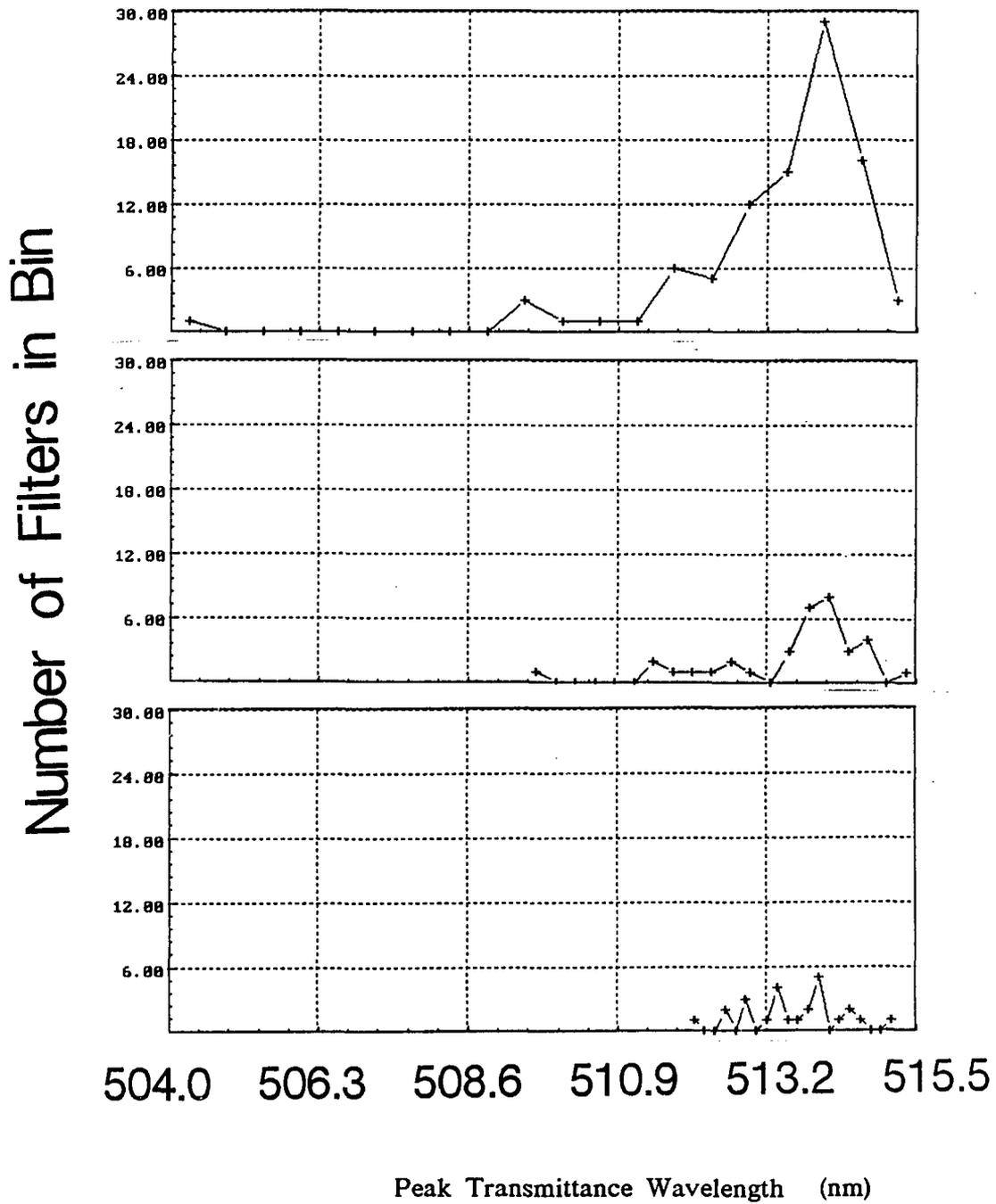
Figure 5.6 Histogram of the low power transmittance peak for: (a) all filters (b) stable filters  $p=4$ ; (c) stable filters  $p=5$ .
