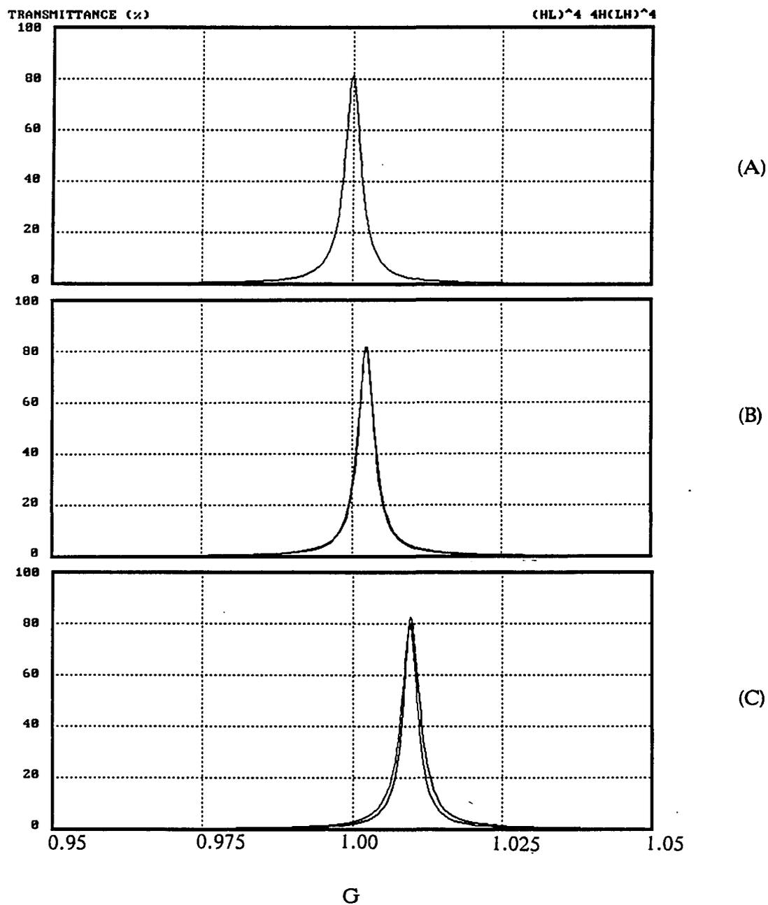
Figure 2.7 The change in transmittance for small change in angle.
