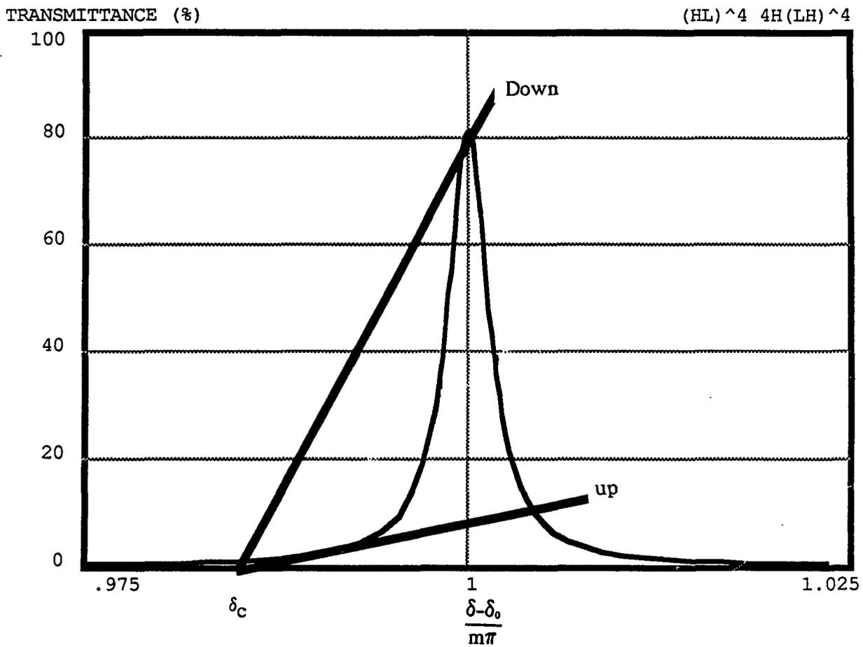
The Switch up (up) and switchdown (down) load lines, ( $I_t/I_i$ ) for a standard Fabry Perot filter design. The point where the two lines meet at the phase axis is  $\delta_c$  the initial detuning.
