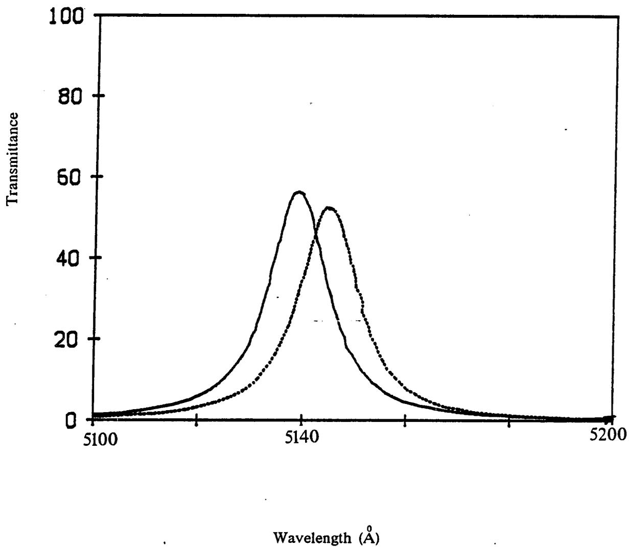
Figure 5.2 *Typical linear performance of a filter* Illustrating the variation in transmittance and halfwidth of the sampled points.
