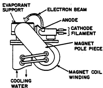
**Figure 4.6** A bent beam electron beam source
