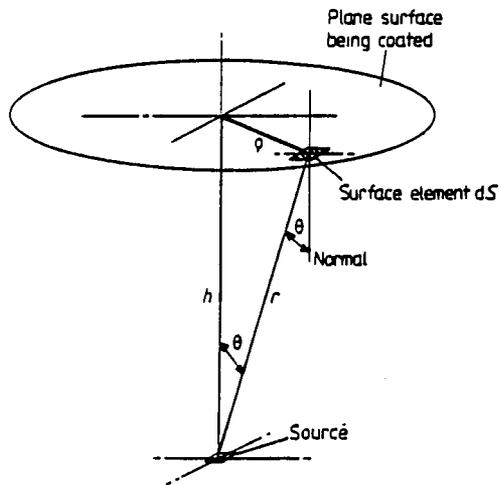
**Figure 4.1** *The source-substrate configuration for a flat plate substrate.*
