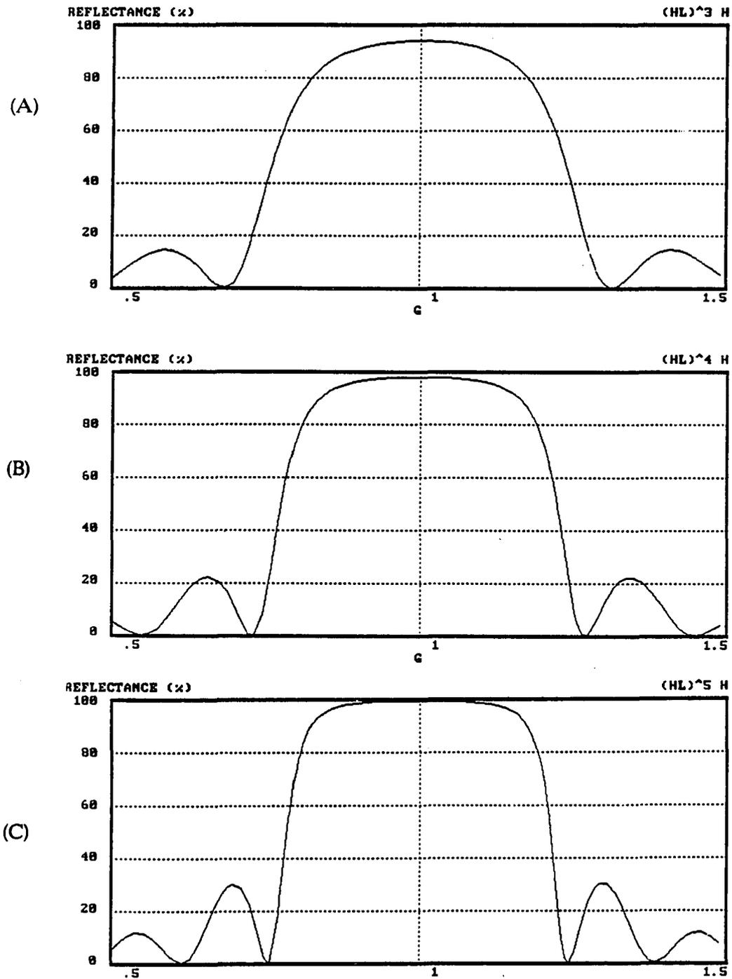
Figure 2.3 The reflectivity of a multilayer stack ;
