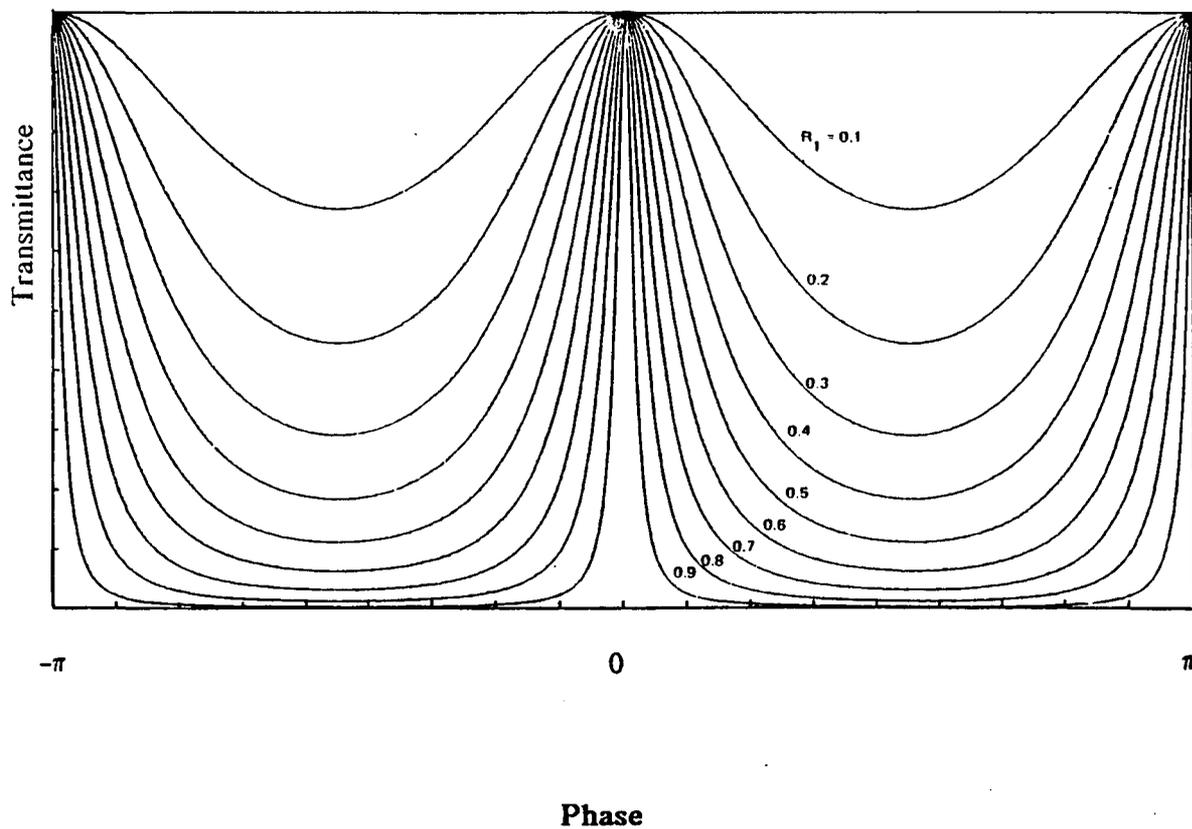
**Figure 2.6** *The Transmittance function of a Fabry-Perot Narrow Band Filter as a function of phase for various reflectivities. The cavity is assumed lossless.*
