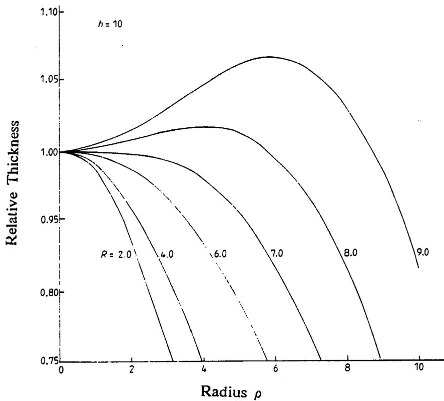
Figure 4.3 The radial distribution of material for a rotating flat plate for various radial source distances (Macleod, 1986)
