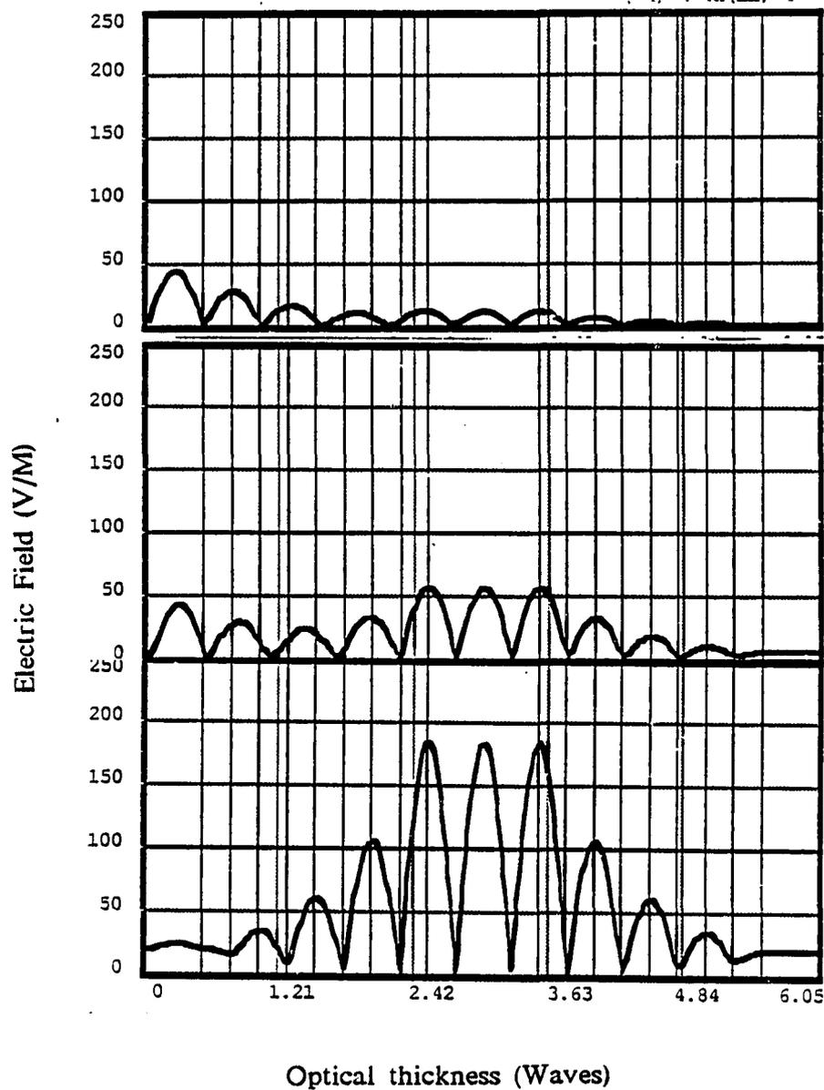
**Figure 3.5** *The electric field in a single cavity filter*
