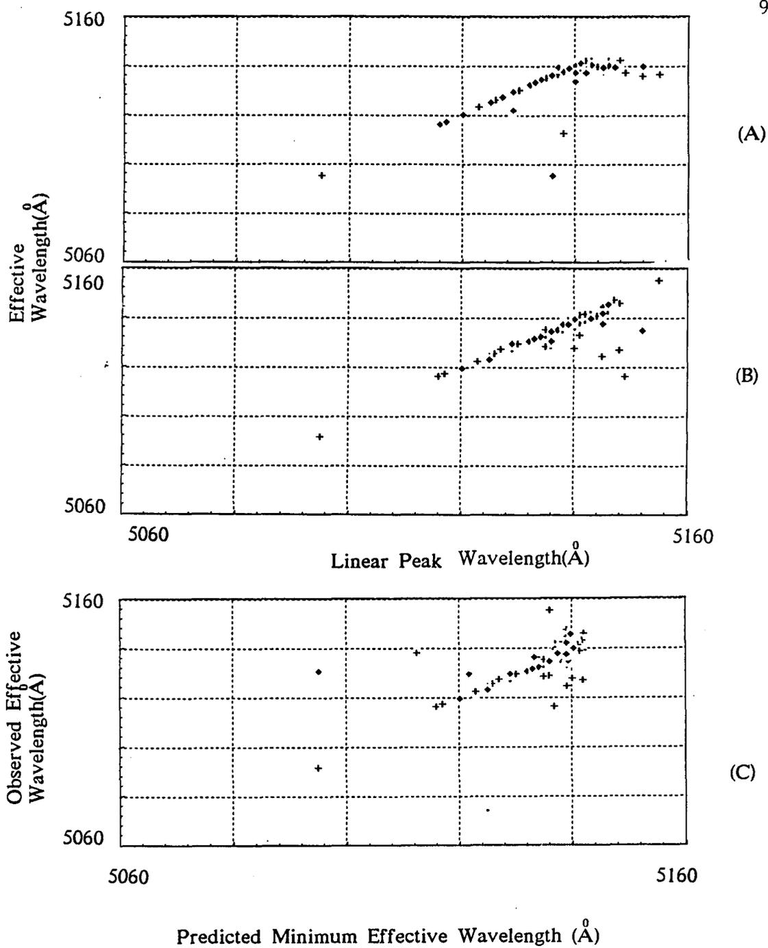
Figure 5.7 The effective nonlinear peak as a function of the linear peak. (a) The behavior predicted from the halfwidth and initial wavelength. (b) The observed behavior (c) The observed compared with the predicted.
