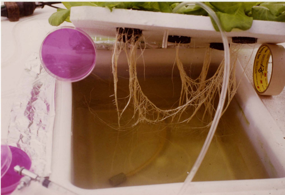
Figure 2. Method used for sampling the nutrient solution for the presence of zoospores.
