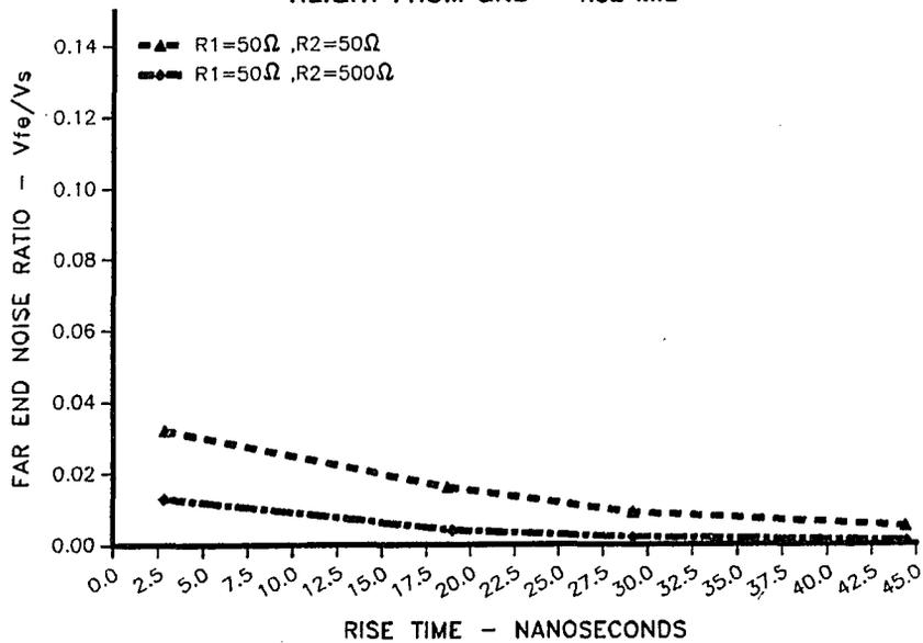
Figure 4.20 Stripline Coupled Noise Ratio vs. Signal Rise Time
