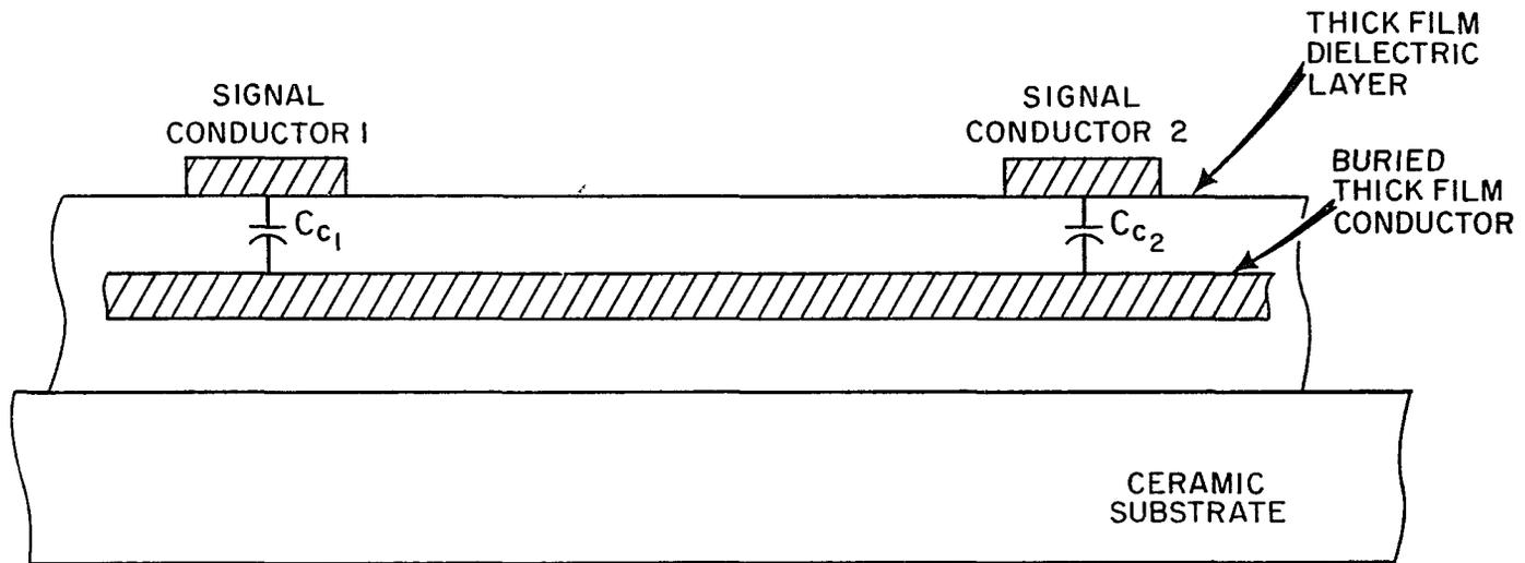
Figure 2.4 Example of Conductive and Capacitive Noise Coupling in a Multilayer Hybrid Circuit
