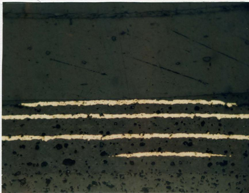
b. Cross Section of a Multilayer Circuit (200X)
