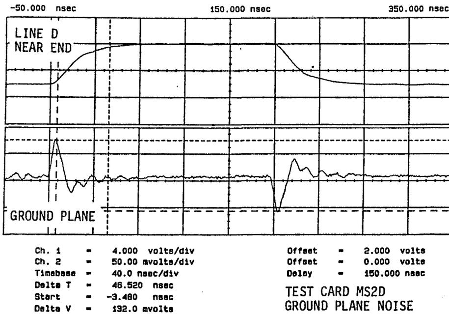
Figure 4.17 Ground Plane Noise on a Multilayer Card
