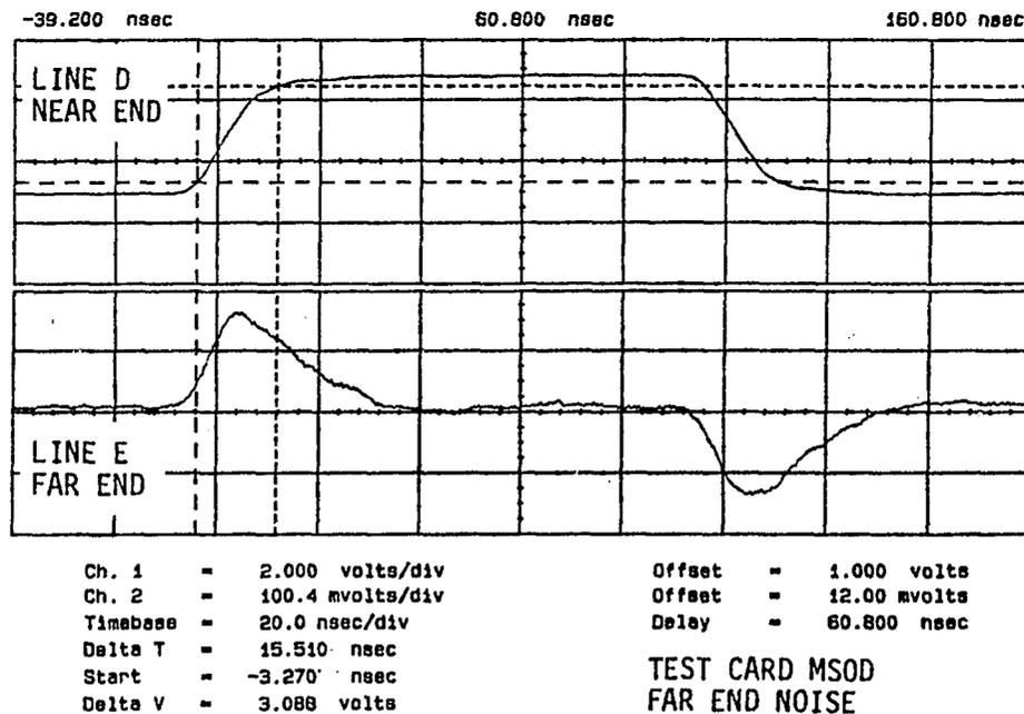
Figure 4.10 Crosstalk on a Single Layer Card
