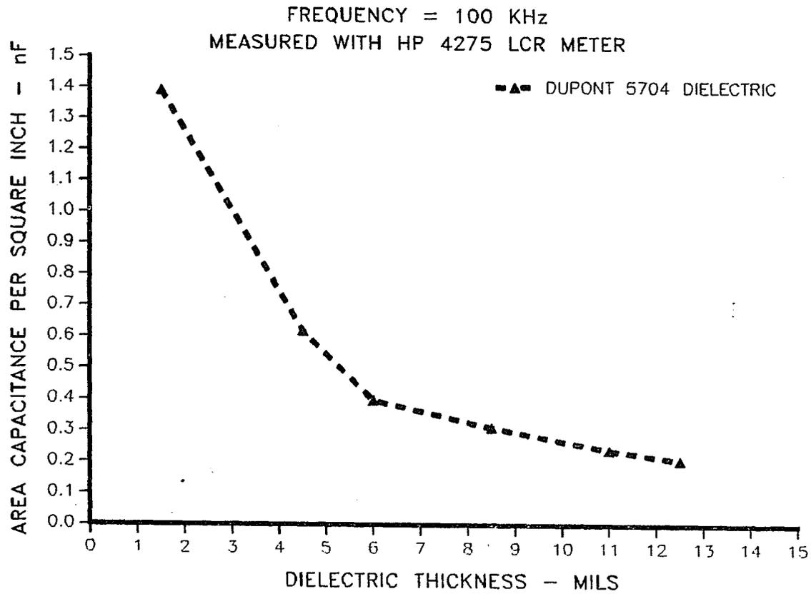
Figure 4.1 Area Capacitance vs. Dielectric Thickness
