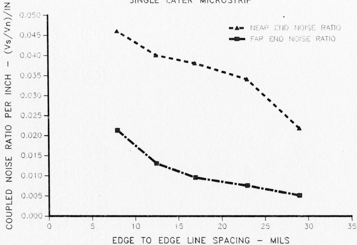
Figure 4.13 Coupled Noise Ratio vs. Line Spacing
