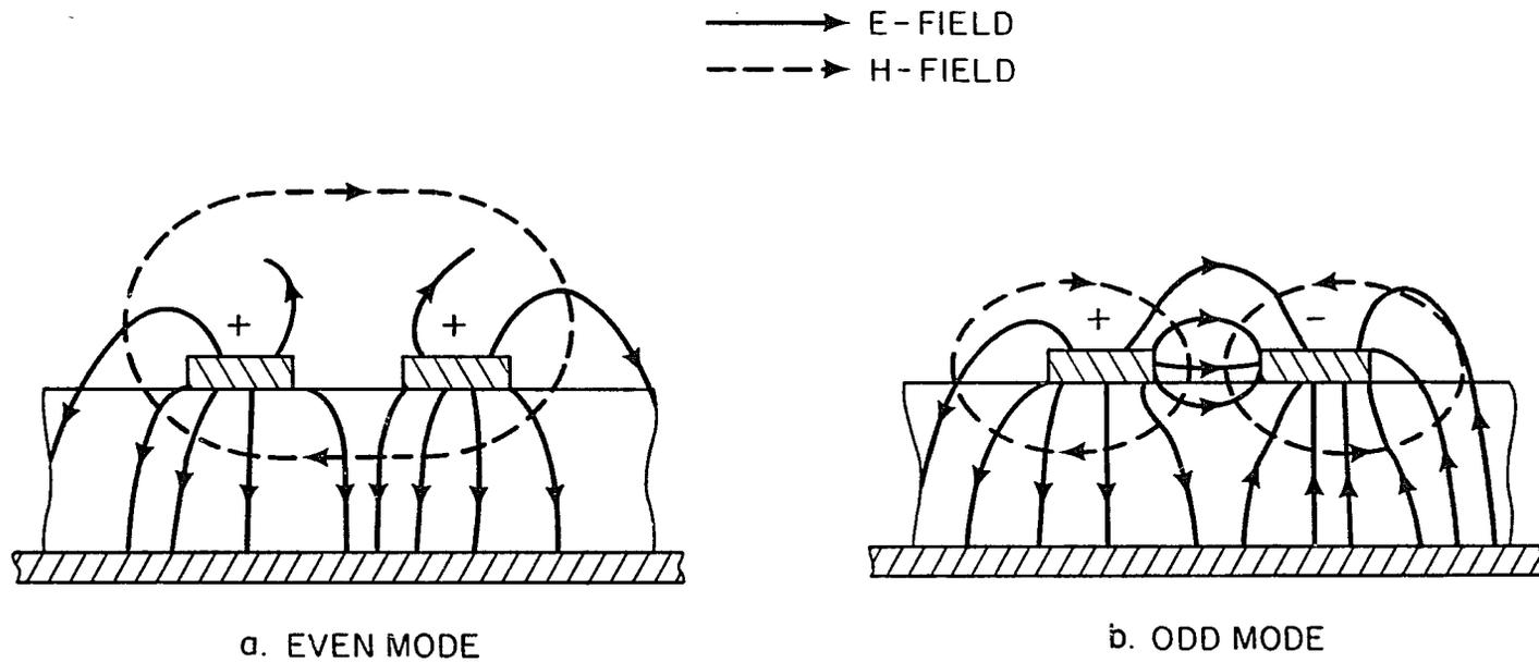
Figure 2.1 Electromagnetic Field Interactions in Parallel Coupled Microstrip Lines
