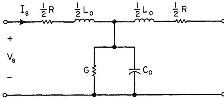
Figure 3.2 Lumped Parameter Transmission Line Model
