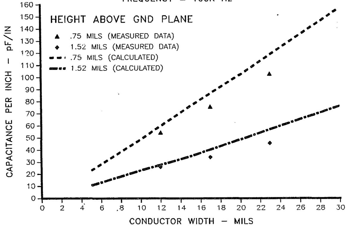
Figure 4.3 Stripline Line Capacitance
