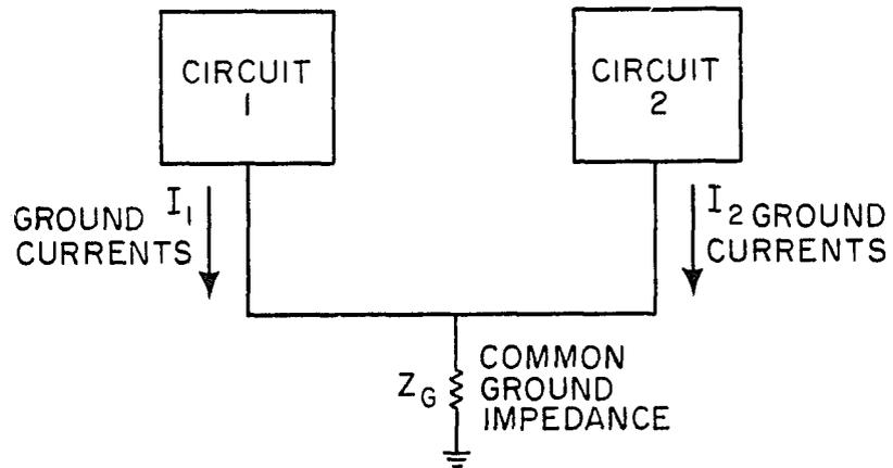
Figure 2.3 Example of Conductive Noise Coupling
