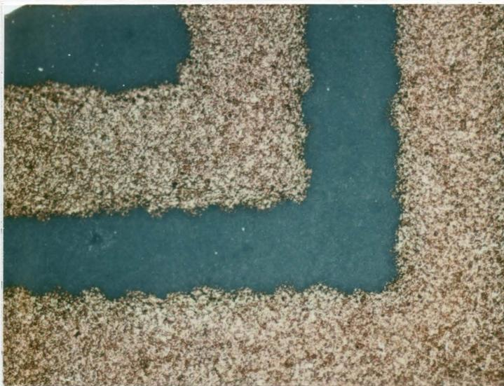
a. Screened Thick Film Conductors (100X)
