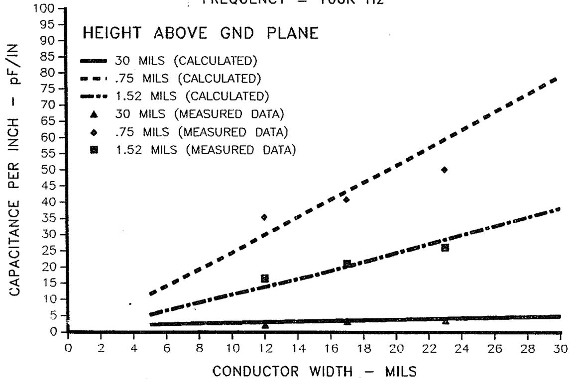
Figure 4.2 Microstrip Line Capacitance
