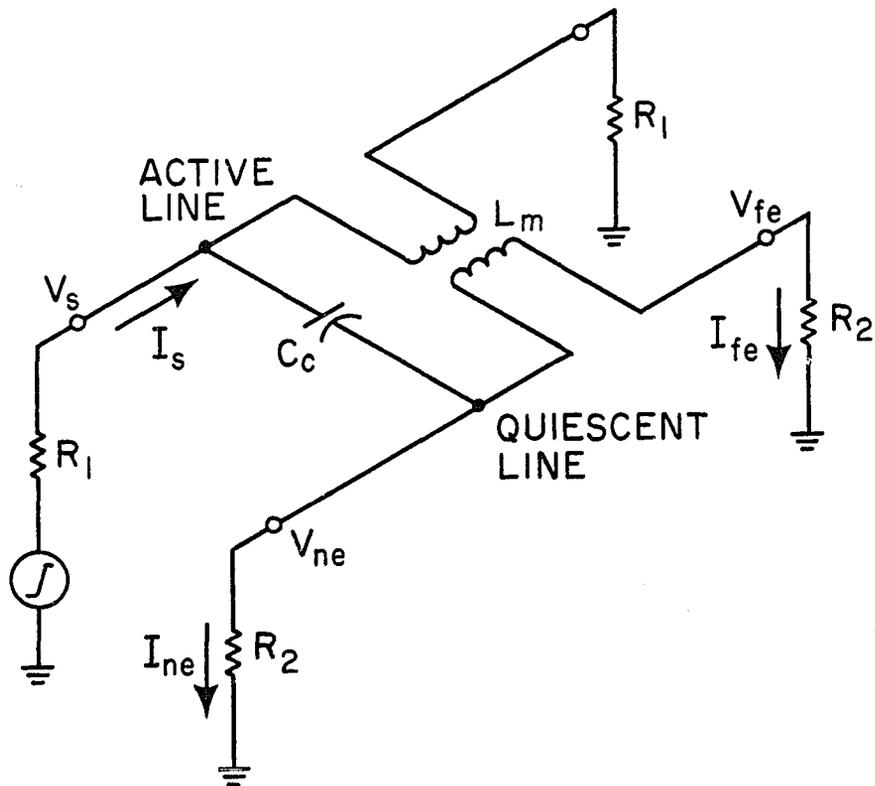
Figure 2.2 Coupled Circuit Model
