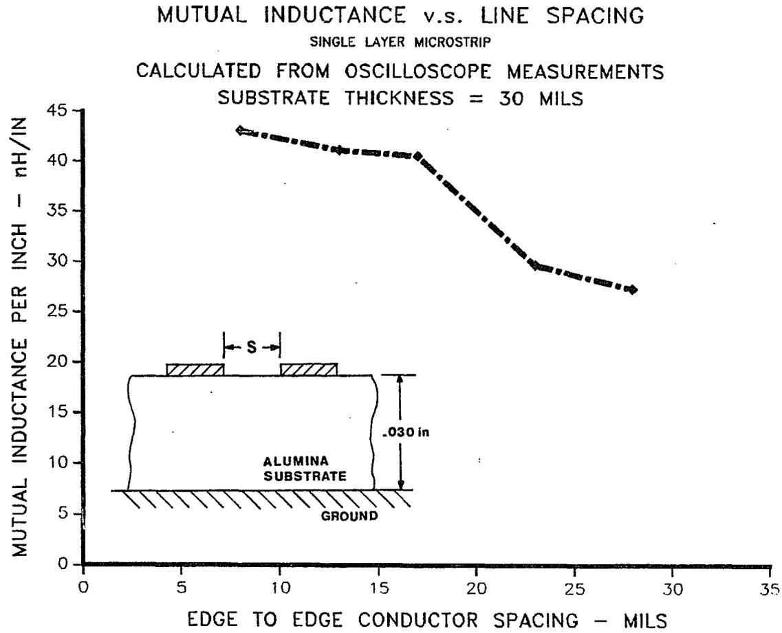
Figure 4.12 Edge to Edge Mutual Inductance vs. Line Spacing
