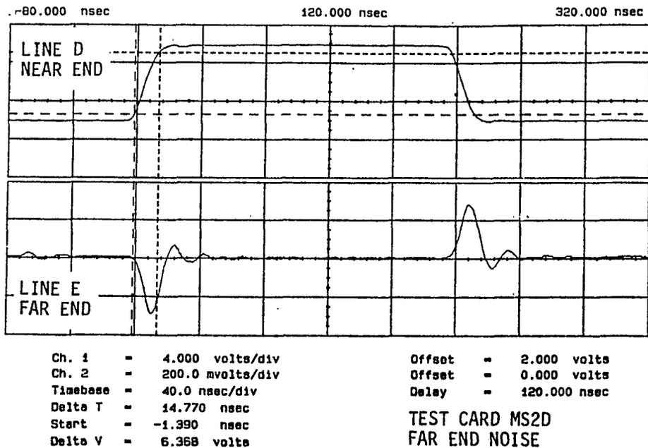
Figure 4.14 Crosstalk on a Multilayer Card
