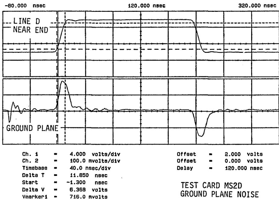
Figure 4.15 Ground Plane Noise on a Multilayer Card
