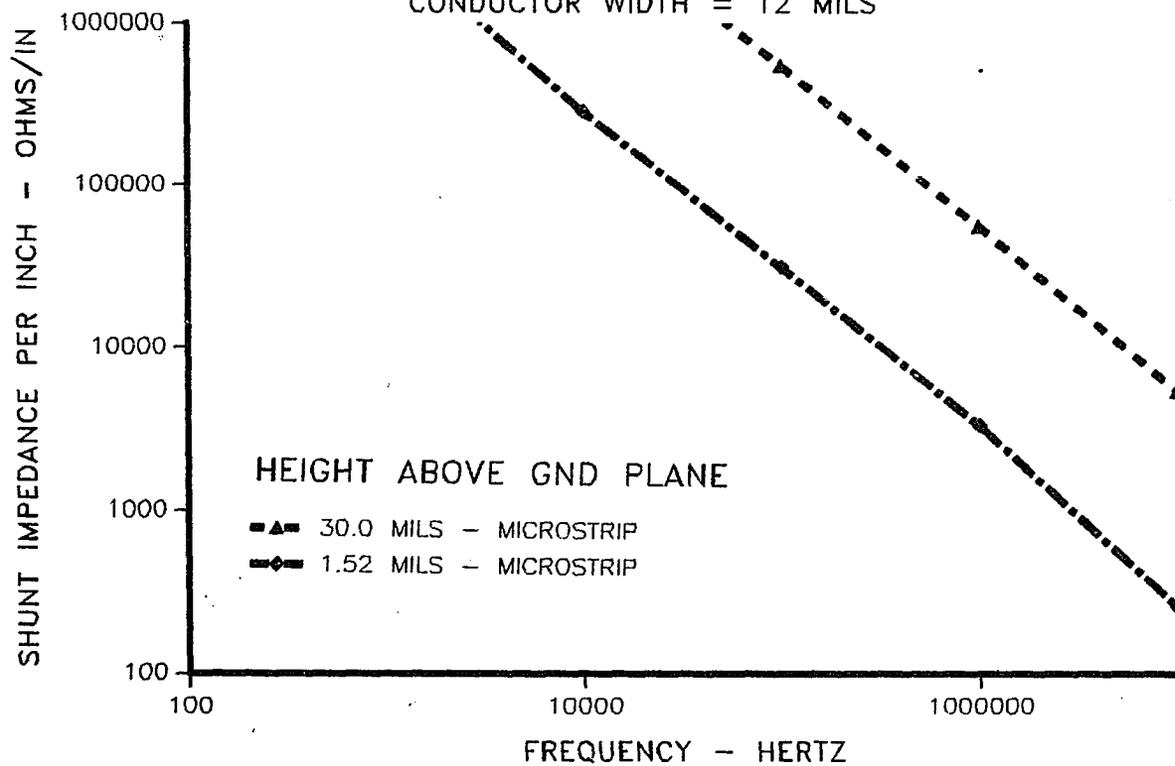
Figure 4.4 Shunt Impedance vs. Frequency
