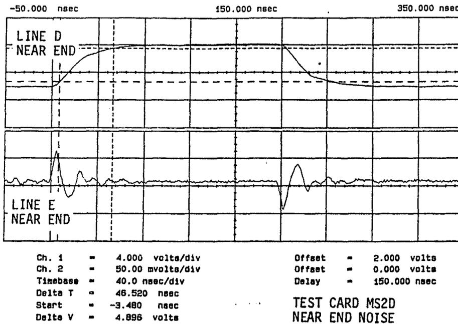
Figure 4.16 Near End Crosstalk on a Multilayer Card
