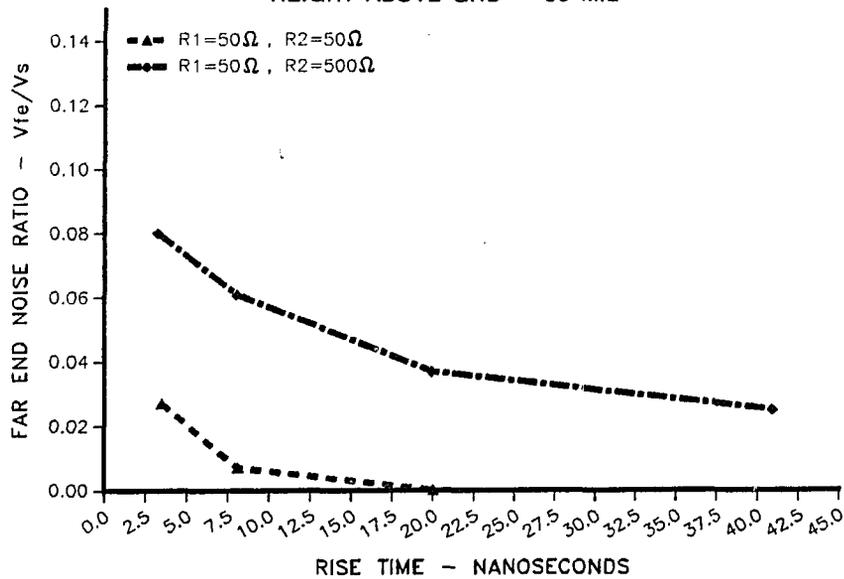
Figure 4.18 Single Layer Microstrip Coupled Noise Ratio vs. Signal Rise Time
