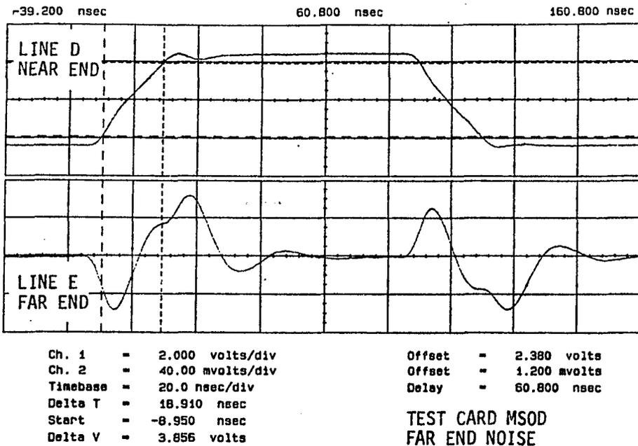
Figure 4.9 Crosstalk on a Single Layer Card (Low Impedance Test Circuit)
