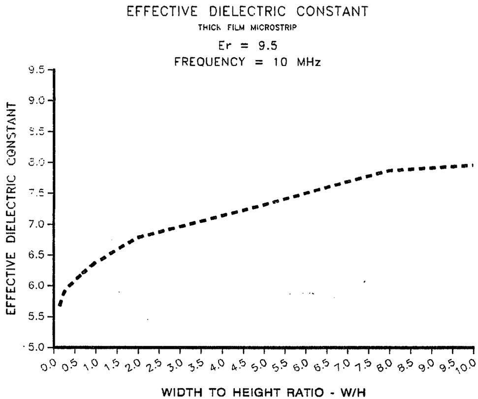
Figure 3.4 Effective Dielectric Constant For Thick Film Microstrips
