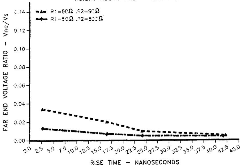
Figure 4.19 Multilayer Microstrip Coupled Noise Ratio vs. Signal Rise Time
