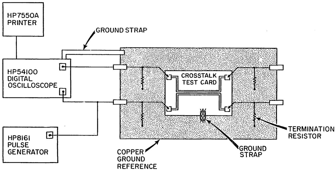
Figure 4.7 Crosstalk Test Setup
