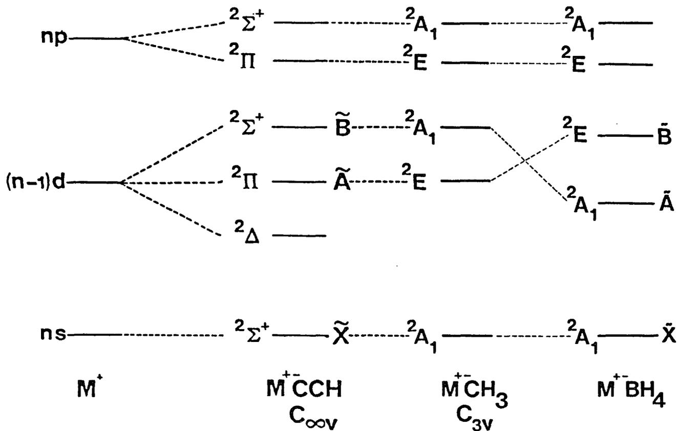
perturbing ligands reduce the symmetry of the metal atomic orbitals and remove some of their degeneracies. The diagram shows the  ${}^2A_1$  and  ${}^2E$  excited state ordering differences in  $MCH_3$  and  $MBH_4$ .
