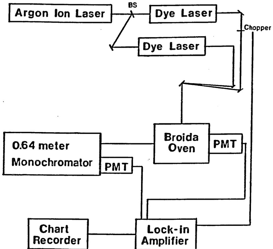
The second type of low resolution experiment, resolved fluorescence, is performed by tuning a dye laser (Coherent 599-01) frequency to a known molecular transition. Emission, or laser induced fluorescence, from the excited molecular state is focussed into a 0.64 m monochromator. The monochromator is scanned to disperse the laser induced fluorescence as a function of wavelength.
