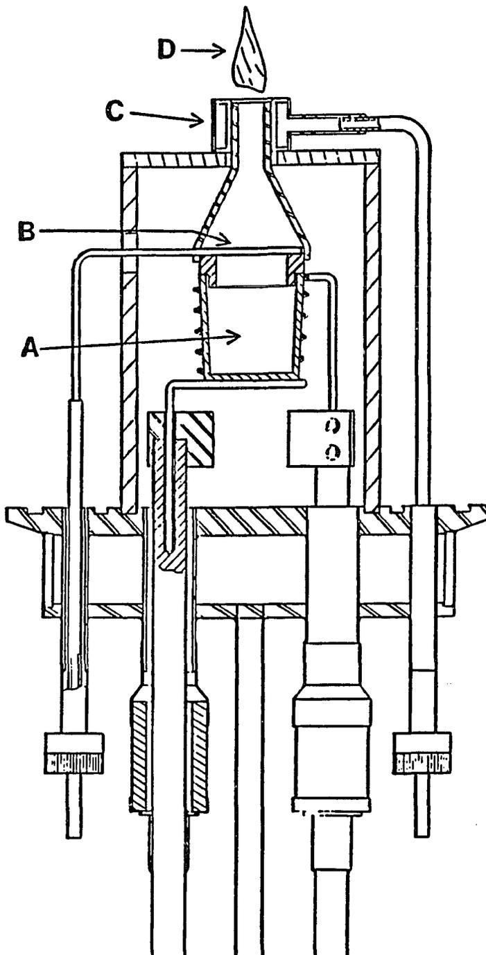
port at the top of the oven is a quartz window at Brewster's angle ( $54^\circ$  for quartz in the visible region). Here, the laser beams are introduced and directed down through the reaction region.
