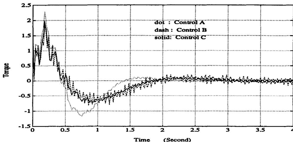
Figure 35: Torques Responses of Three Controllers
