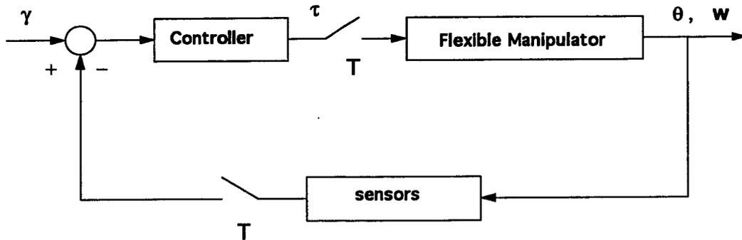
Figure 26: Digital Feedback Control System
