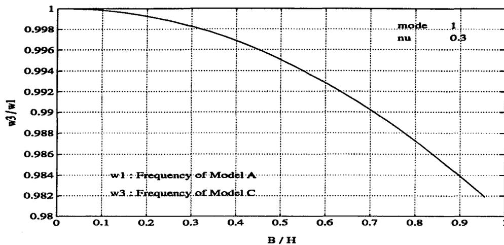
Figure 9: Influence of Shear Deformation: First Order
