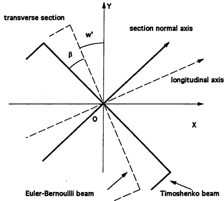
Figure 2: Motion of the Transverse Section
