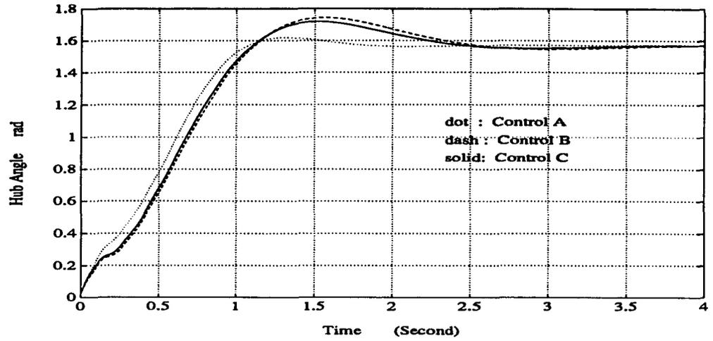
Figure 33: Hub Rotation Responses of Three Controllers
