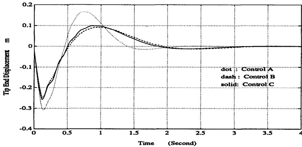
Figure 34: Tip End Displacement Responses of Three Controllers
