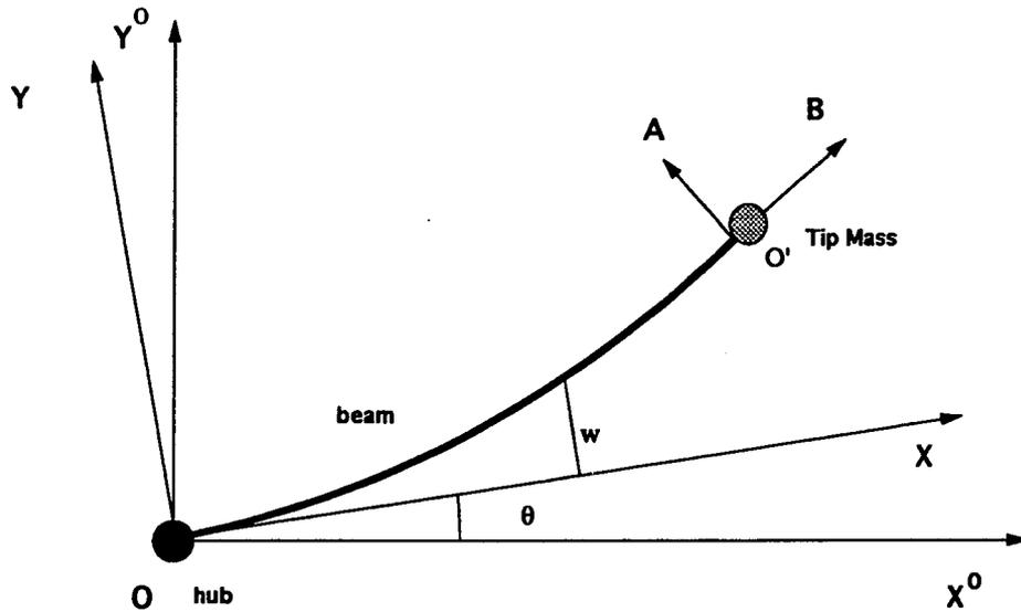
Figure 1: One-Link Flexible Manipulator
