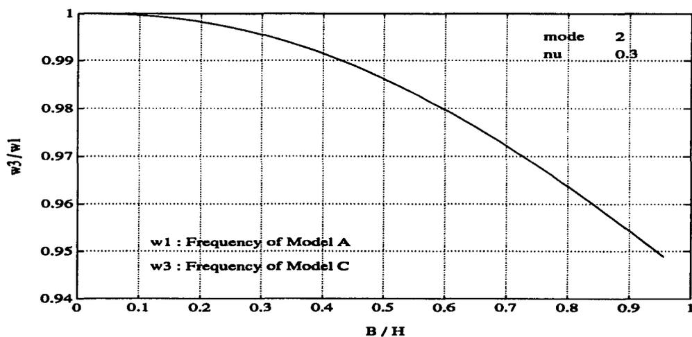
Figure 10: Influence of Shear Deformation: Second Order
