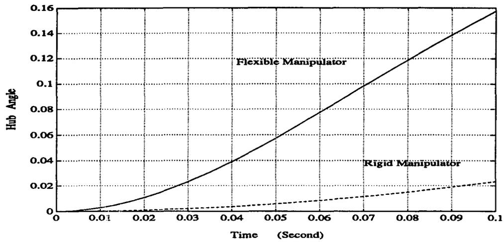
Figure 29: Hub Rotation Response of Pulse Torque ( $t_0 \leq t \leq t_D$ )
