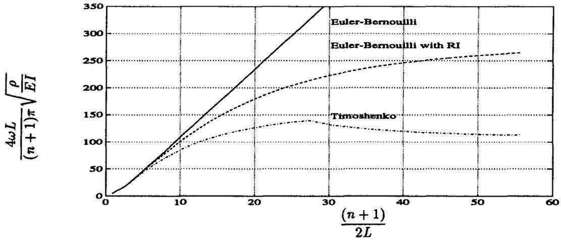
Figure 12: Influence of Rotatory Inertia and Shear Deformation
