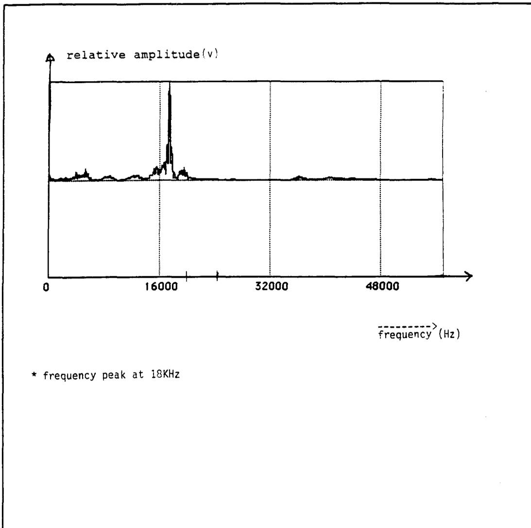
Figure 16 averaged Fast Fourier Transform on multiple heart valve sounds of patient 2.
