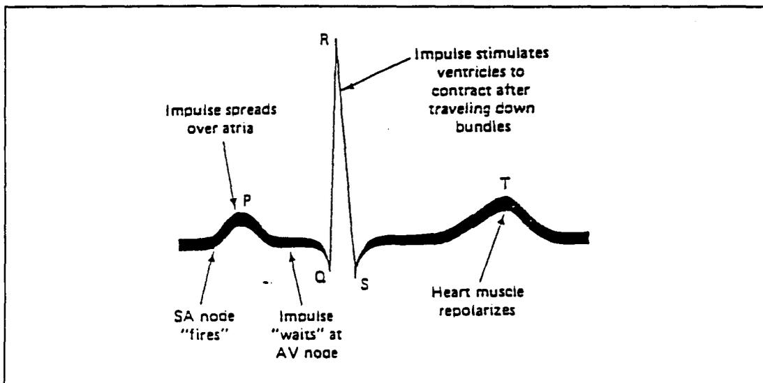
Figure 3 ECG waveform obtained at the body's surface (3)
