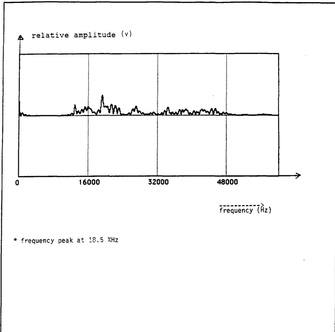
Figure 17 averaged Fast Fourier Transform on multiple heart valve sounds of patient 3.
