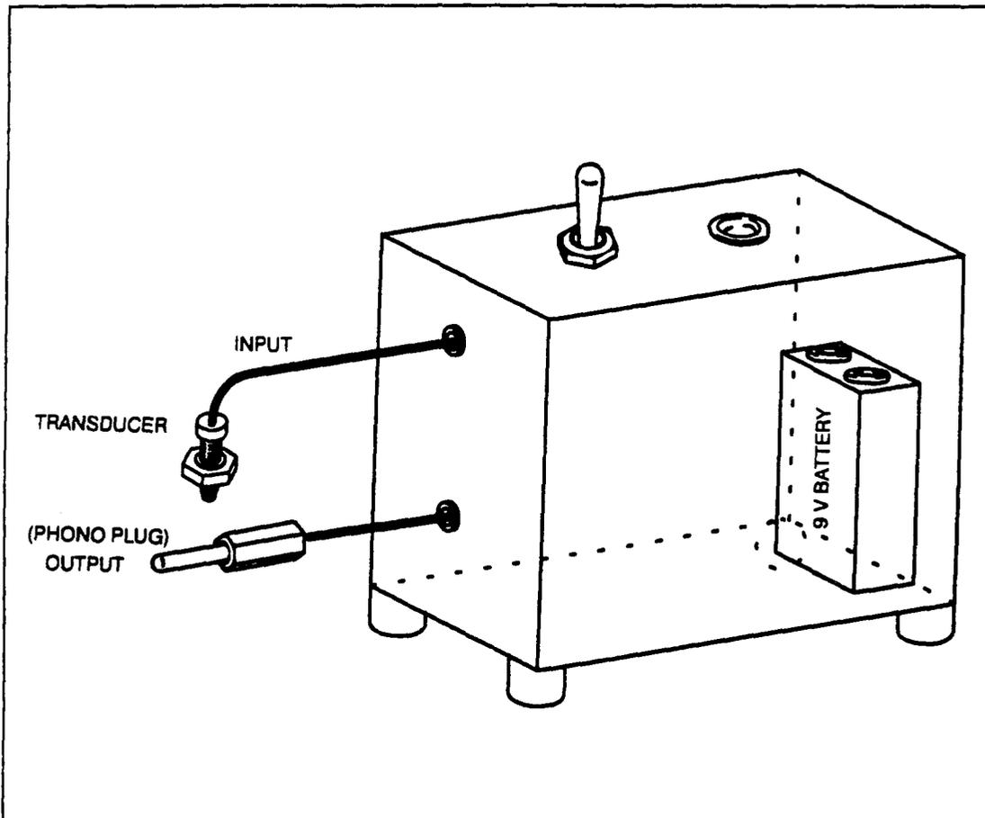
Figure 11 photo of hardware with the input and output shown.
