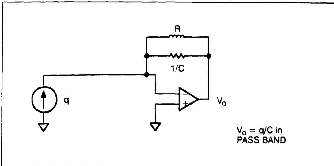
Figure 8 equivalent circuit representation for the charge amplifier with a charge generator as input.
