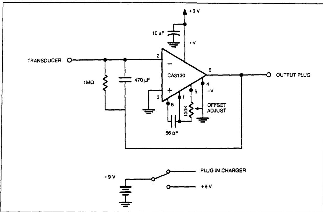
Figure 7 the CA3130 Operational Amplifier design
