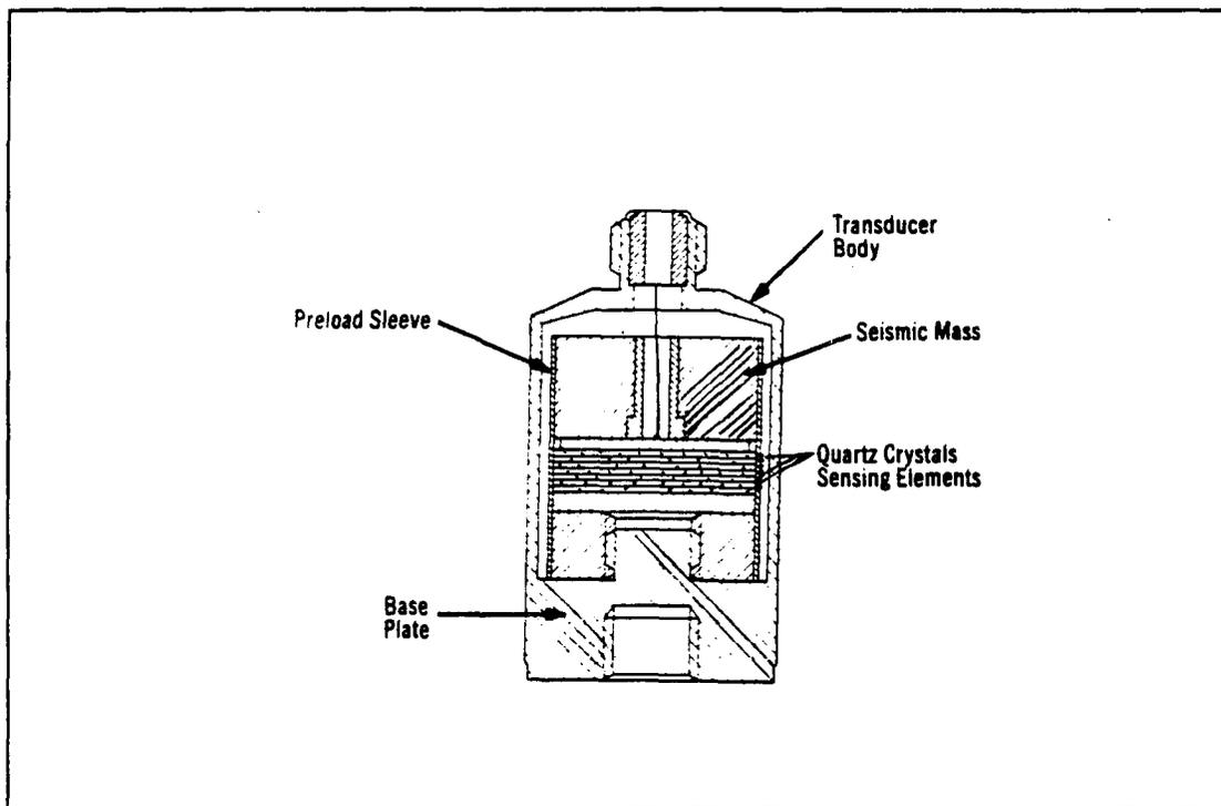
Figure 5 typical transducer (2).
