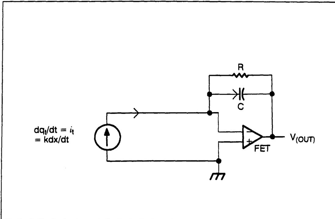
Figure 9 equivalent circuit based on current generator as input.
