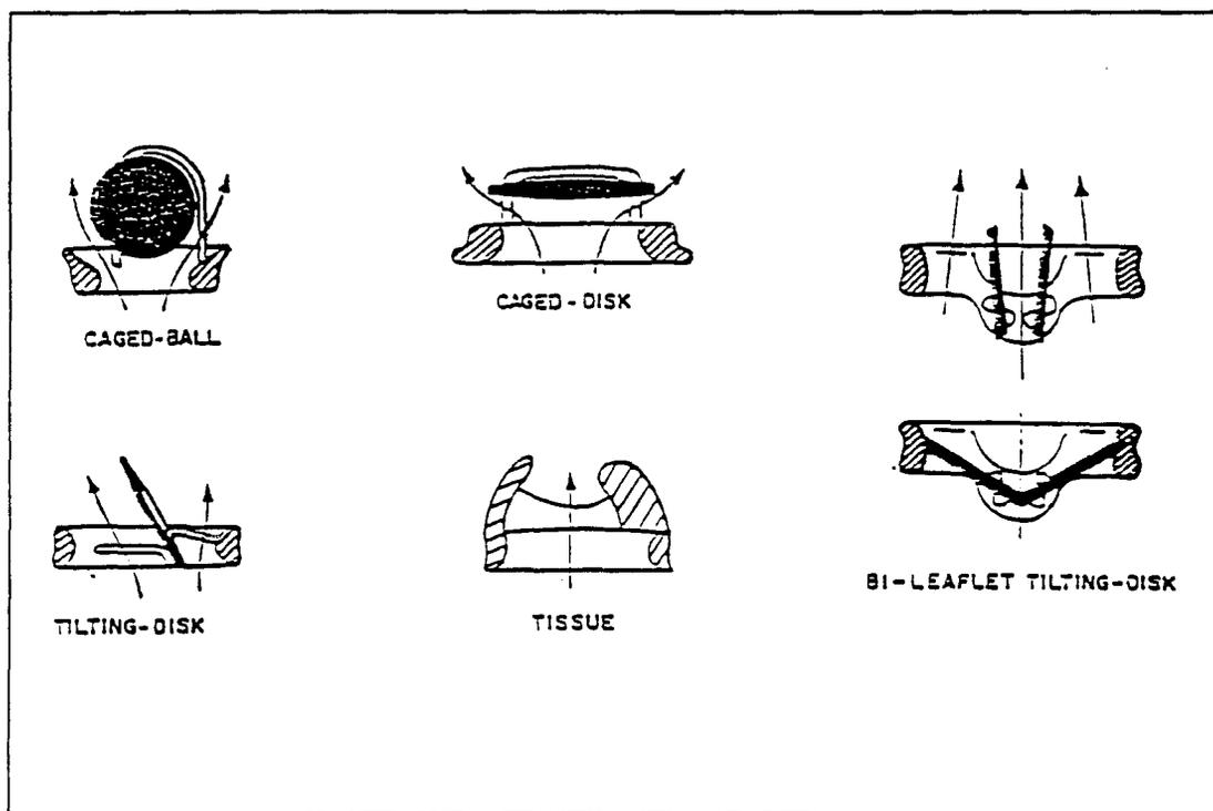
Figure 1 design and flow patterns of major categories of current prosthetic valves (1).
