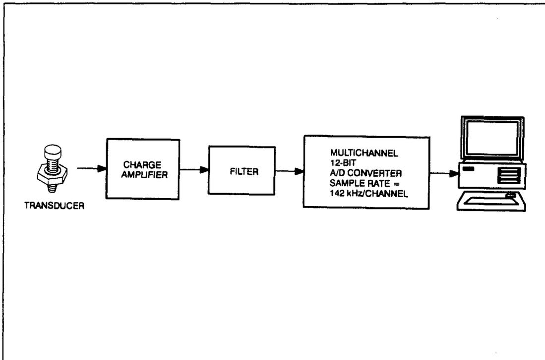
Figure 6 schematic of data acquisition system
