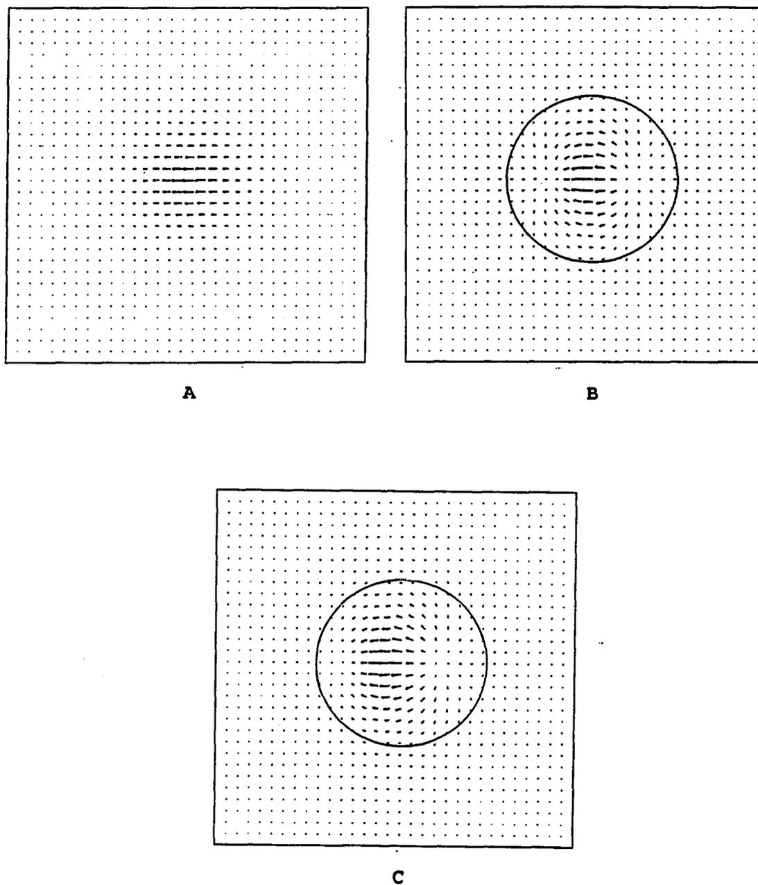
Figure 3.14: Plane  $x=8$  of the magnetic field generated by: A) the analytical solution to the problem in Fig. 3.13 B) the analytical solution to the problem in Fig. 3.12 C) the simulated solution to the problem in Fig. 3.12.
