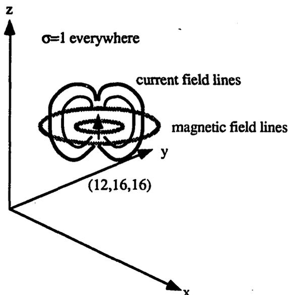
Figure 3.13: A vertical dipole at position (12,16,16) surrounded by an infinite space of uniform conductivity.
