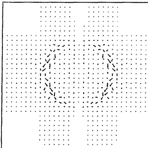
Figure 4.9: Plane  $x=16$  of the surface currents that generated the field in Fig. 4.8.
