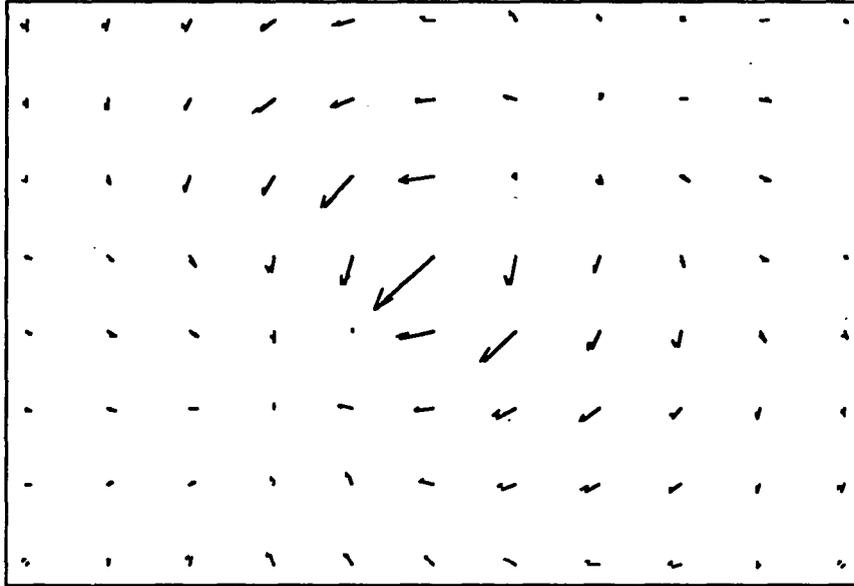
Figure (2.8): The current dipole return field, plane  $y=5$ .
