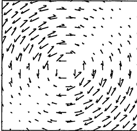
Figure (2.6): The real part of the tangential projection of the Fourier transform of the delta function, plane  $\eta=0$ .
