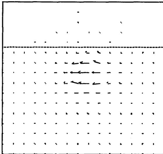
Figure 3.11: The magnetic field in plane  $y=6$ . Ideally, the field should equal zero above the plane  $z=10$ .
