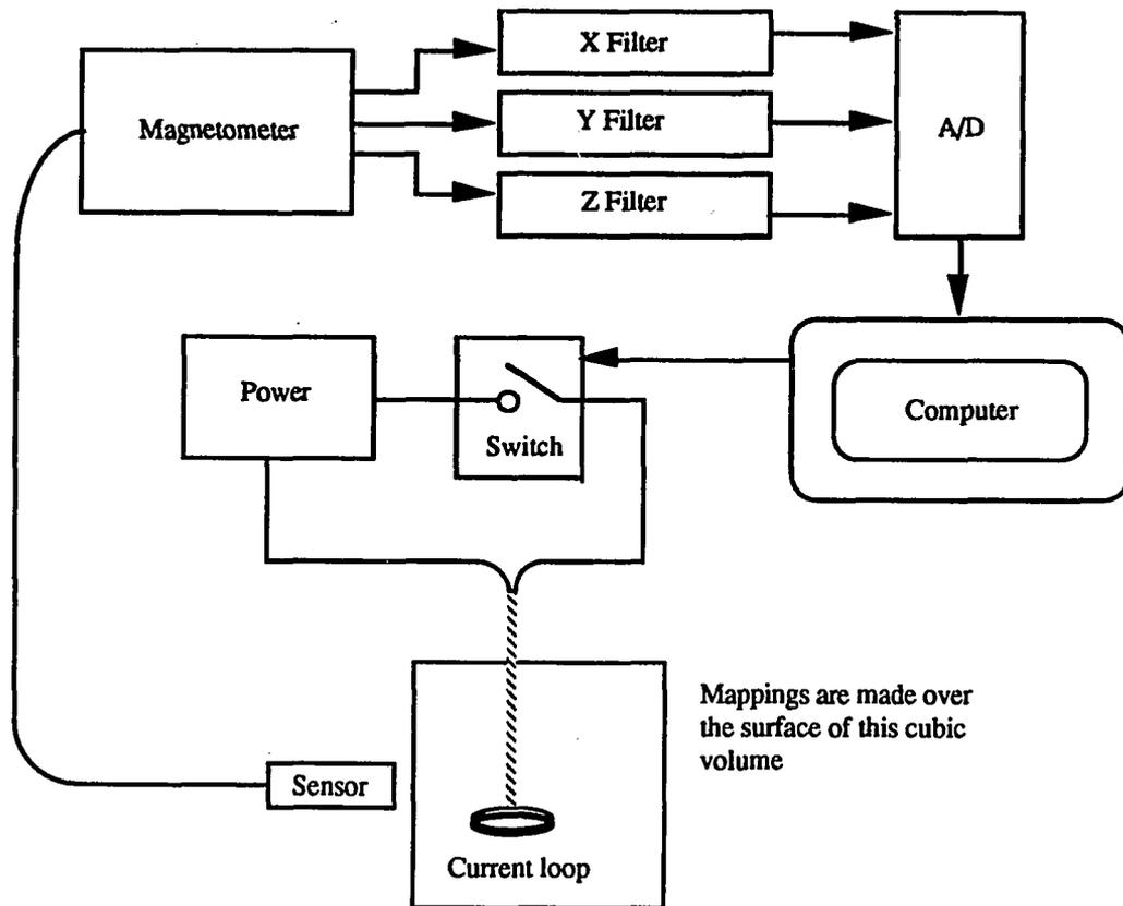
Figure 1.3: Schematic of the magnetic field mapping system
