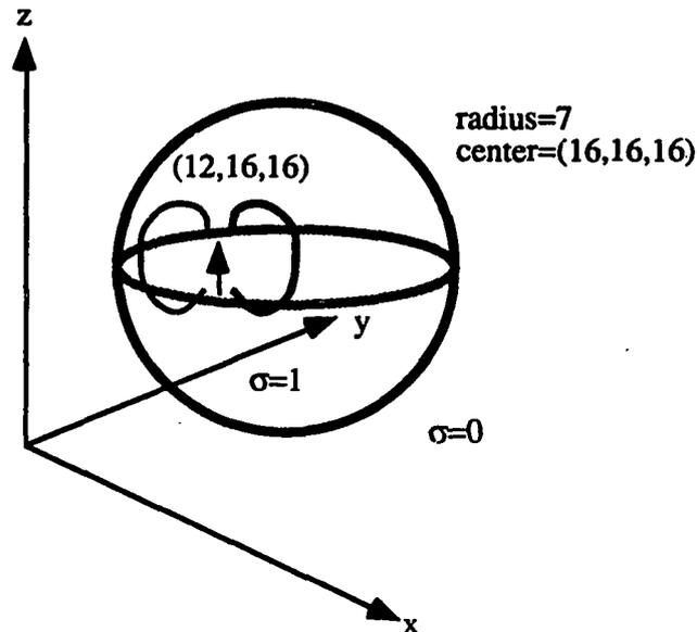
Figure 3.12: A vertical dipole in a sphere of uniform conductivity.
