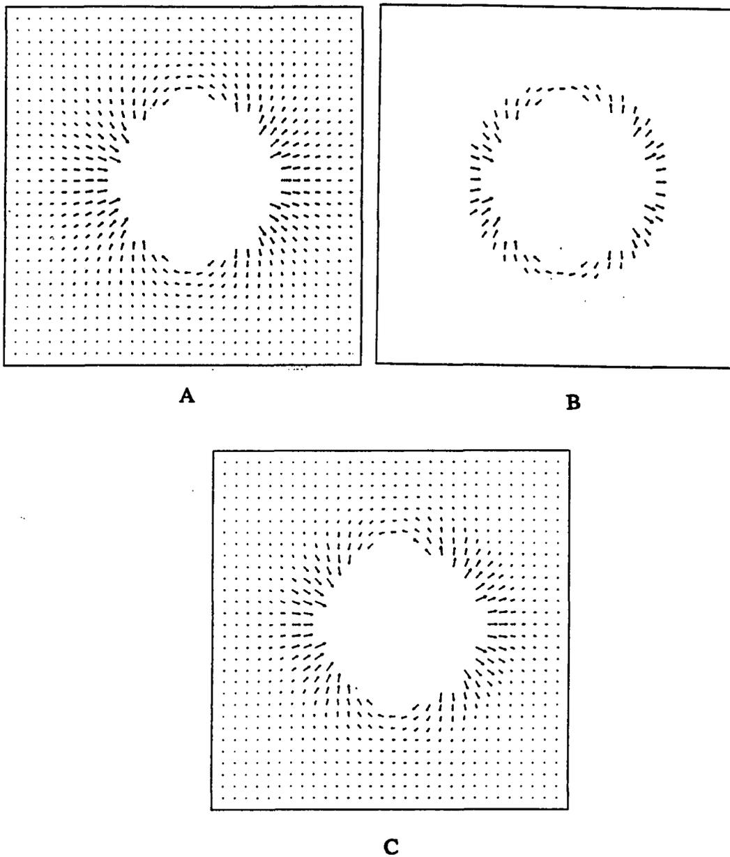
Figure 4.4: A) Analytic calculation of the magnetic field surrounding the sphere in Fig. 3.10 B) The surface values of field A C) Extrapolation of the surface values using Fourier projection. All three figures show plane  $y=16$ .
