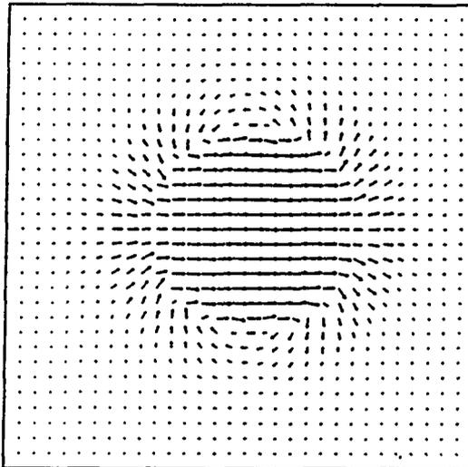
Figure 4.8: Plane  $y=16$  of the magnetic field produced by a Fourier tangential iteration on the field in Fig. 4.4 A).
