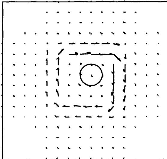
Figure 4.6: Plane  $z=6$  of the current field that generates the magnetic field in Fig. 4.5. The circle represents the current that generated the original field in Fig. 4.2.
