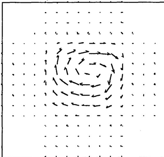
Figure 4.7: Plane  $z=10$ , the currents on the top surface of the cube.
