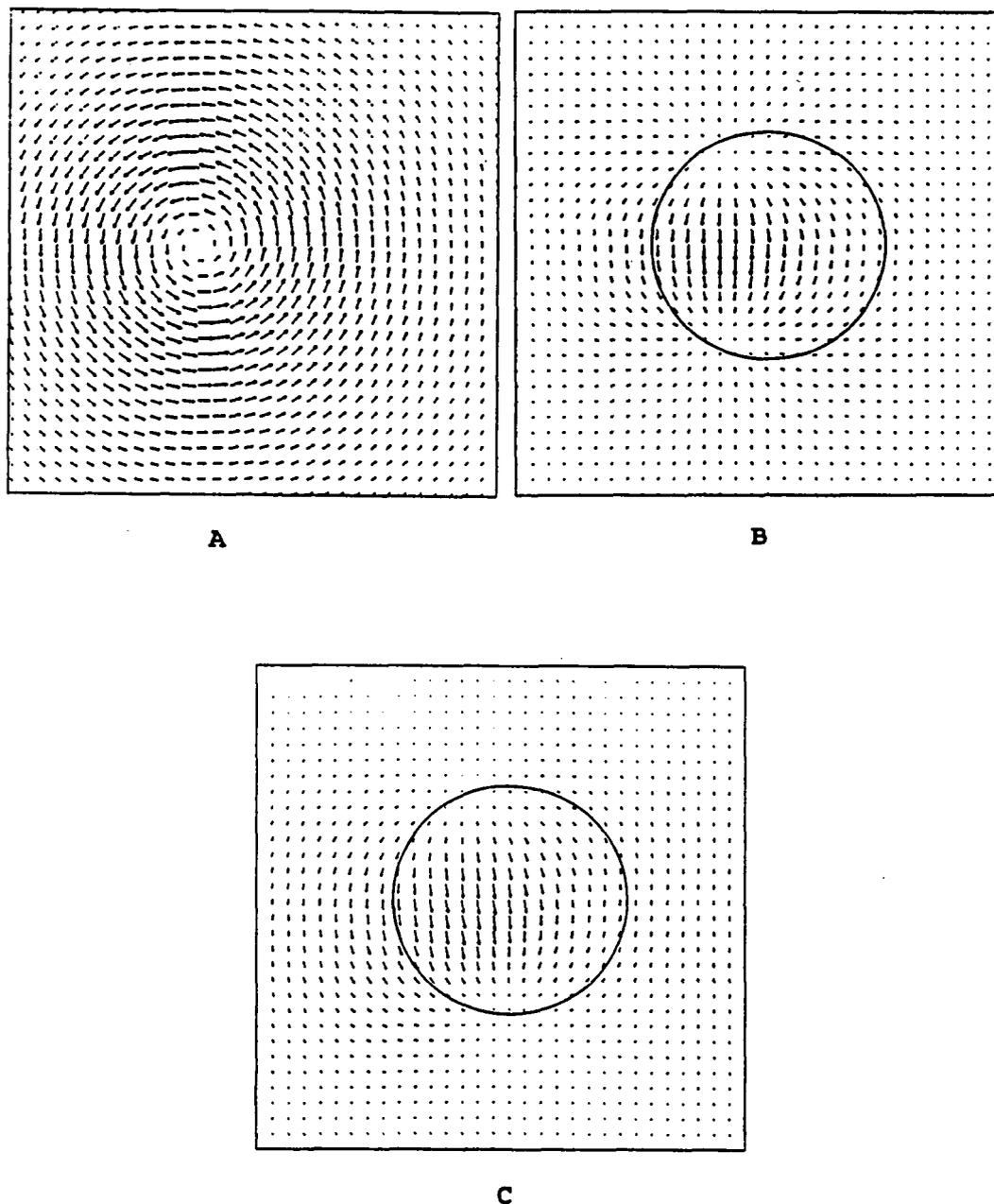
Figure 3.16: Plane  $z=8$  of the magnetic field generated by: A) the analytical solution to the problem in Fig. 3.13 B) the analytical solution to the problem in Fig. 3.12 C) the simulated solution to the problem in Fig. 3.12.
