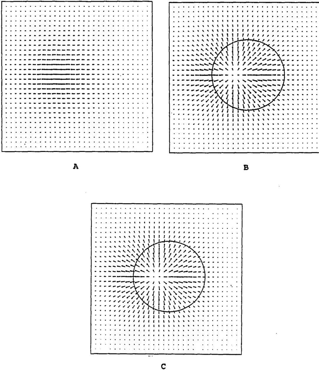
Figure 3.15: Plane  $y=24$  of the magnetic field generated by: A) the analytical solution to the problem in Fig. 3.13 B) the analytical solution to the problem in Fig. 3.12 C) the simulated solution to the problem in Fig. 3.12.
