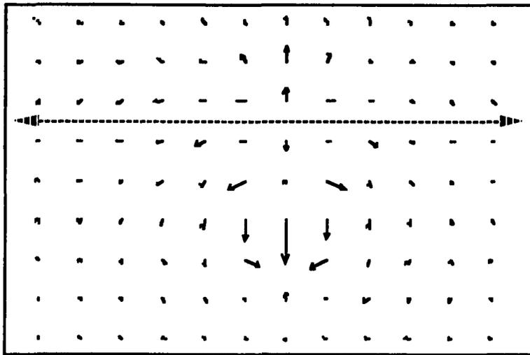
Figure 3.8: The electric field in plane  $y=10$ . The dotted line indicates the interface between zero and non-zero conductivity.
