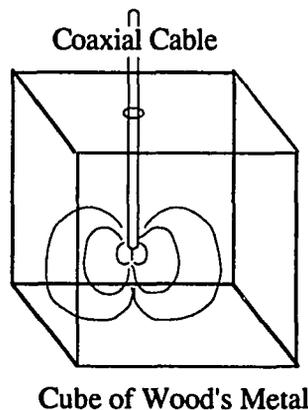
Figure 1.2: Current dipole phantom source
