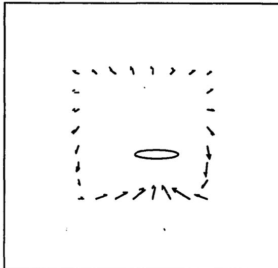
Figure 4.2: Plane  $y=8$  of the surface magnetic data collected from the source in Fig. 4.1. Plane  $y=8$  cuts through the center of the current loop shown here as an oval. (From this perspective it should actually look like a line segment).
