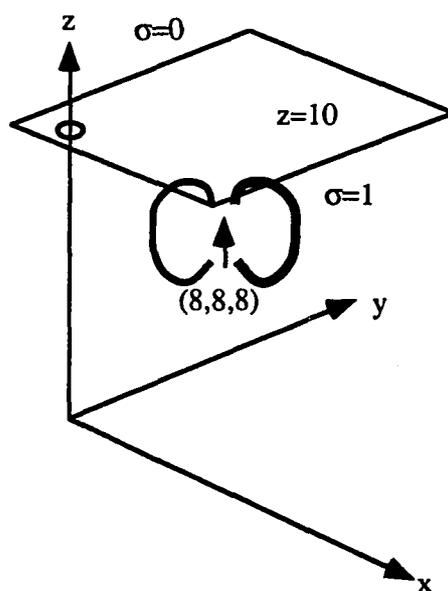
Figure 3.7: A vertical dipole at position (8,8,8). The conductivity is zero above the plane  $z=10$  and one below.
