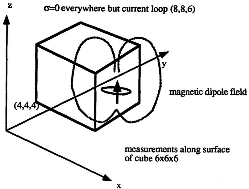
Figure 4.1: A current loop phantom source generating a magnetic dipole field that was mapped over the surface of the cube.
