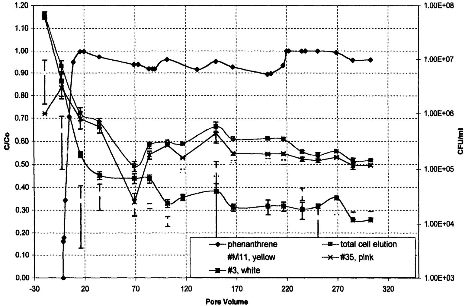
Figure 4.10 Biodegradation and cell elution in a three-species column system. *Actinobacter junii* (3), *Pseudomonas oleavoreans* (M11), *Methylobacterium* sp. (35).
