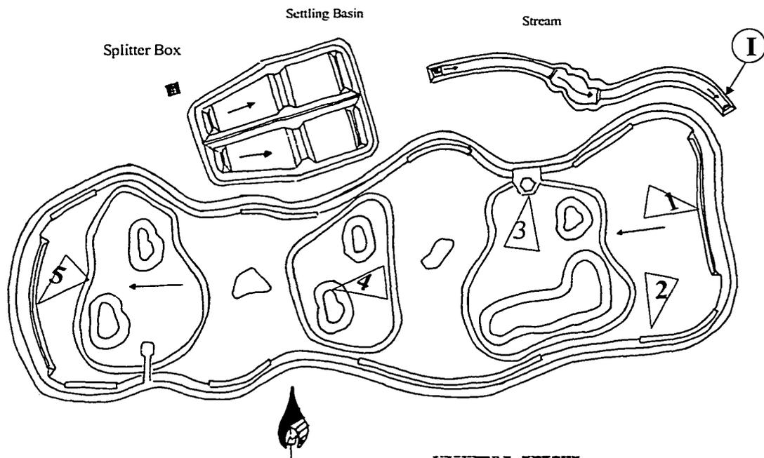
**Figure 1. Schematic representation of the east polishing basin showing the injection (I) and sampling sites at the inlet (1), lysimeter area (2), first (3) and second (4) open water zones, and outlet (5) of the system.**
