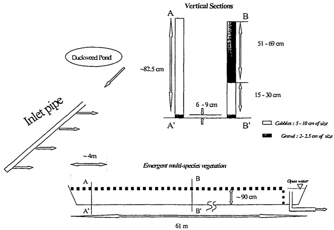
Figure 1. Schematic representation of the vegetated-gravel bed where the tracer study was conducted. The vertical sections (A-A' and B-B') show gravel and cobble layers stratification in the wetland. The influent water is distributed along the inlet by the inlet pipe.
