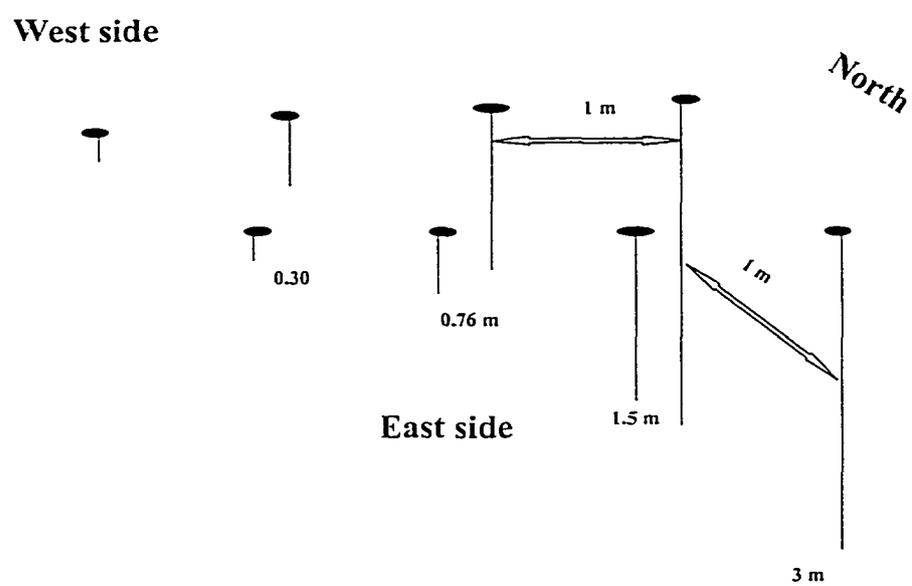
**Figure 2. Schematic representation of the East and West lysimeter arrays depicting installation depths (0.3, 0.76, 1.5, and 3 m) and separation between adjacent lysimeters (1 m).**
