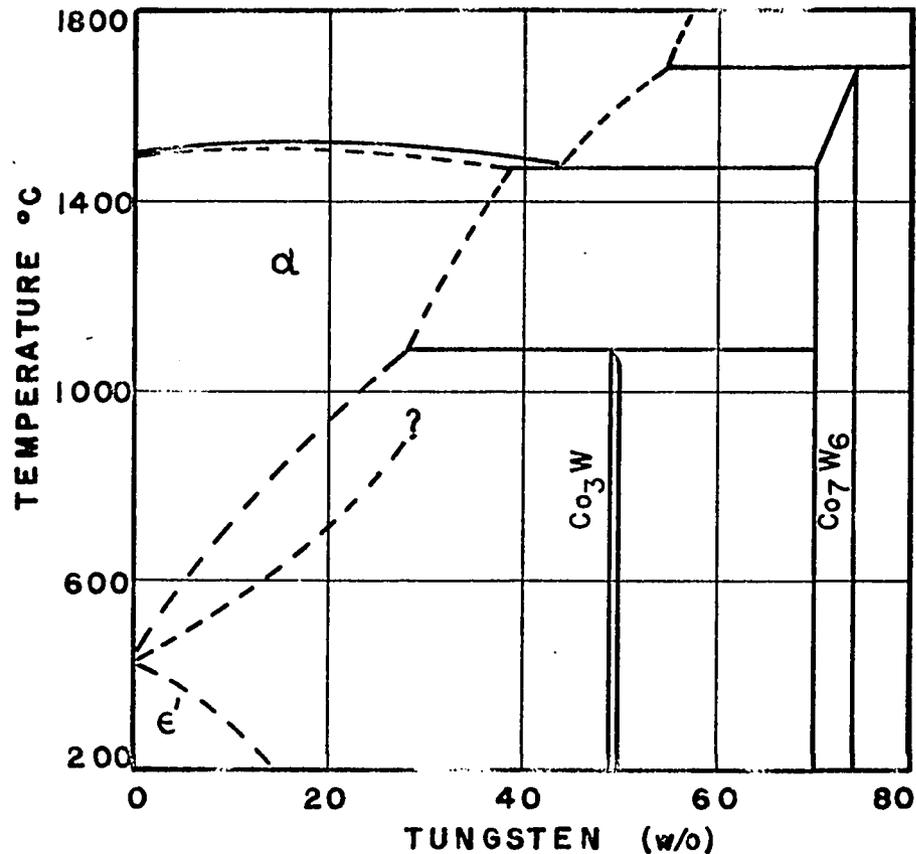
Fig. 6. The Co-W Phase Diagram
