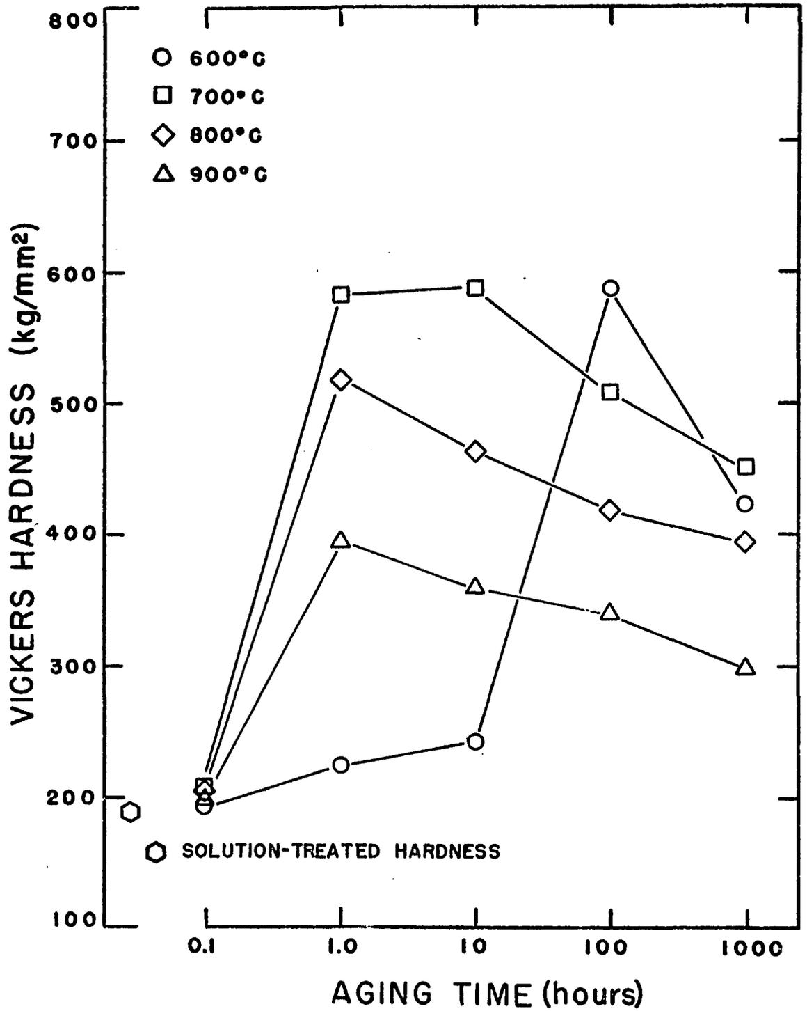
Fig. 20. Aging Curves for Co-4Al-6Ti
