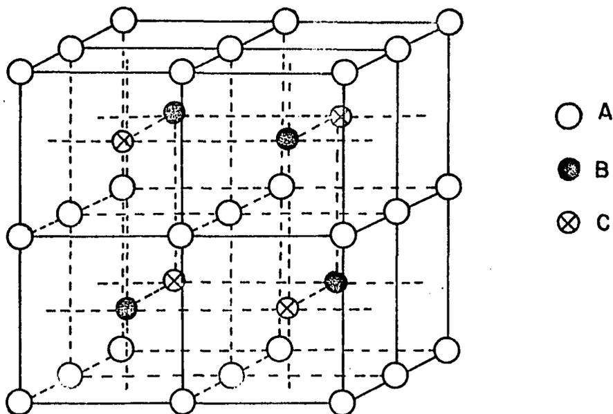
Fig. 8. Body-centered Cubic Model
