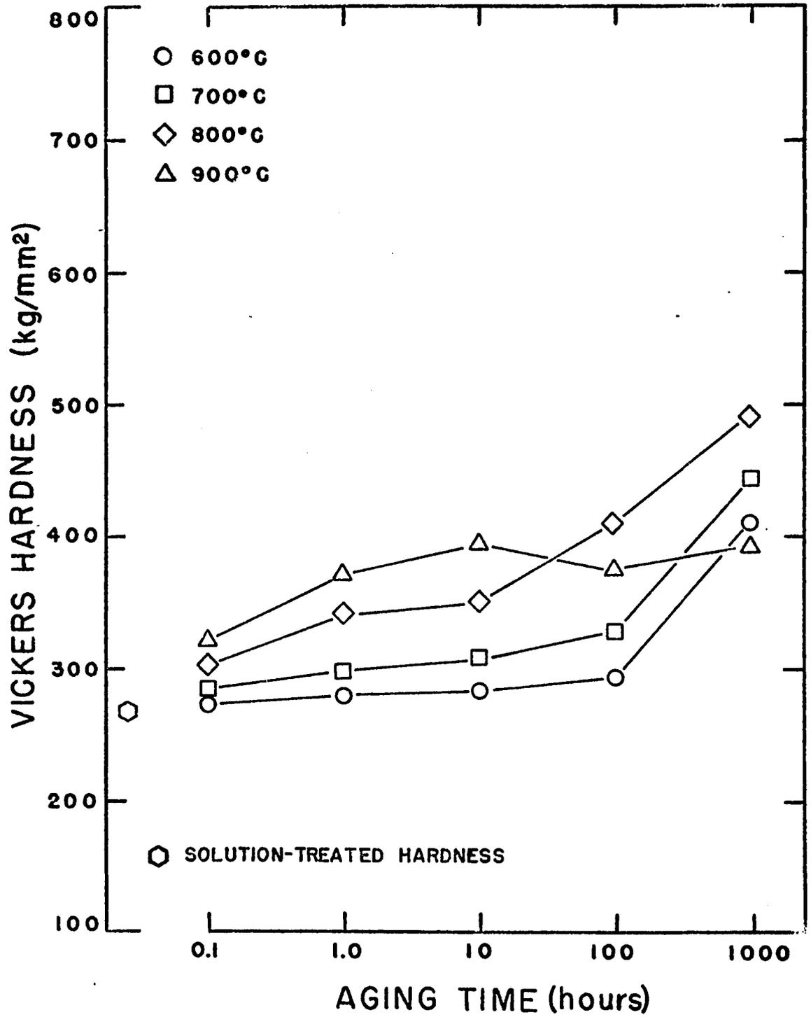
Fig. 27. Aging Curves for Co-4Al-25W
