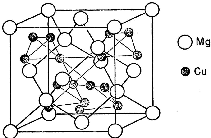
Fig. 7. The MgCu<sub>2</sub> Structure
