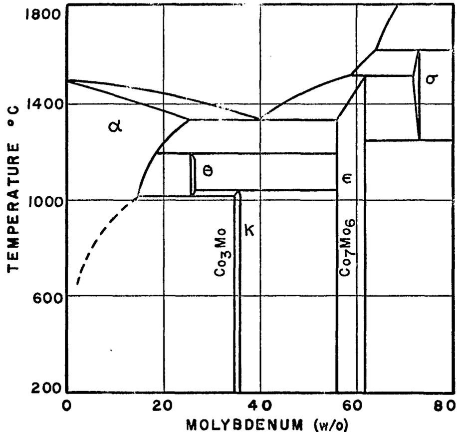
Fig. 5. The Co-Mo Phase Diagram
