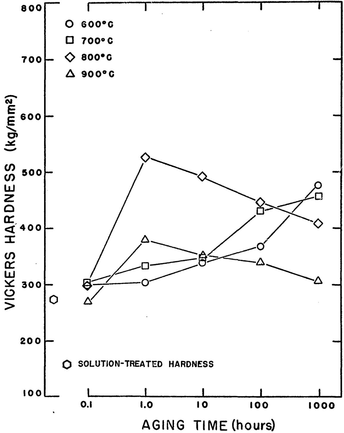
Fig. 21. Aging Curves for Co-4Al-9Ti
