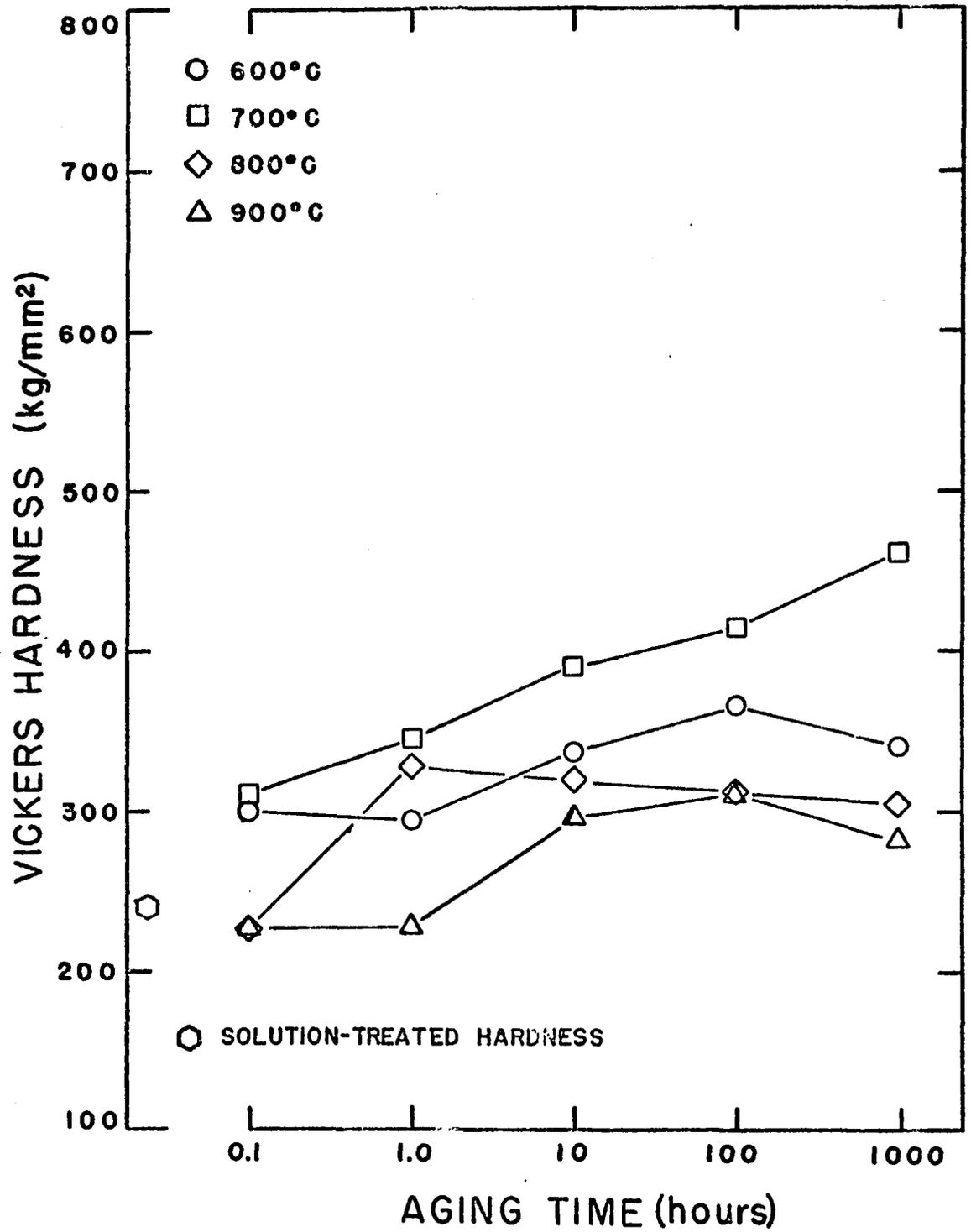
Fig. 11. Aging Curves for Co-4Al-5Nb
