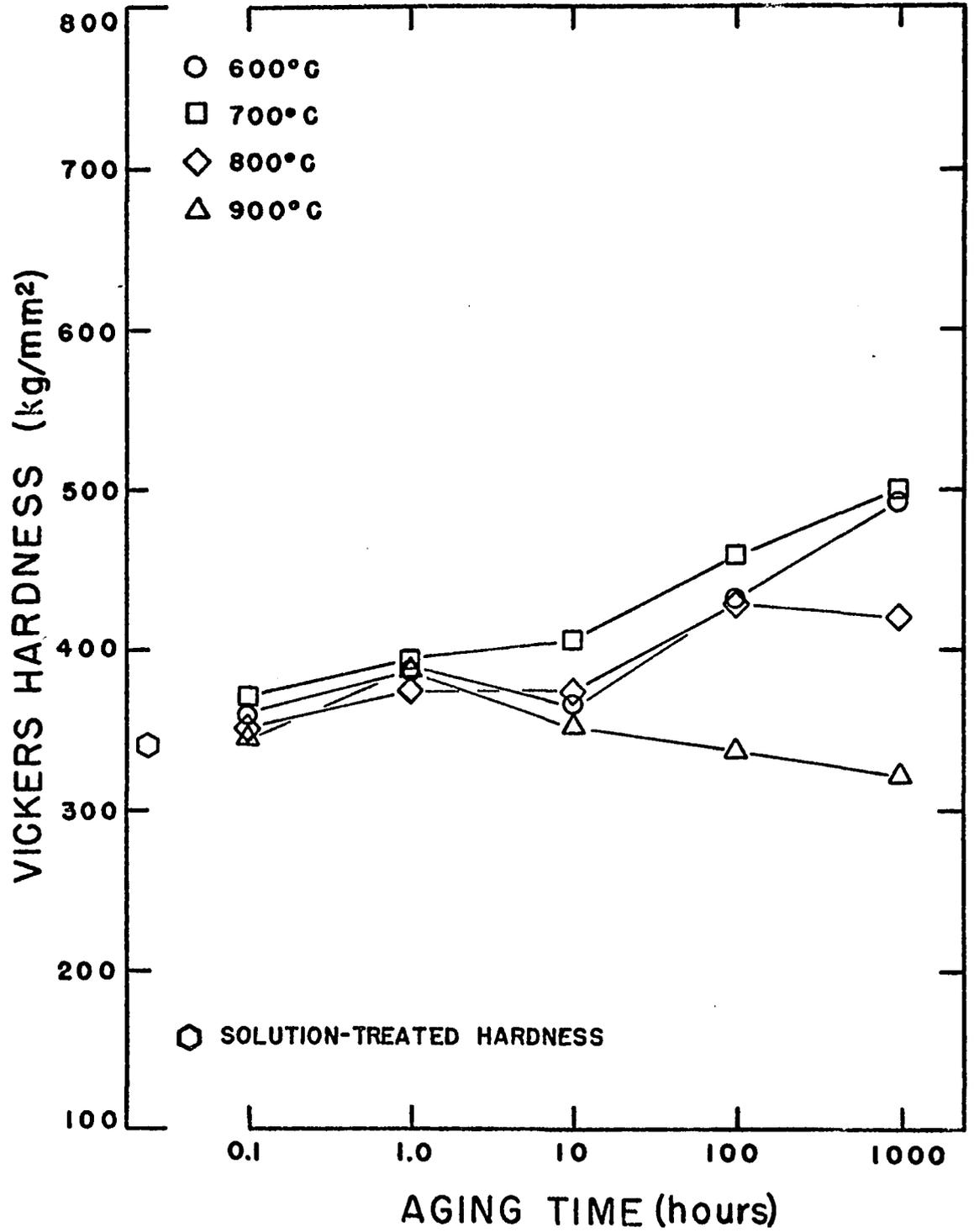
Fig. 22. Aging Curves for Co-4Al-12Ti
