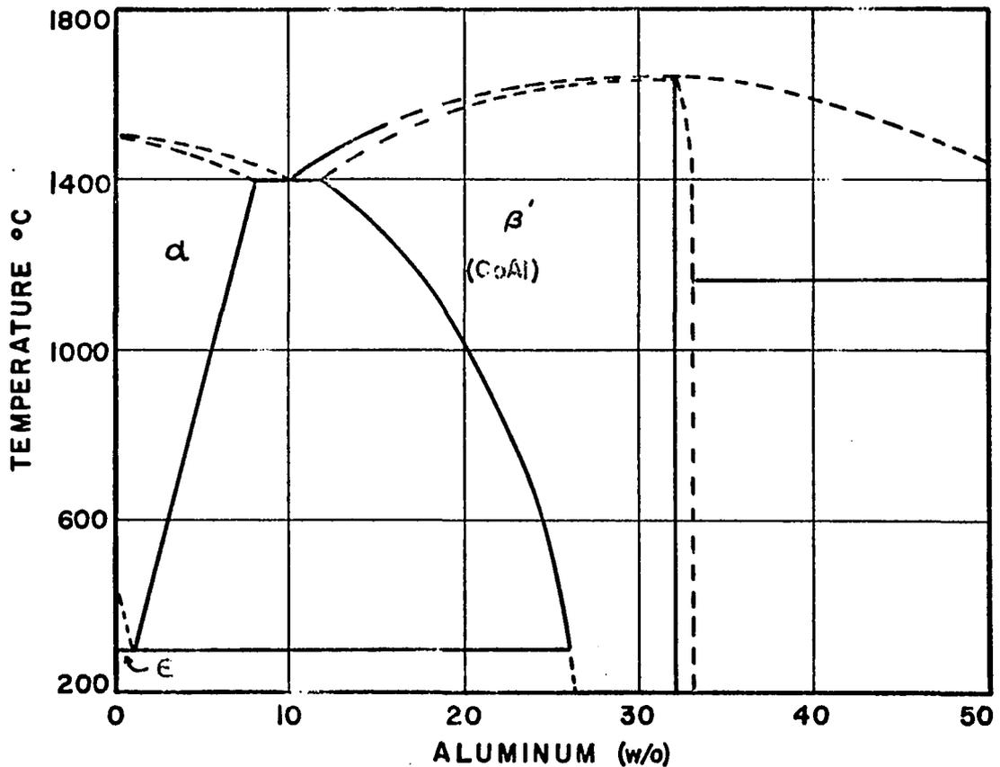
Fig. 1. The Co-Al Phase Diagram
