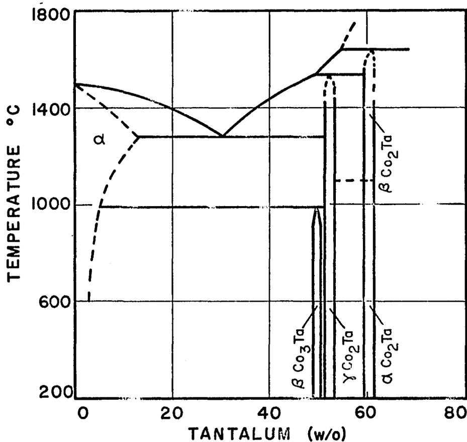
Fig. 3. The Co-Ta Phase Diagram
