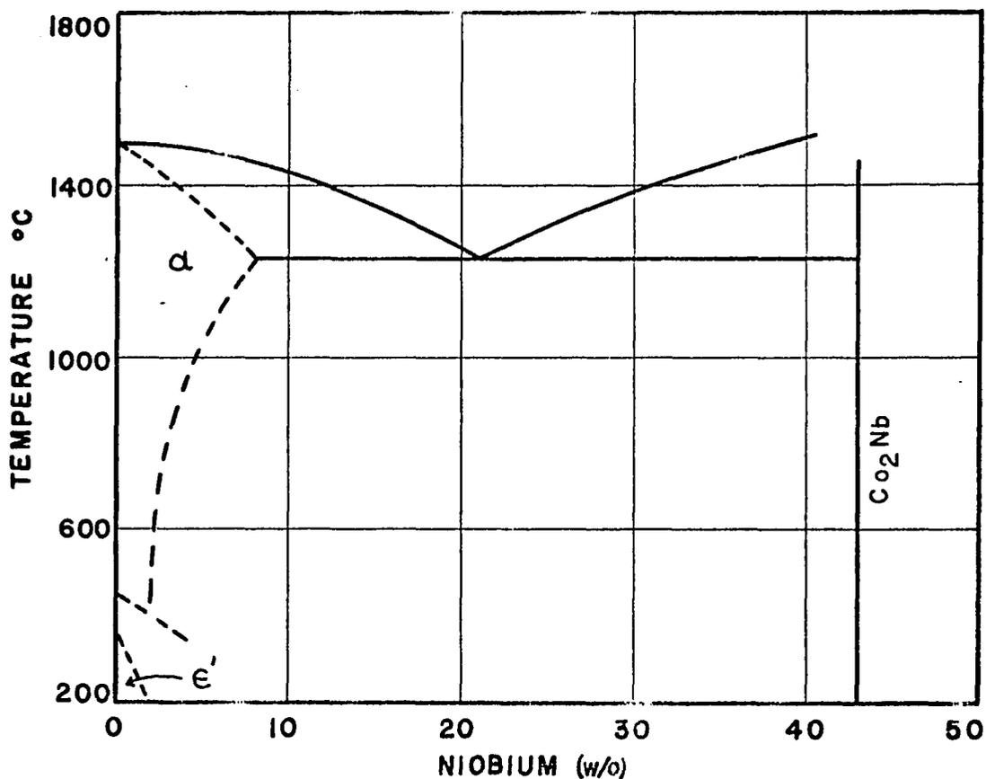
Fig. 2. The Co-Nb Phase Diagram
