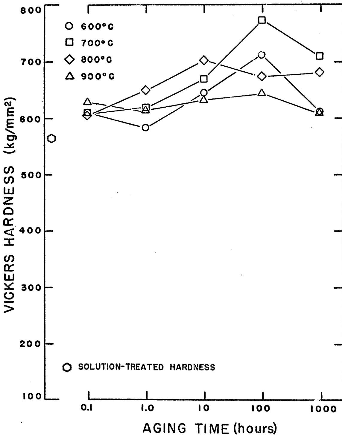
Fig. 14. Aging Curves for Co-4Al-20Nb
