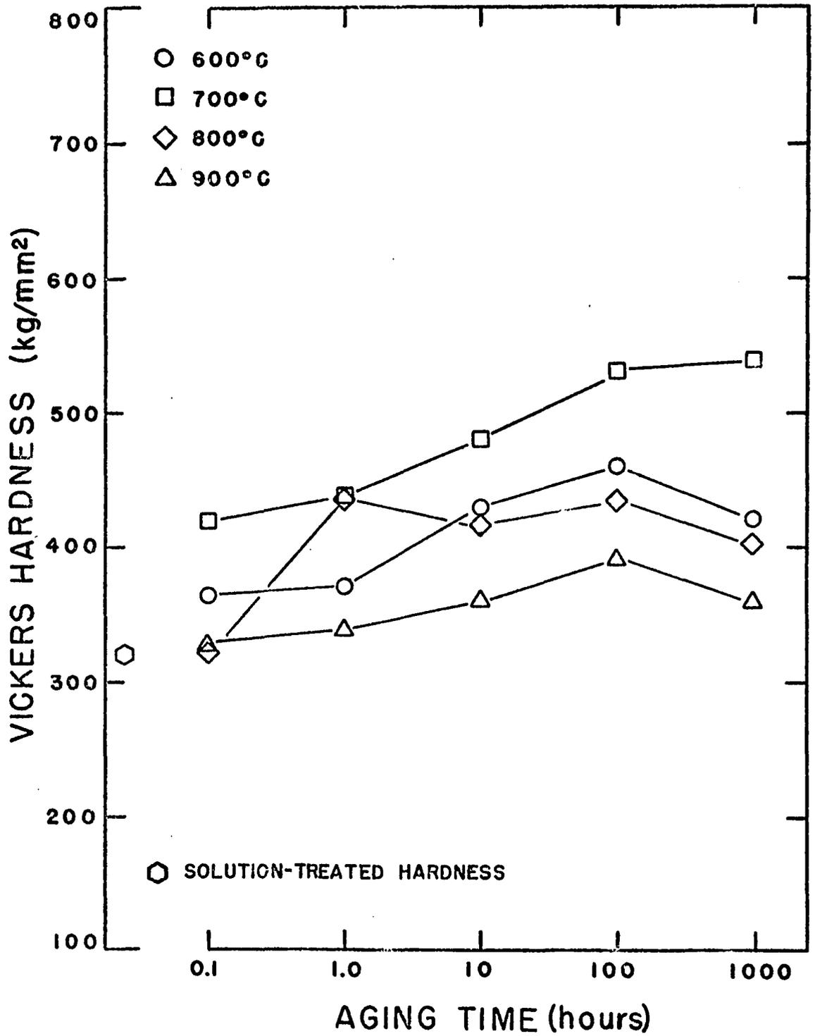
Fig. 12. Aging Curves for Co-4Al-10Nb
