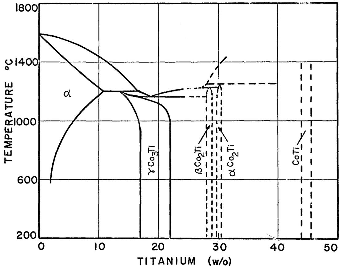
Fig. 4. The Co-Ti Phase Diagram
