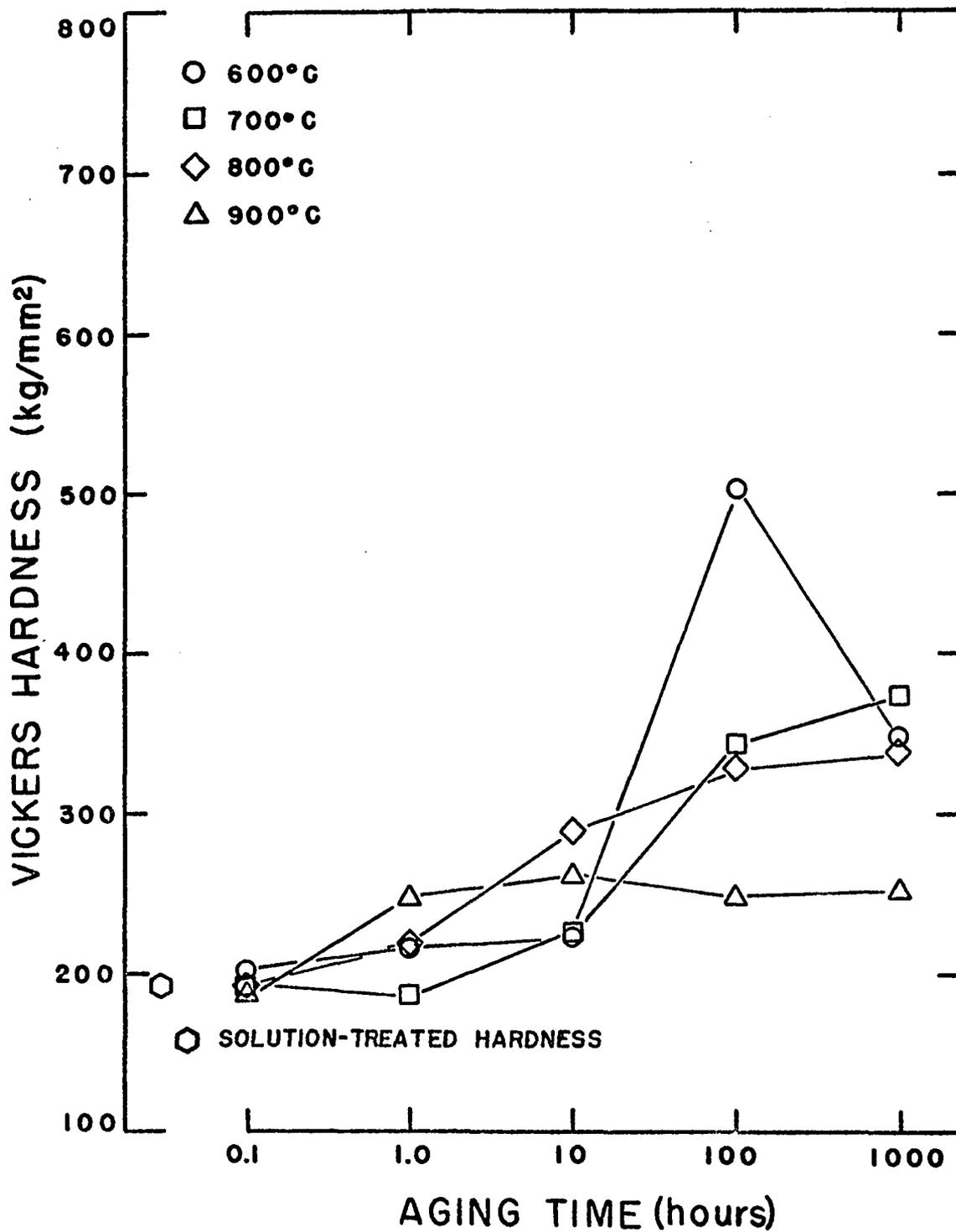
Fig. 19. Aging Curves for Co-4Al-3Ti
