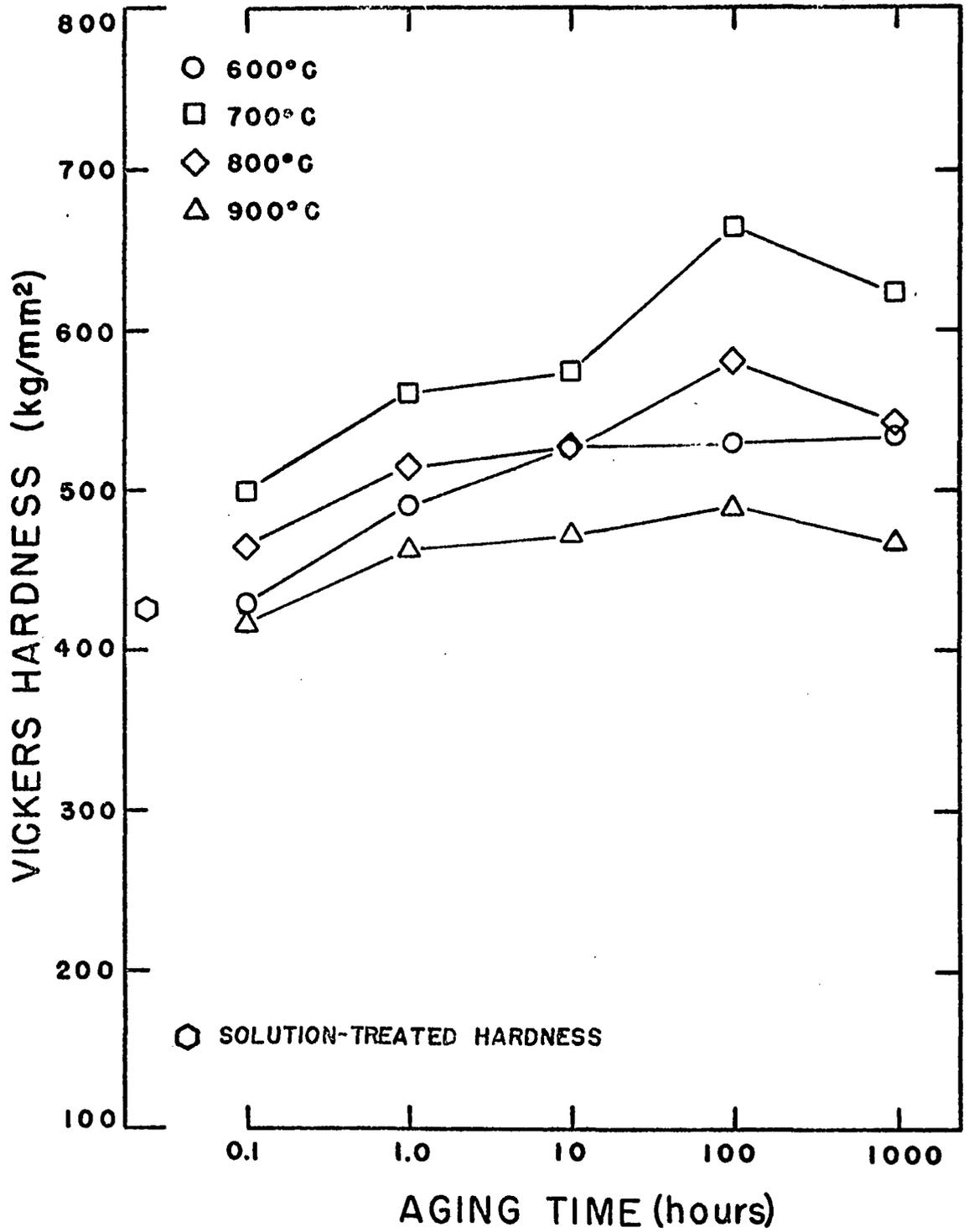
Fig. 13. Aging Curves for Co-4Al-15Nb
