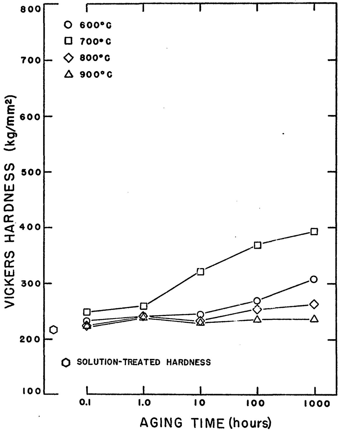
Fig. 26. Aging Curves for Co-4Al-10W
