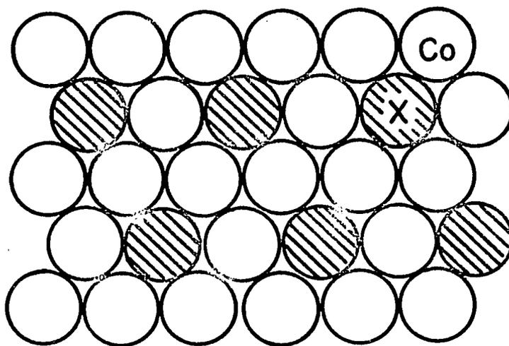
Fig. 9. Close-packed Triangular Ordering
