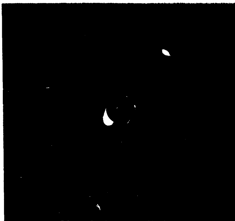
Fig. 44. Pinhole Back-Reflection Diffraction Pattern of a Tenzalloy Test Bar with a Feather Crystal Structure.
