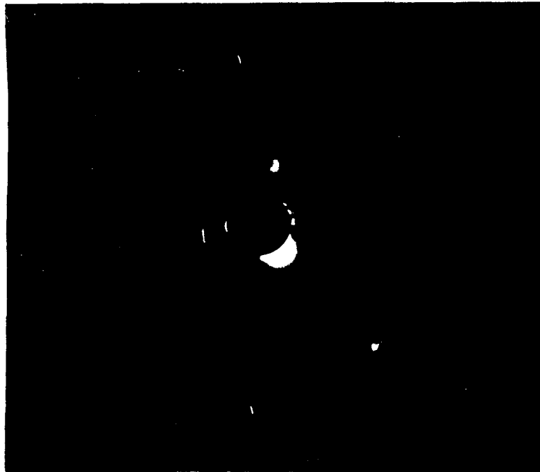
Fig. 43. Pinhole Back-Reflection Diffraction Pattern of a Tenzalloy Test Bar with a Columnar Crystal Structure.
