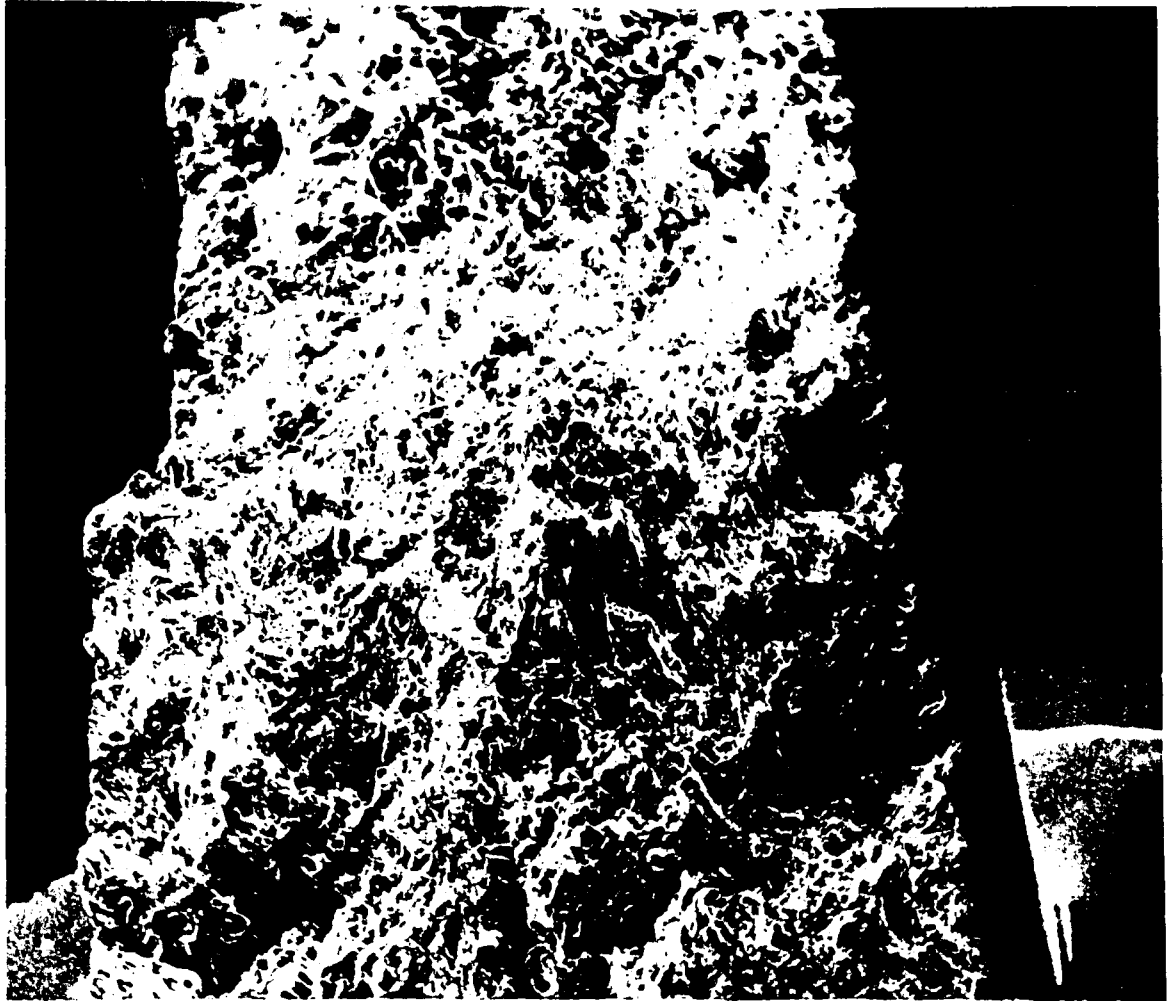
Fig. 47a. Scanning Electron Micrograph of the Fracture Surface of a Tenzalloy Test Bar which had a Random Grain Structure, 25X.
