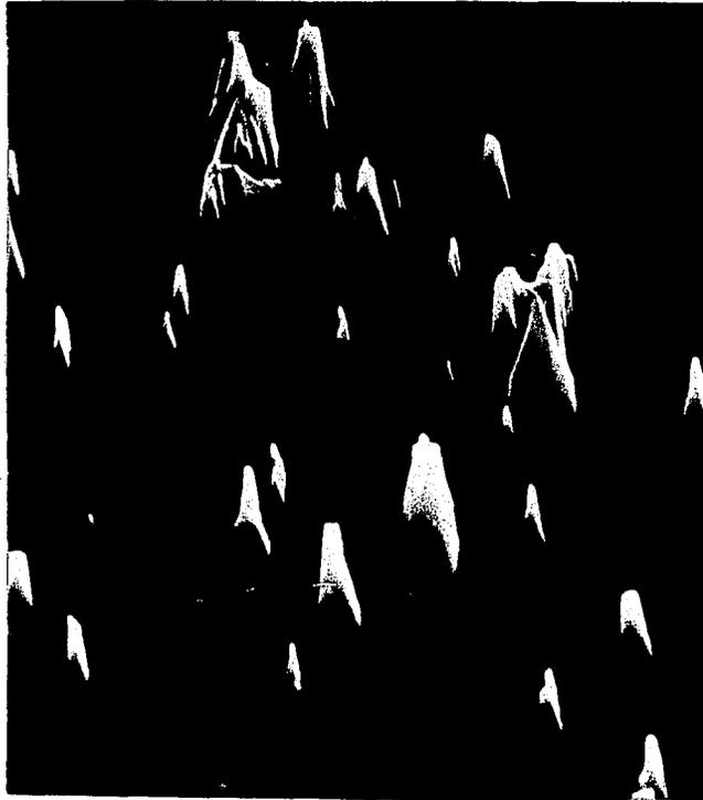
Fig. 64. SEM Micrograph, Fused Silica, 5 KeV, Xenon at 45°, Magnification 3,000X.
