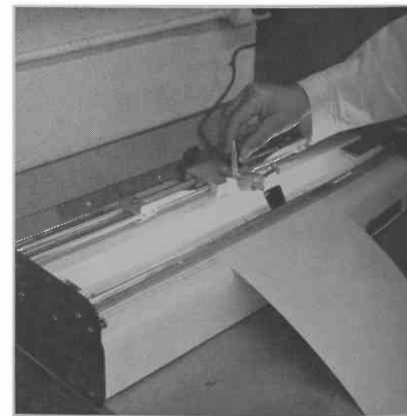
FIGURE 2 — Chromatogram stripper used for the uniform application of sample solutions in micro-quantities.
