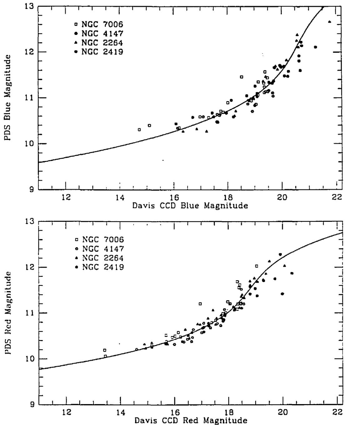
Figure 5. Calibration curves for PDS to CCD magnitude conversion for four red and blue standard fields from separate POSS plates. The separate symbols indicated by the legend show each star cluster plotted and the best fit curve to the data. Calibration curve parameters are given in Table 1.
