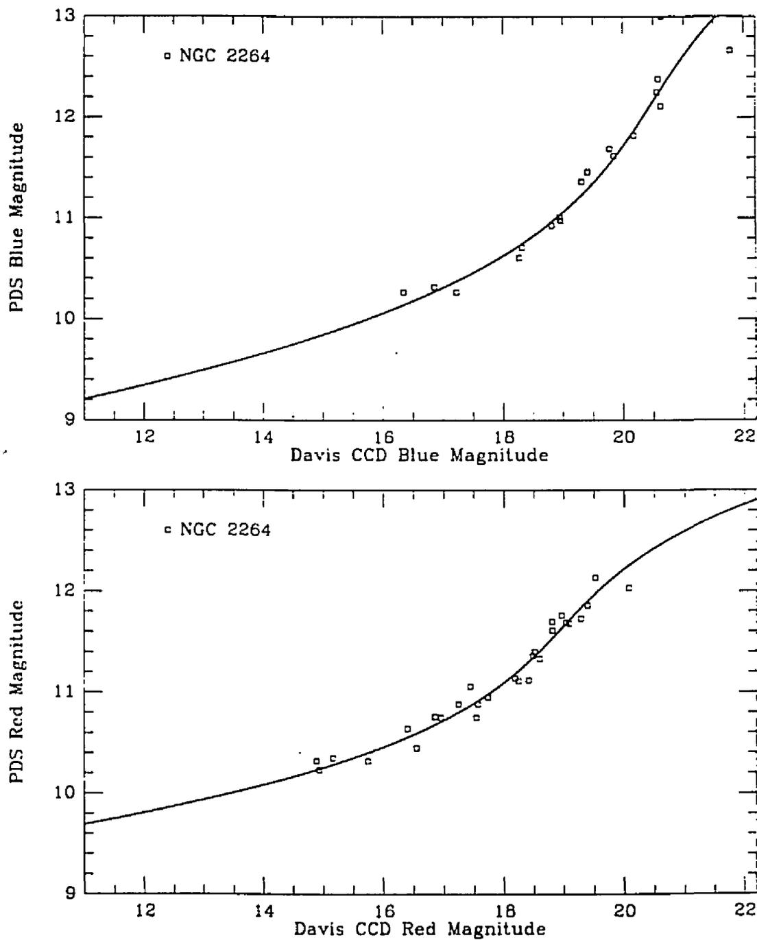
Figure 6. Calibration curves for PDS to CCD magnitude conversion for NGC2264 cluster data from a single POSS plate for each color. Note that the scatter in the fit in Figure 5 is greatly reduced here by using data from one plate. The calibration curve parameters are given in Table 1.
